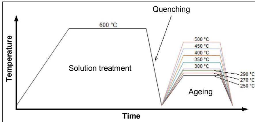
**Figure 1** Heat treatment of NiTi wires
