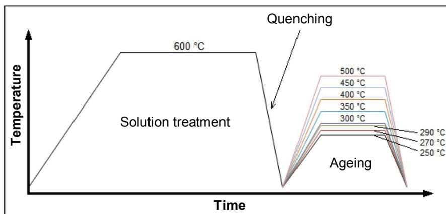
**Figure 1** Heat treatment of NiTi wires
