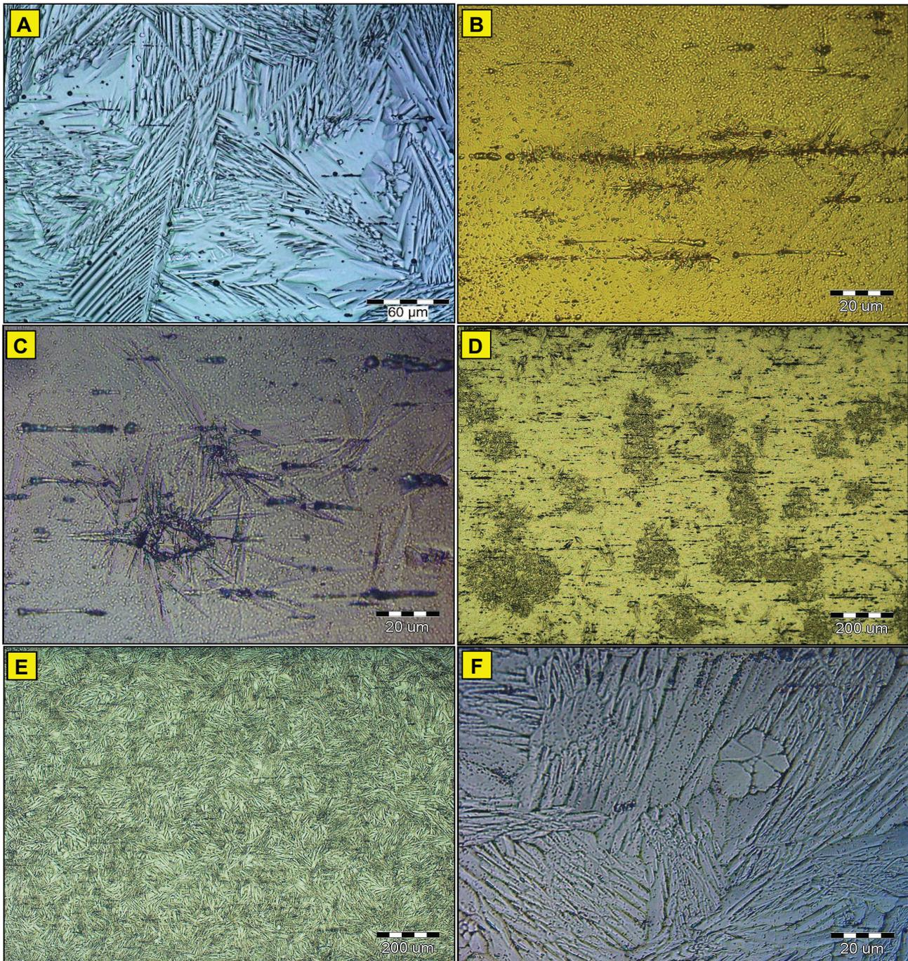
**Figure 2** Microstructure of NiTi wires after various conditions of heat treatment
