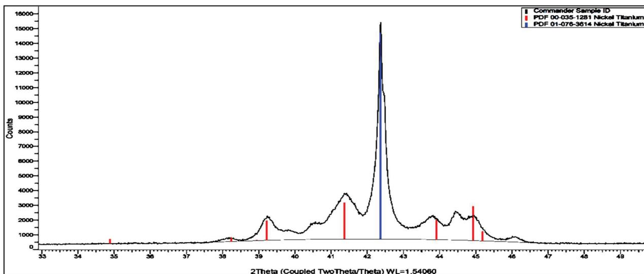
**Figure 4** X-ray diffraction spectrum of TiNi alloy (wire diameter 1 mm, initial material)
