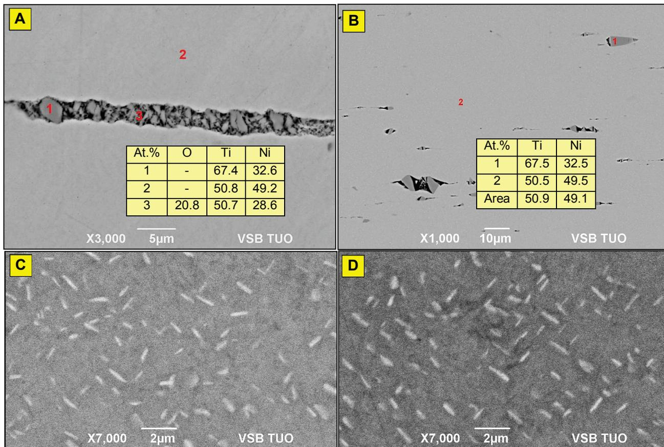
**Figure 3** SEM/EDX analysis of NiTi wire after various heat treatment
