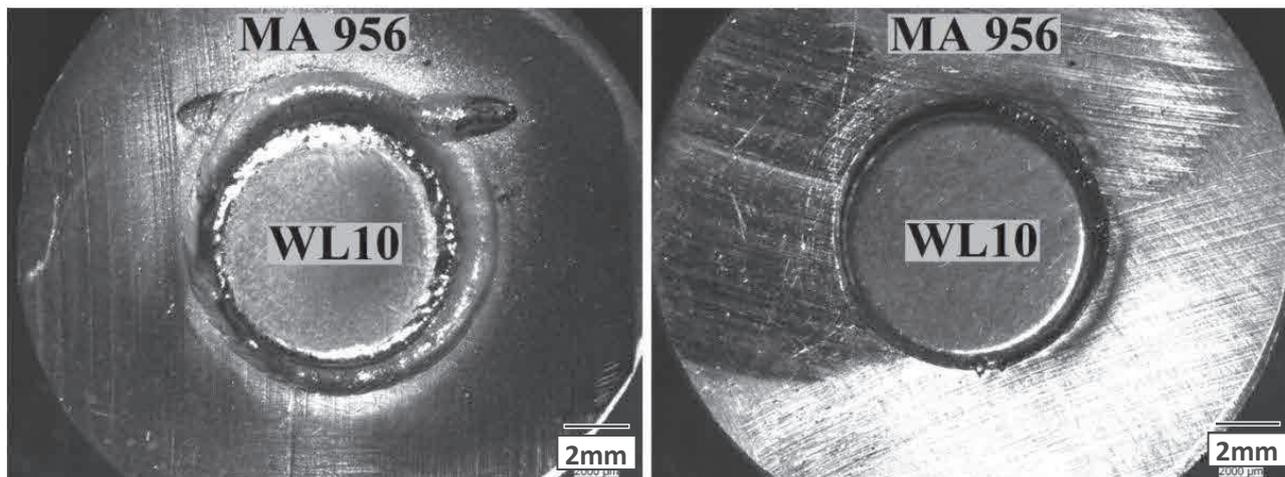
**Figure 1** Typical view of the samples from the top (left) and bottom (right) of the joint
