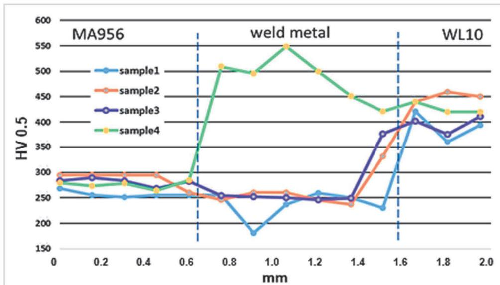
**Figure 3** Microhardness of the weld area, weld metal noted by the vertical lines
