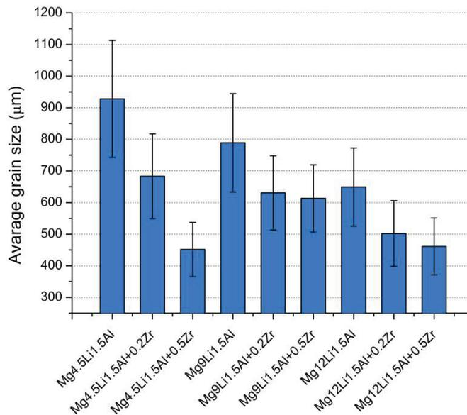
**Figure 2** Variation of grain size of investigated Mg-Li-Al alloys with the addition levels of Zr
