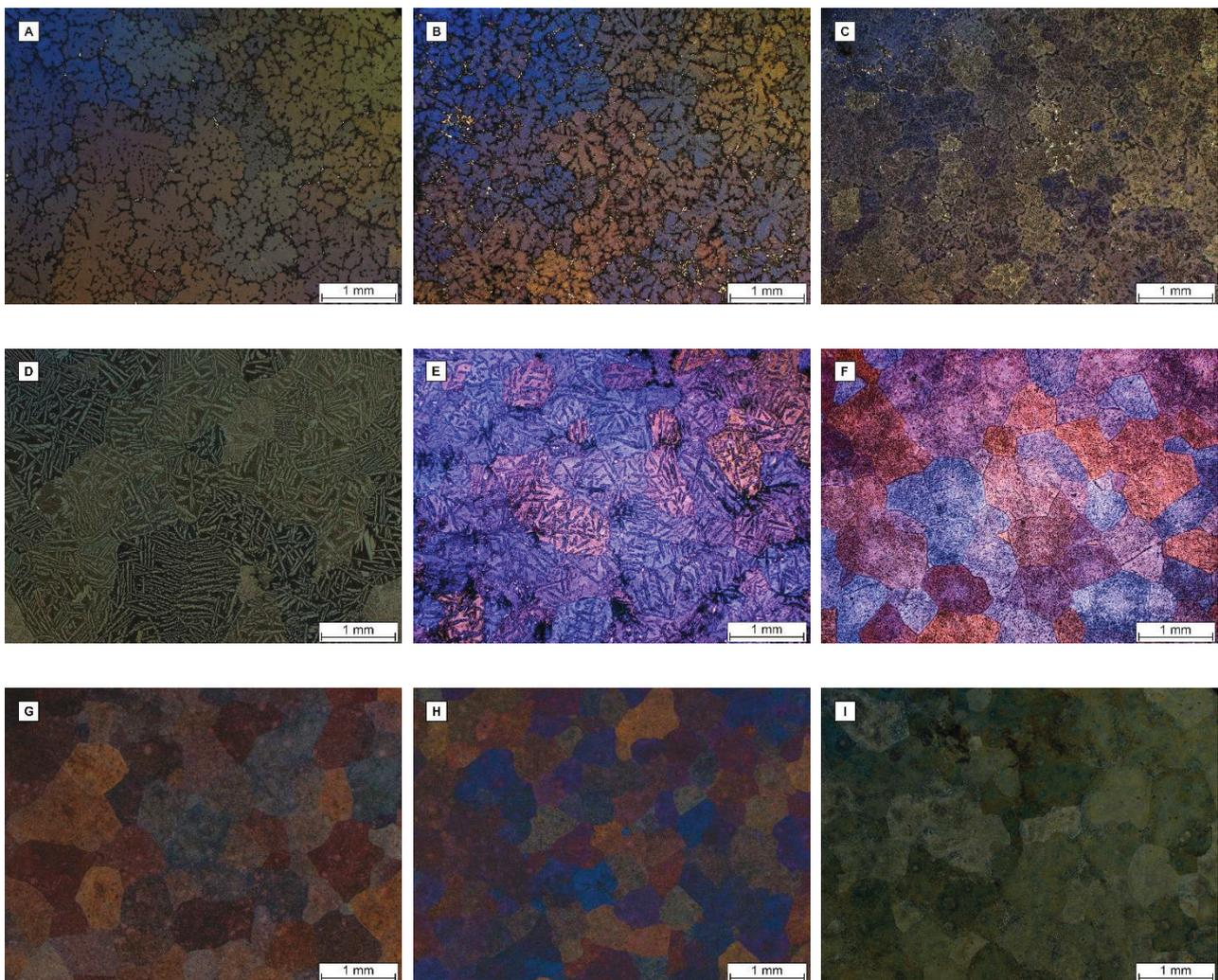
**Figure 1** Optical micrographs showing the grain size of Mg-Li-Al base alloy at various level of Li and Zr (in wt.%): a) Mg-4.5Li-1.5Al, b) Mg-4.5Li-1.5Al+0.2Zr, c) Mg-4.5Li-1.5Al+0.5Zr, d) Mg-9Li-1.5Al, e) Mg-9Li-1.5Al+0.2Zr, f) Mg-9Li-1.5Al+0.5Zr, g) Mg-12Li-1.5Al, h) Mg-12Li-1.5Al+0.2Zr, i) Mg-12Li-1.5Al+0.5Zr, Nomarsky contrast
