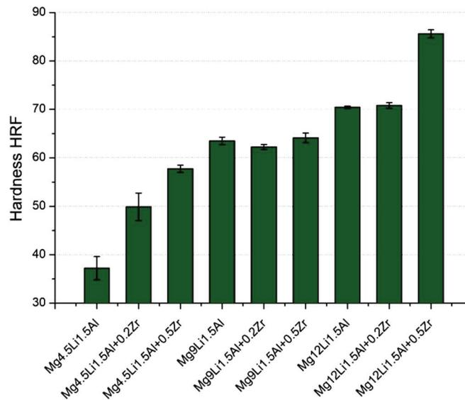
**Figure 3** Hardness of investigated Mg-Li-Al alloys
