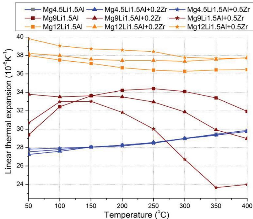
**Figure 4** Changes of linear thermal expansion coefficient of investigated Mg-Li-Al alloys
