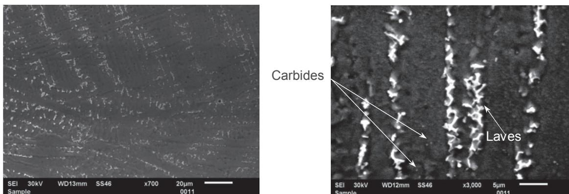
**Figure 3** Microstructure of cellular dendritic fusion zone of Inconel 625 and Inconel 718 weld
