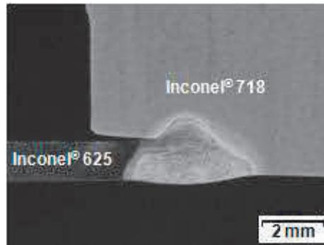
**Figure 1** Macrostructure of multi-material weld obtained by oscillated electron beam welding
