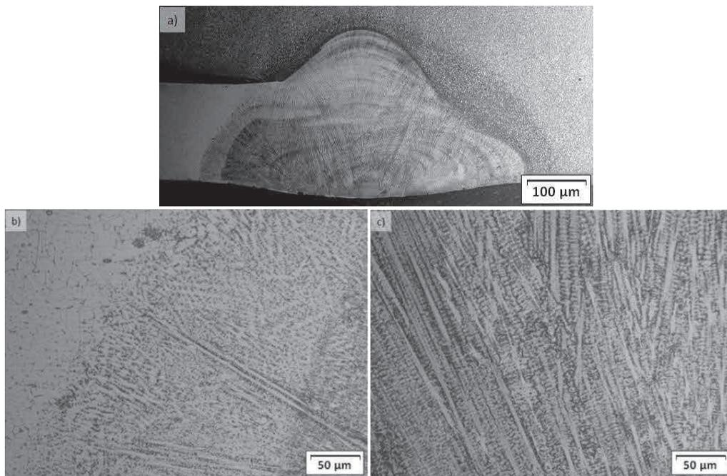
**Figure 2** Microstructure of multi-material weld of Inconel<sup>®</sup> 718 and Inconel 625:
