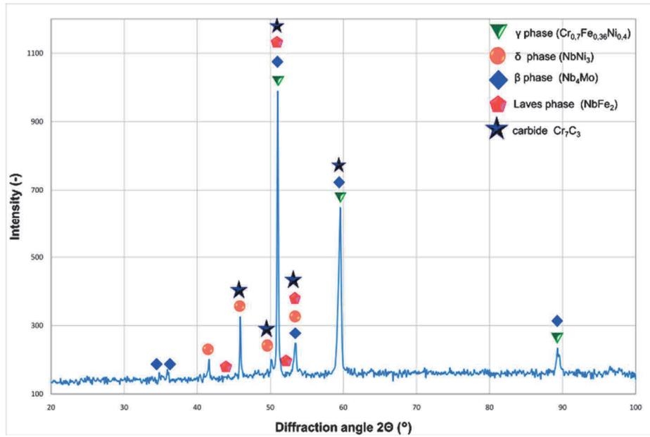
Figure 4 Diffractogram of fusion zone of Inconel 625 and Inconel 718 weld
