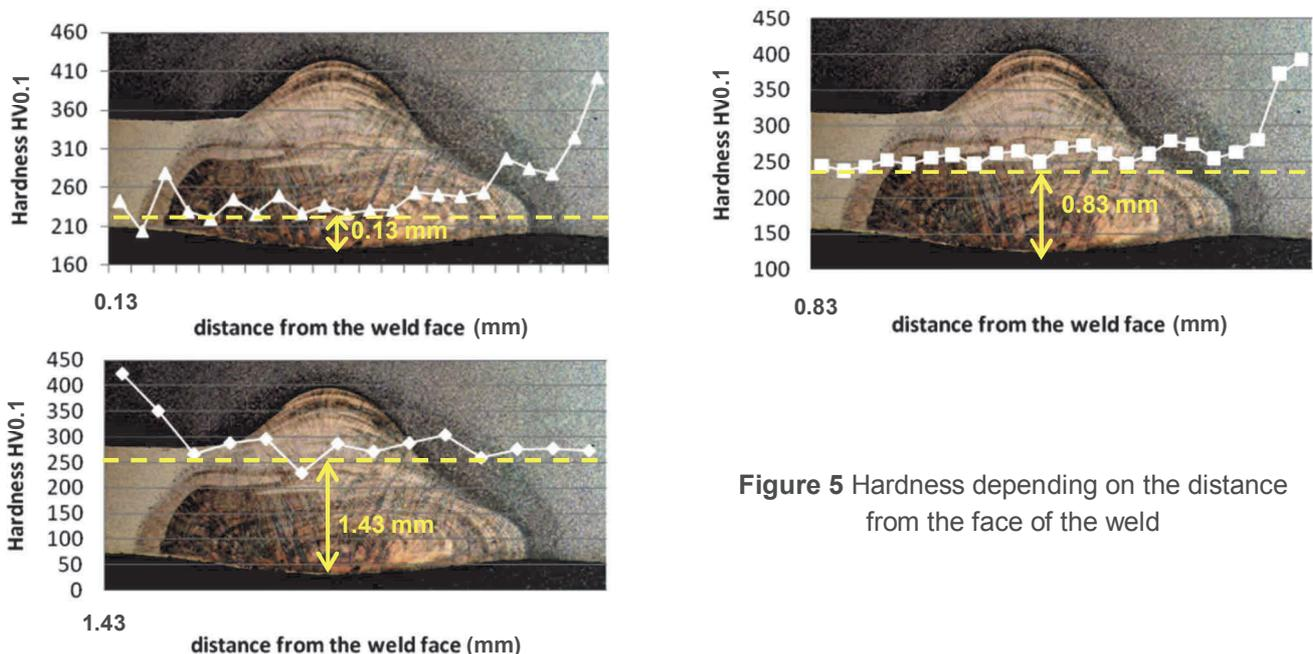
Figure 5 Hardness depending on the distance from the face of the weld
