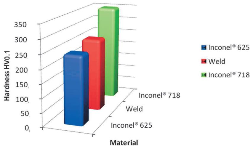
**Figure 6** Average values of hardness HV0.1 in individual zones
