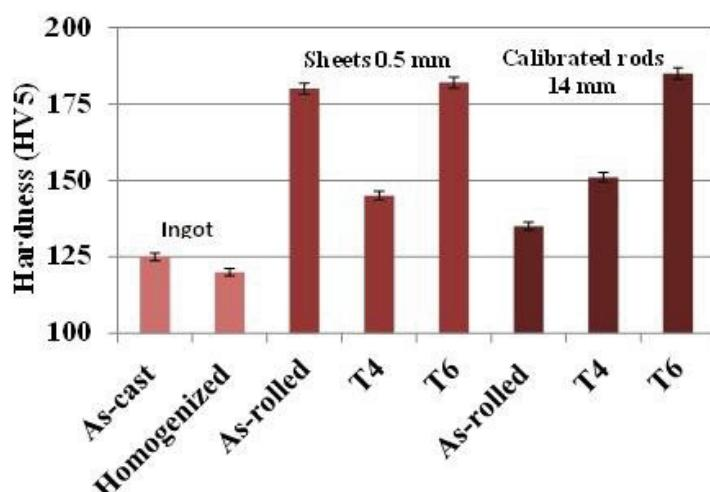
**Figure 7** Hardness of the experimental alloy depending on a processing way
