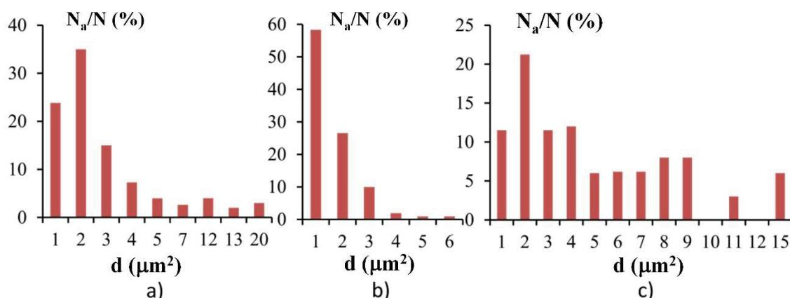
$N_a/N$  -ratio of the number of particles of size  $a$  to the total number of particles;  $d$  - area of particles ( $\mu\text{m}^2$ )
