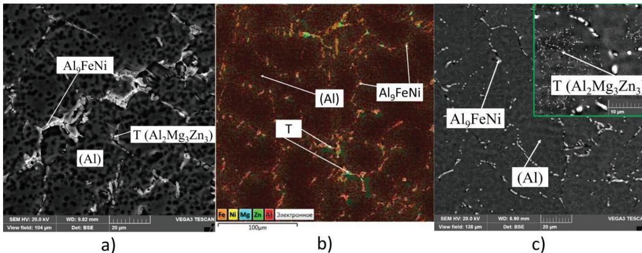
**Figure 4** Microstructure of ingot from experimental alloy: (a) as-cast SEM; (b) as-cast multilayered distribution map; (c) after two-step homogenization
