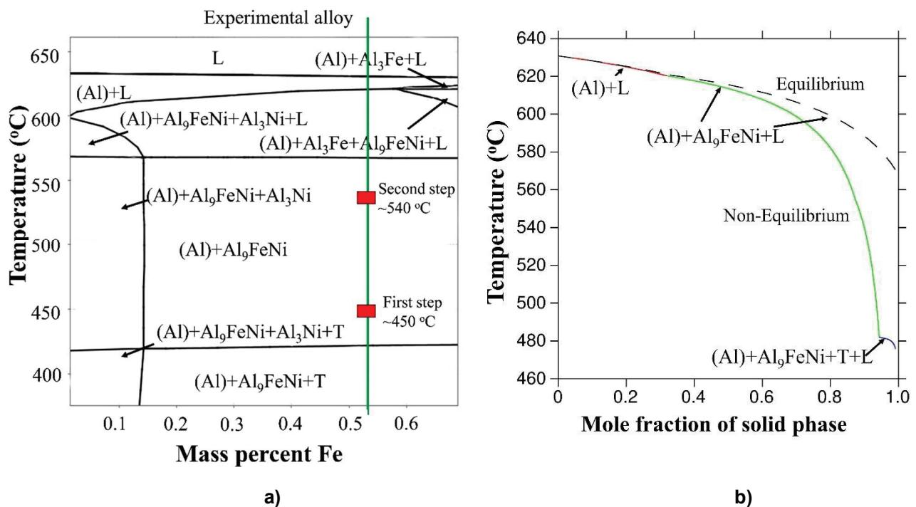
**Figure 3** Fragment of polythermal section of Al-Zn-Mg-Fe-Ni system (6.54 wt.% Zn, 2.33 wt.% Mg, and 0.67 wt.% Ni) (a) and mole fraction of solid - temperature diagram during non-equilibrium crystallization (b) [3, 4]
