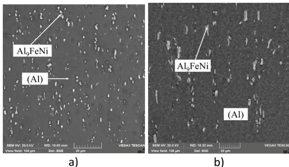
**Figure 5** Microstructure of experimental alloy after ageing in mode T6: (a) thin sheet (0.5 mm); (b) rods (14 mm)
