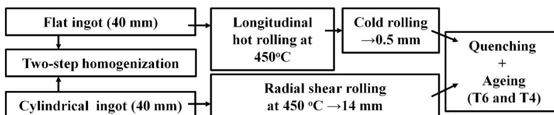
**Figure 1** Scheme of thermomechanical treatment
