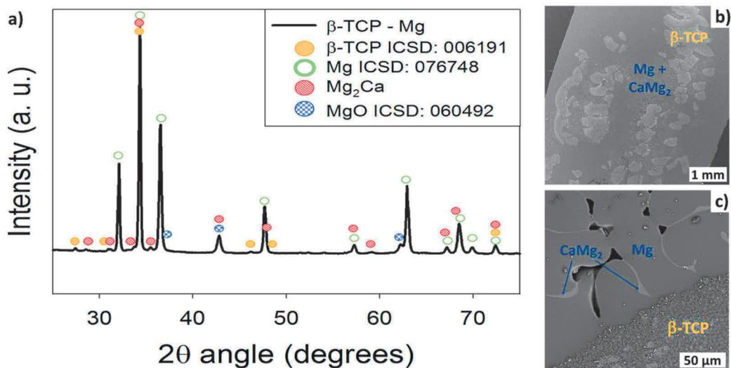
**Figure 6** a) Representative X-ray diffraction pattern of the  $\beta\text{-TCP}$  - Mg composite obtained by CAMI, b) SEM micrograph of the composite microstructure, and c) the detailed view of the  $\beta\text{-TCP}$  - Mg interface
