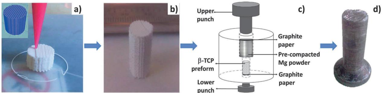
**Figure 1** Methodology process for production of  $\beta$ -TCP - Mg composite. a) the appearance of the robocasting process of a cylindrical preform carried out using the computer model (presented in the left upper corner), b) sintered preform with a 150- $\mu$ m-pore size, c) mould design and arrangement for CAMI process, and d) screw-like  $\beta$ -TCP - Mg composite obtained by CAMI
