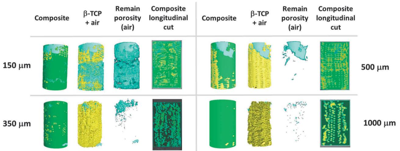
**Figure 5**  $\mu\text{CT}$  reconstruction of Mg-infiltrated  $\beta\text{-TCP}$  preforms with different pore size
