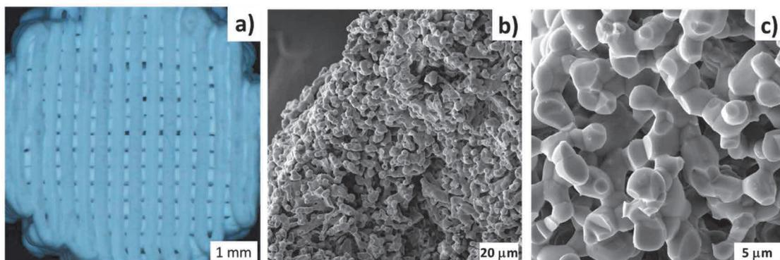
**Figure 2** a) Typical appearance of a  $\beta$ -TCP preform with a 150- $\mu$ m-pore size (light microscopy), b) representative microstructure of the sintered  $\beta$ -TCP strands, and c) detailed micrograph of the microporosity in the  $\beta$ -TCP strands of the robocast preforms.
