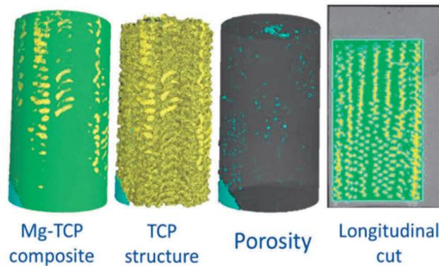
**Figure 3** 3D imaging reconstruction and phase differentiation for the infiltrated  $\beta$ -TCP - Mg composite obtained using a  $\beta$ -TCP preform with 500- $\mu$ m-pore size
