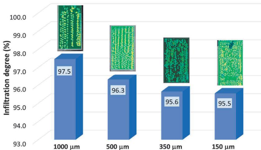
**Figure 4** Average infiltration degree in the  $\beta$ -TCP - Mg composite depending on the pore-size of the initial preforms
