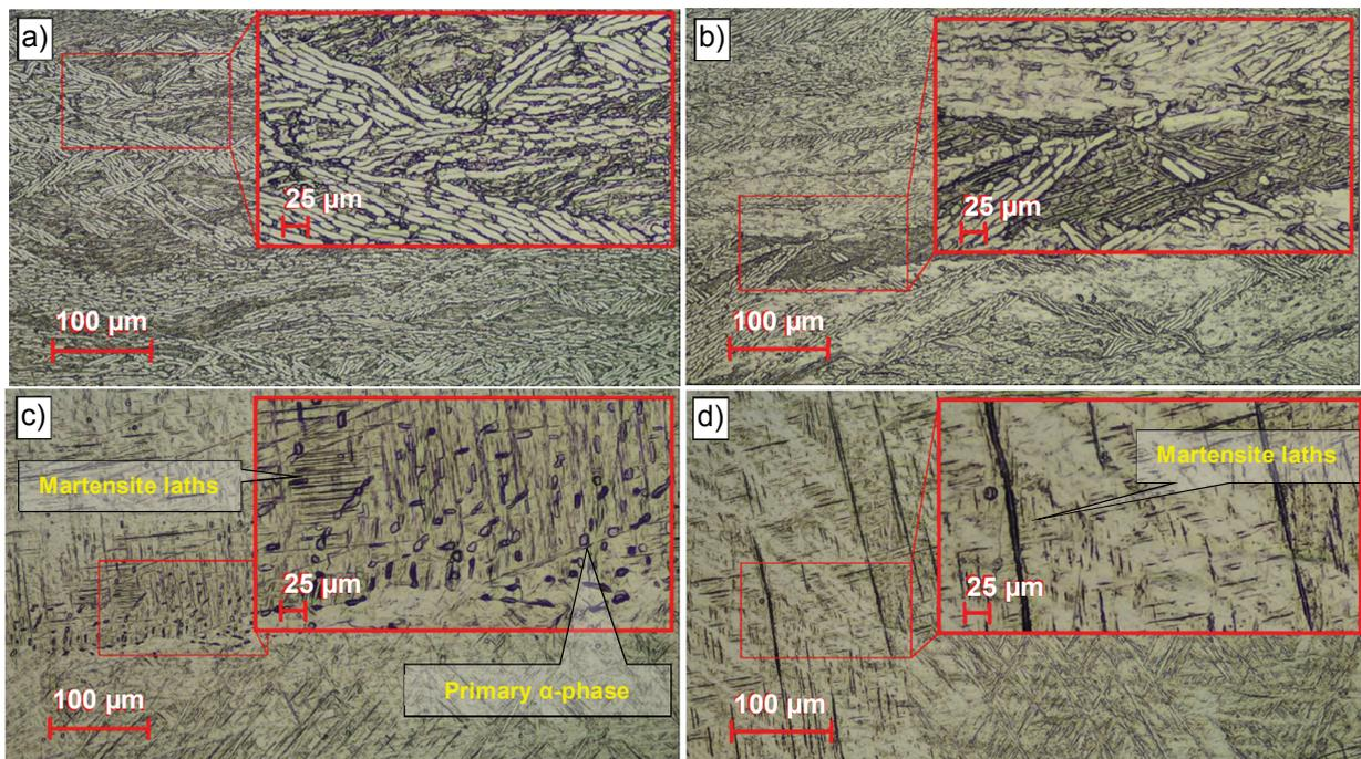
**Figure 3** Micrographs of the Ti5Al4V alloy in as-received condition and (a) after ST for 30 min at 890 °C (b); 920 °C (c) 950 °C (d) WQ. Micrographs were made at the RD.
