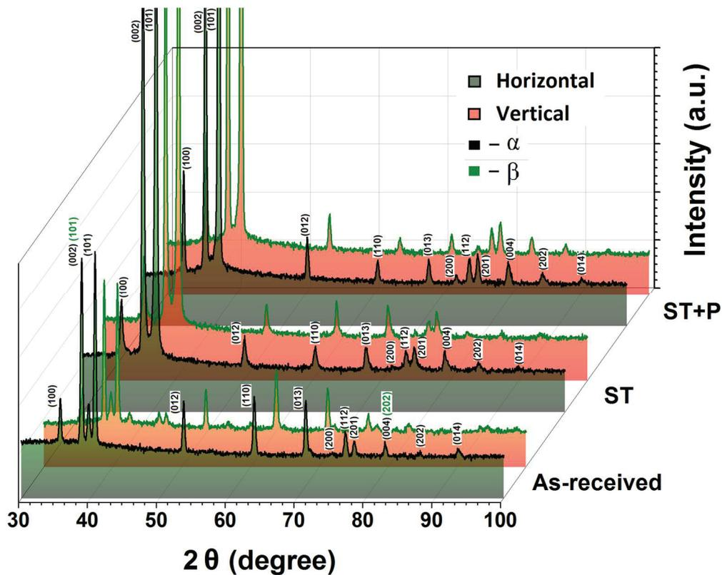
**Figure 5** XRD patterns of the as-received, ST for 30 min at 920 °C and P for 4 hours at 500 °C samples scanned in horizontal and vertical direction of the RD
