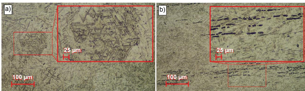
**Figure 4** Micrographs of the Ti5Al4V alloy after ST for 30 min at 920 °C and P for 4 hours at a) 500 °C and b) 520 °C
