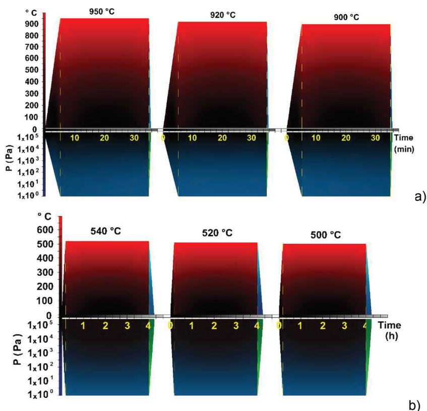
**Figure 1** Cyclograms of the applied heat treatment processes: a) solution treatment; b) precipitation
