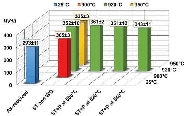
**Figure 2** Comparison of the hardness values of the Ti5Al4V samples after ST at three different temperatures and WQ, as well as after P at three different temperatures. All measurements were made at the rolling direction (RD) of the material.
