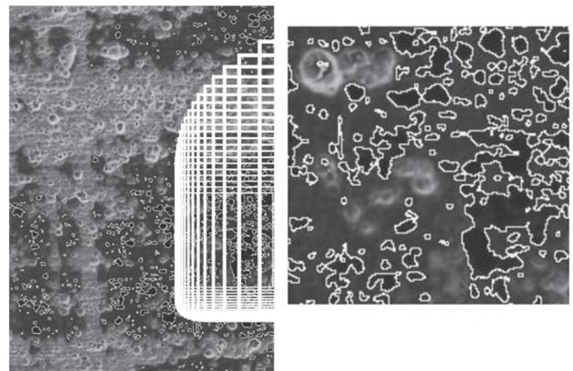
**Figure 3** Visual example of detection of sliding film on surface layer after tribology test on sample 2A4C
