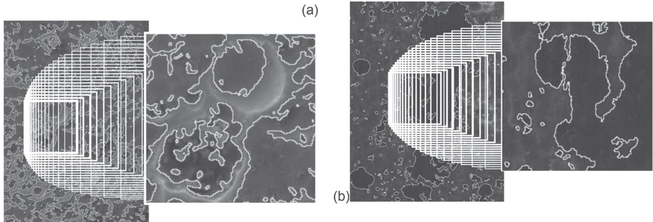
**Figure 4** Graphic presentation of detection result of specific area of surface layer (a) before tribology test ("ridge"), (b) after tribology test ("sliding film") on sample 2D3A
