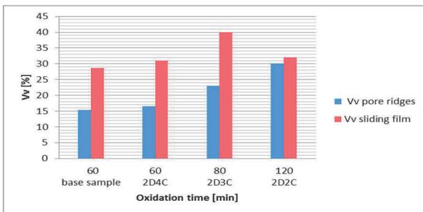
**Figure 7** Comparison the surface layer before (pores ridges) and after (sliding film) tribology test
