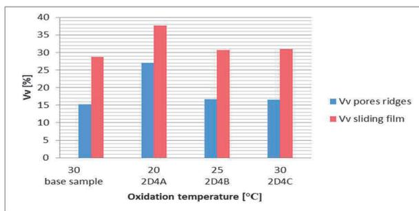
**Figure 5** Comparison the surface layer before ("pores ridges") and after ("sliding film") tribology test
