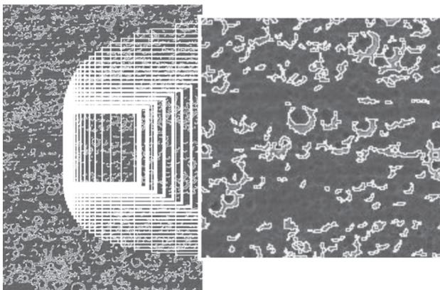
**Figure 2** Visual example of detection of pores of ridges before tribology test on sample 2A4C
