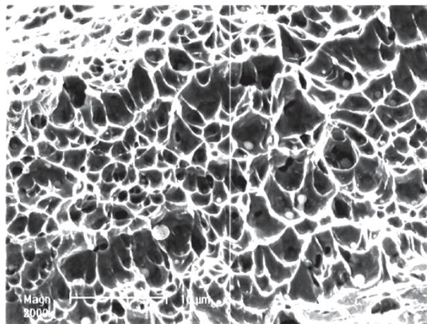
**Figure 1** Fracture surface of metal weld deposit with 0.3 % Mo (small size of inclusions) [1]
