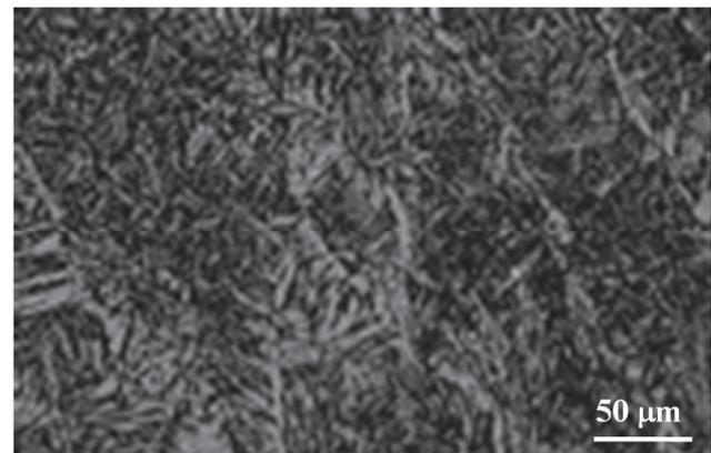
**Figure 2** Acicular ferrite above 60 % in various deposits (of laser welding with micro-jet cooling on the left, of MAG welding on the right)
