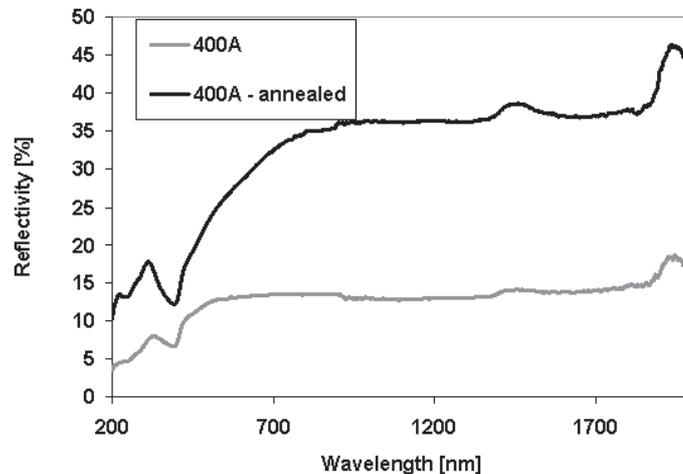
**Figure 7** Reflectivity of the as-sprayed and annealed 400 A coating
