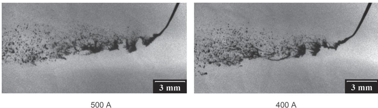
**Figure 1** Shadowgraph of suspension injection into the plasma jet (bright area)
