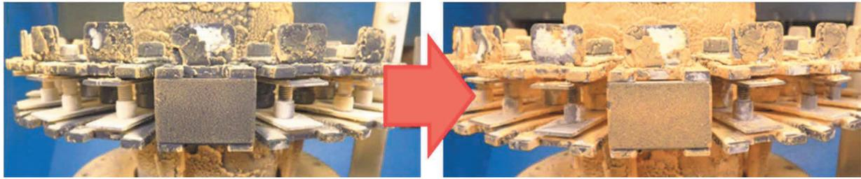
**Figure 5** 400 A sample before (left) and after annealing by plasma torch
