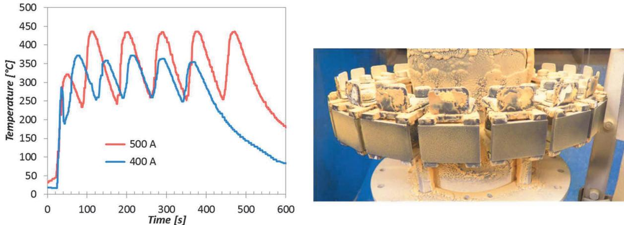
**Figure 2** Left) Sample temperature history during deposition. Right) Samples after the coating deposition. Experiment 500 A
