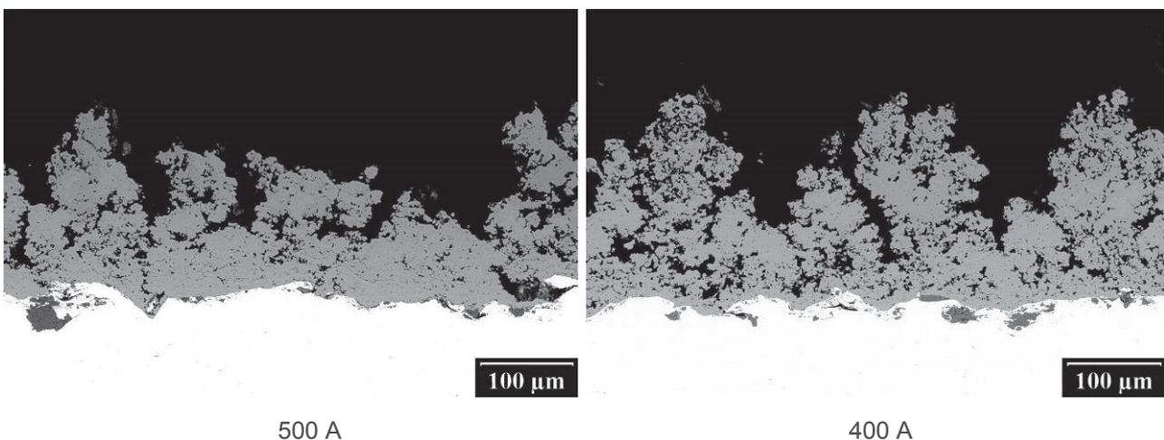
**Figure 3a** Cross-sections of the deposited coatings
