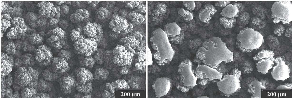
**Figure 6** Free surface of the deposited 400 A coating before and after additional annealing by plasma torch
