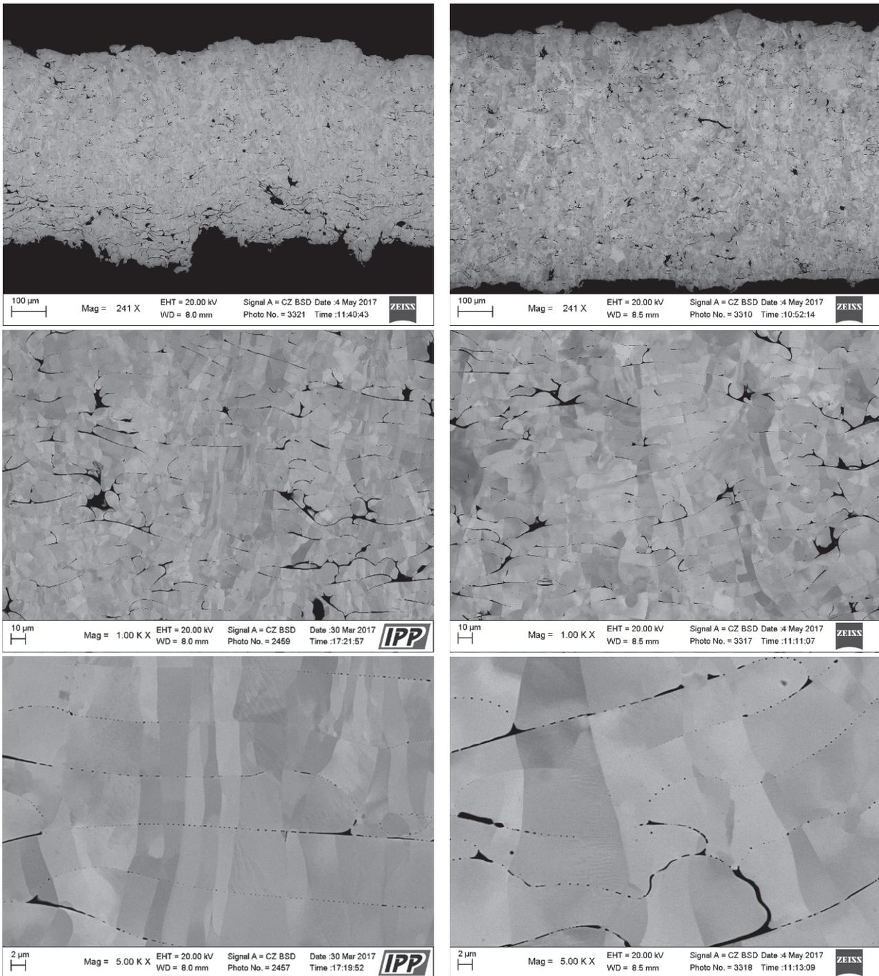
**Figure 4** Microstructure of the coatings: without preheating (left) and with preheating (right), general overview (top row), cross-section showing span of the columnar grain trough several splats (middle row), detail of the columnar grains (bottom row)
