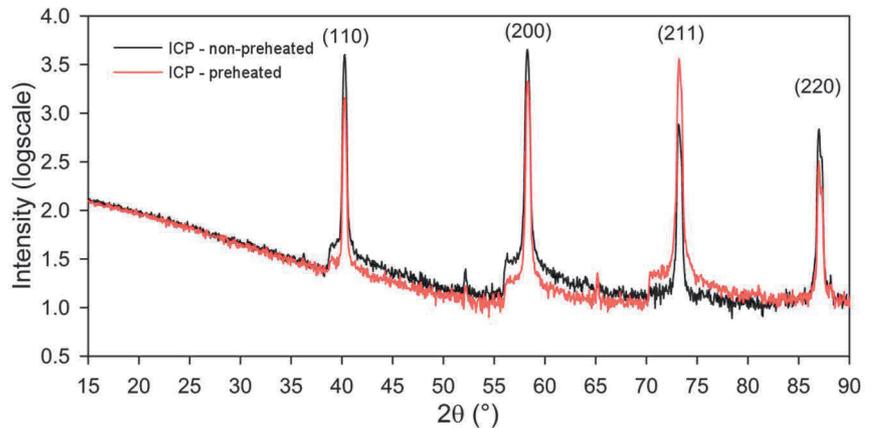
**Figure 2** Diffraction patterns from the free surfaces of the samples documenting pure W coating
