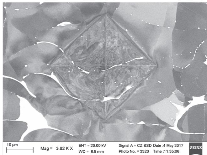
**Figure 5** Indentation in the cross-section of the preheated sample
