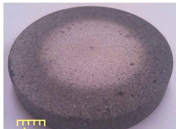
**Figure 1** Preheated sample after tungsten coating deposition
