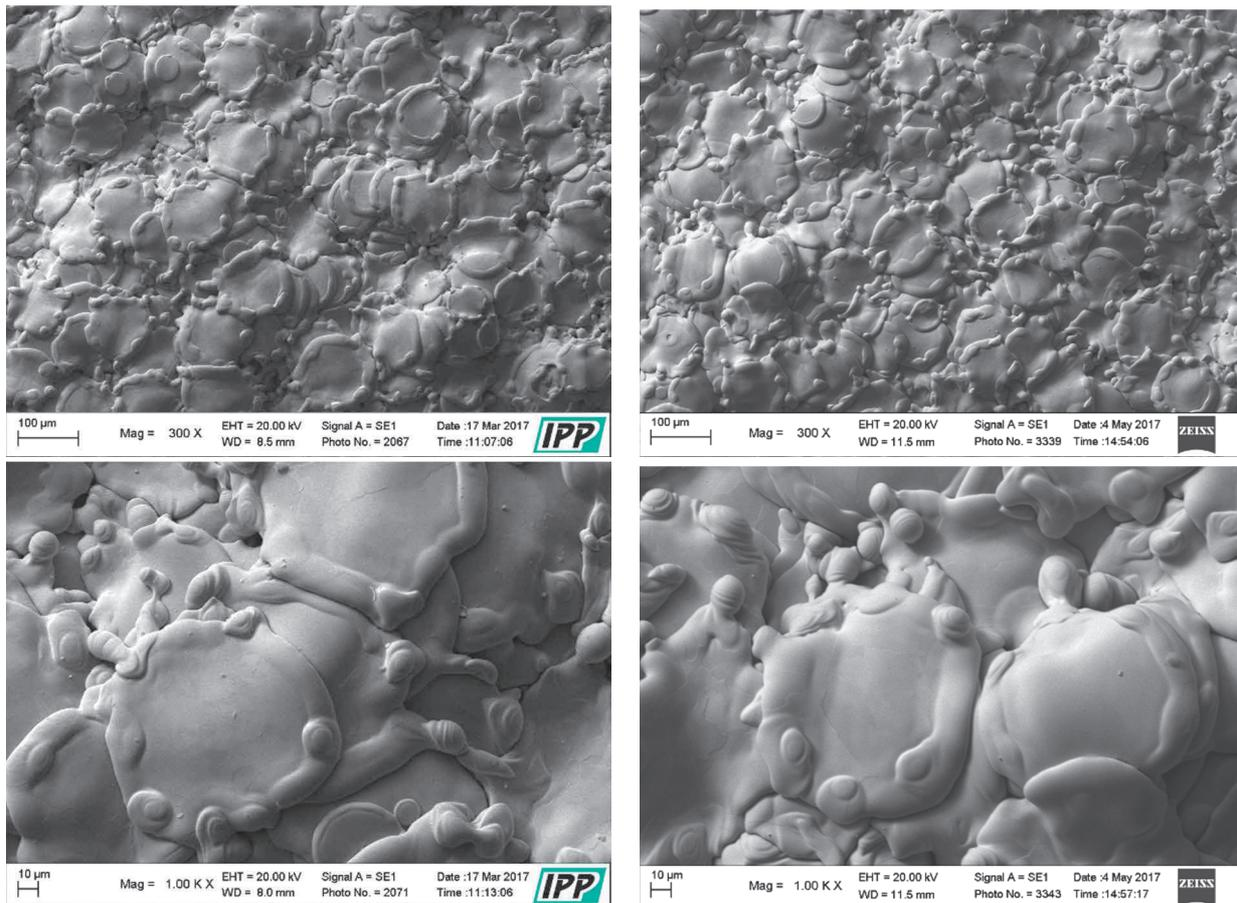
**Figure 3** Micrographs of the coatings free surface: without preheating (left) and with preheating (right)
