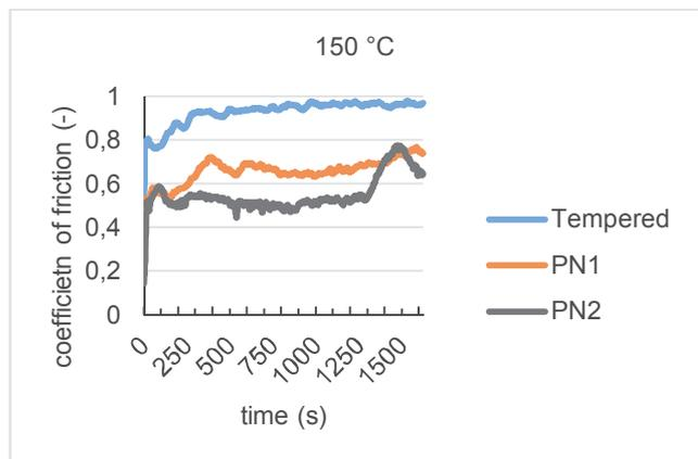
**Figure 4** Coefficient of friction at 150 °C
