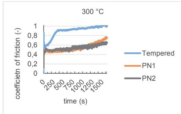
**Figure 5** Coefficient of friction at 300 °C
