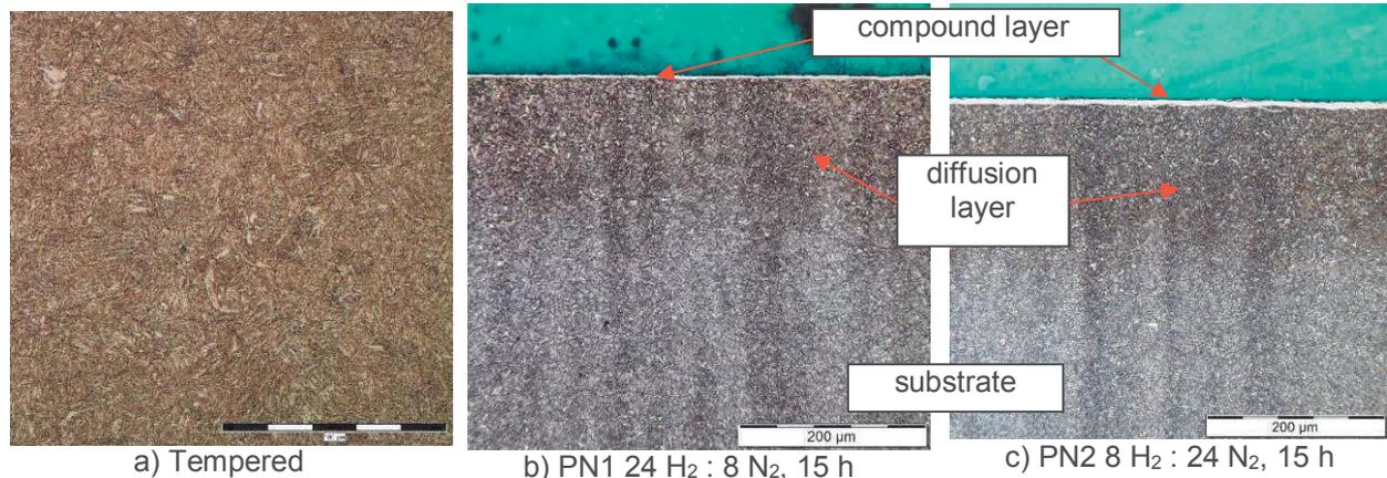
**Figure 1** Cross-sectional microstructure (500x)
