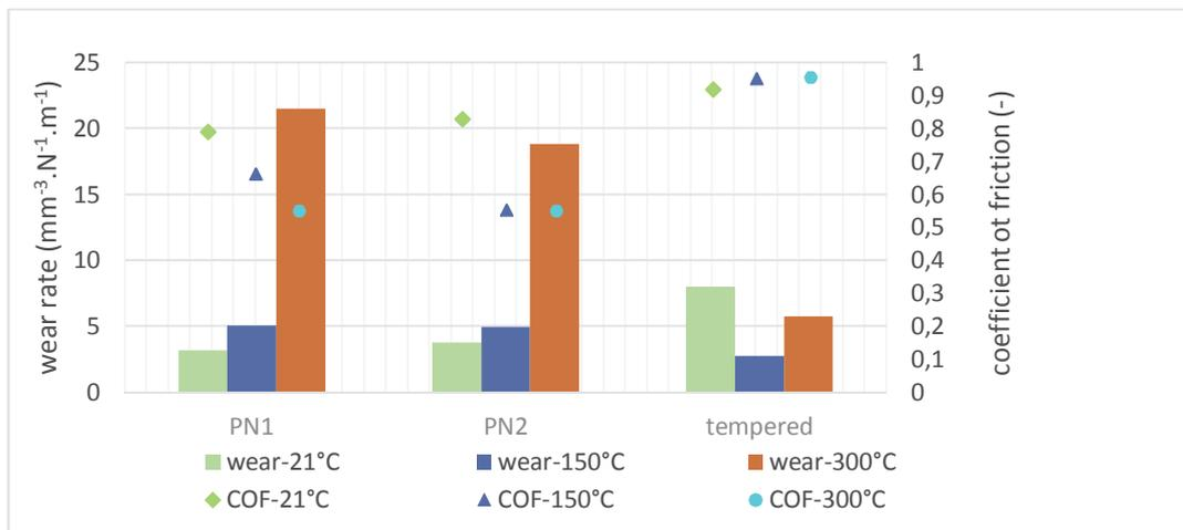
**Figure 6** Relationship between the wear rate and the coefficient of friction
