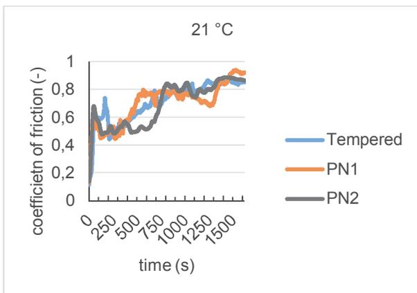
**Figure 3** Coefficient of friction at 21 °C
