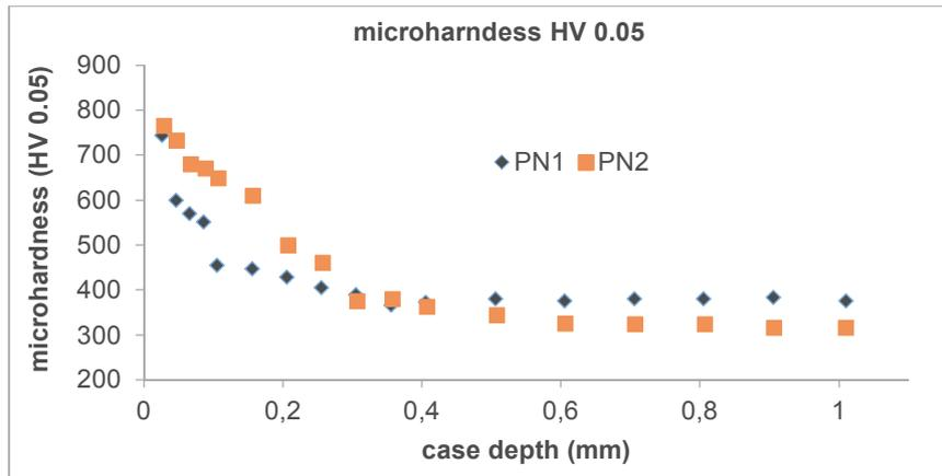
**Figure 2** Microhardness of nitrided sample
