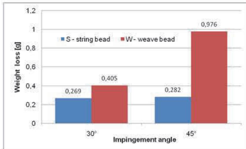
Figure 6 Results of erosion tests
