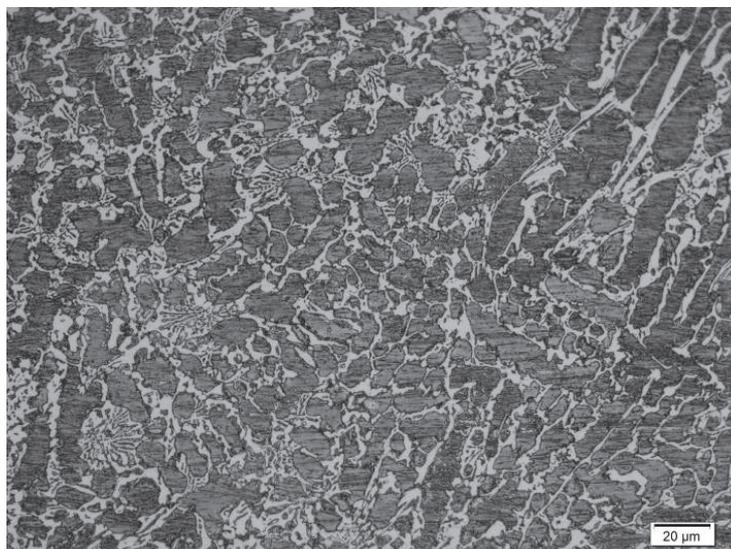
**Figure 4** Structure of coating made with weave bead, a) magnification x50, b) magnification x500
