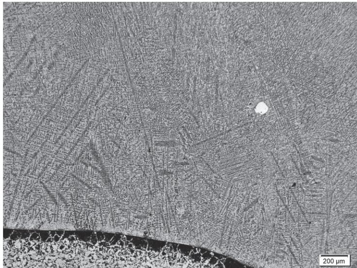
**Figure 3** Structure of coating made with weave bead, magnification x50
