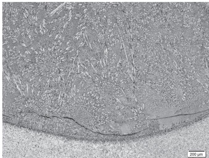
**Figure 1** Structure of coating made with string bead, magnification x50
