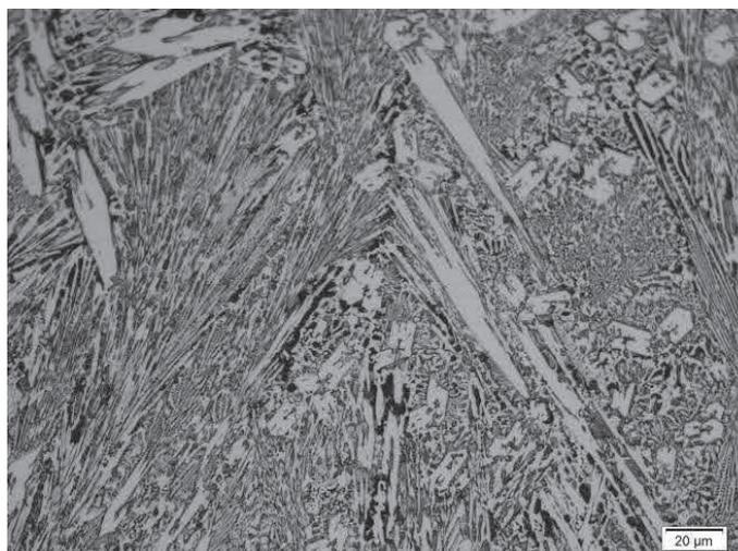
**Figure 2** Structure of coating made with string bead, magnification x500
