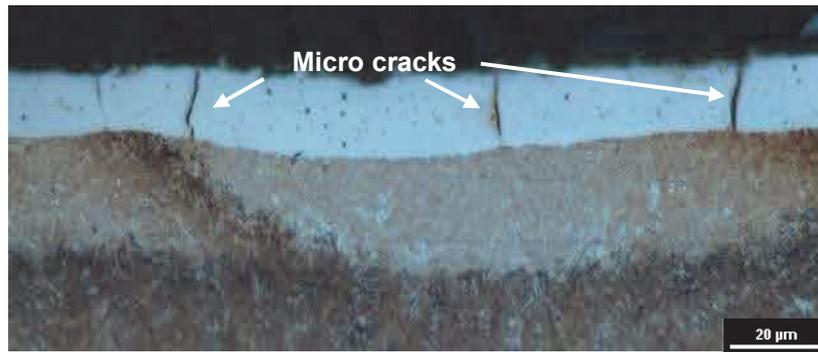
**Figure 5** Metallographic structure - micro cracks in the white layer for machining parameters:
