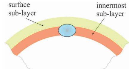
**Figure 2** Scheme of CNTL sub-layers with a fish-eye crack on the fracture surface.
