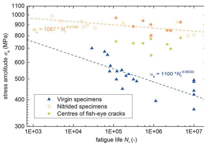
**Figure 5** The S-N curves of nitrided and virgin specimens along with experimental data
