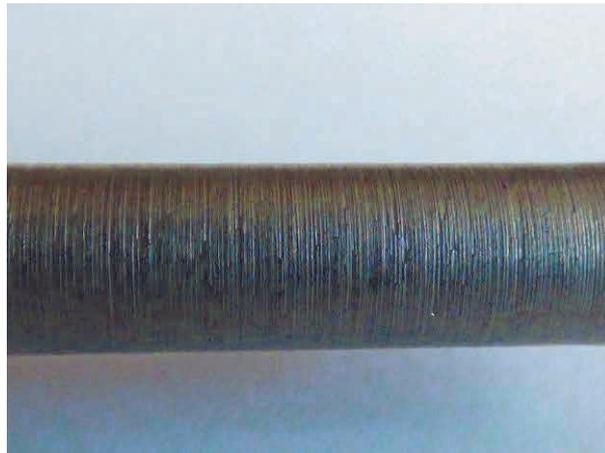
**Figure 4** Circumferential micro-scratches on the specimen surface caused by turning
