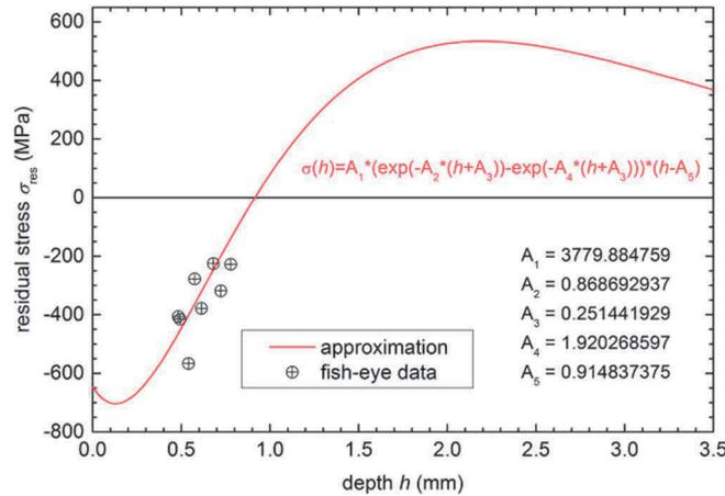
**Figure 6** The fitting curve  $\sigma_{res}(h)$  determining the profile of calculated residual stresses inside the nitrided specimens with surfaces finished by turning.
