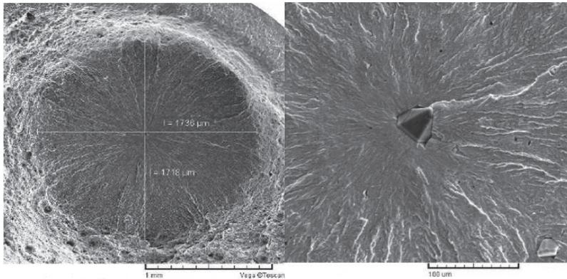
**Figure 1** Fish-eye crack in a nitrided specimen; a) the global SEM view b) inclusion in the fish-eye centre.
