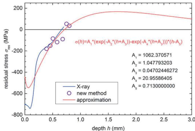
**Figure 3** Stress profiles obtained by experiment (X-ray) and approximation of fish-eye data (new method) for nitrided specimens with surfaces finished by fine-grinding
