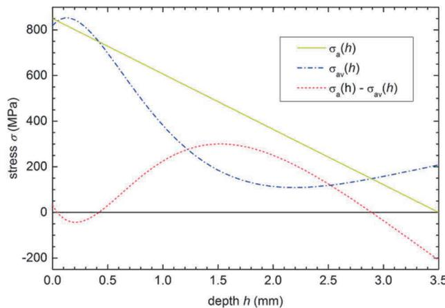
**Figure 7** Comparison of fatigue limit of virgin specimens modified by the predicted residual (mean) stress in the bulk of the nitride specimens ( $\sigma_{av}(h)$ ) with the bending stress along the whole specimen radius, applied at the fatigue limit of nitrided specimens ( $\sigma_{av}(h)$ ). The difference between the applied bending stress and the modified fatigue limit of virgin specimens ( $\sigma_a(h) - \sigma_{av}(h)$ ) is also plotted.
