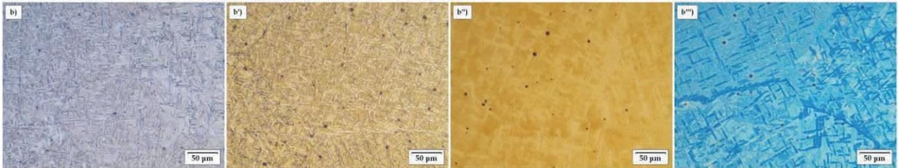
**Figure 1b** Microstructure of the porous sinters 100% Ti-6Al-4V (25 MPa): b) before thermal oxidation and after thermal oxidation at temperatures: b') 400°C, b'') 500°C, b''') 600°C
