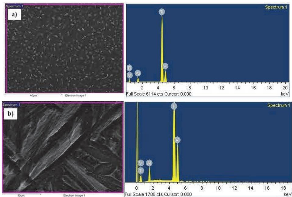
**Figure 3** Analysis of chemical composition (Spectrum 1): a) 100% Ti-6Al-4V (bulk alloy) after thermal oxidation at temperature 400°C, b) 100% Ti-6Al-4V (porous sinterers) after thermal oxidation at temperature 500°C
