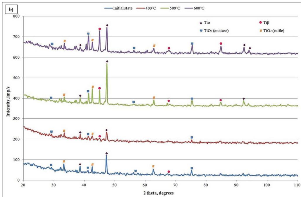
**Figure 4** Diffractograms of the titanium alloy after thermal oxidation at appropriate temperatures: a) 100% Ti-6Al-4V (bulk alloy), b) 100% Ti-6Al-4V (porous sinters)
