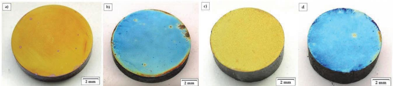
**Figure 2** Macroscopic images of the titanium alloys after thermal oxidation at appropriate temperatures:
