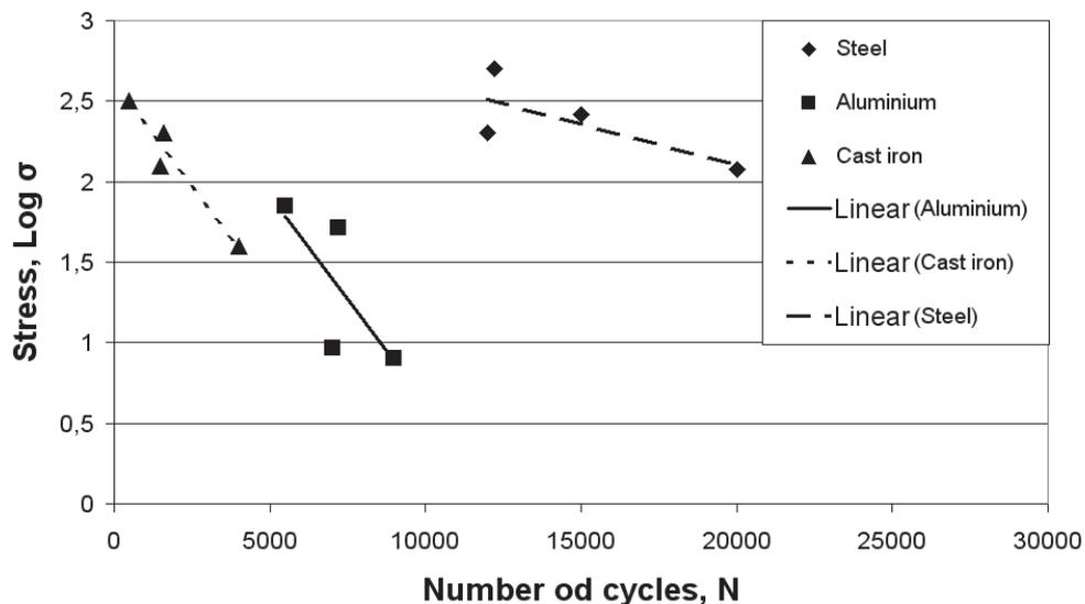
**Figure 4** A diagram of the fatigue strength as a function of the number of cycles
