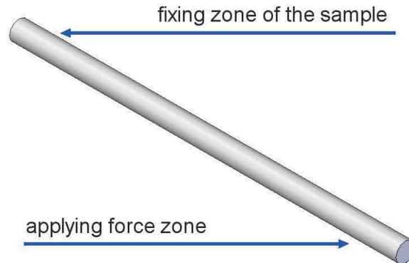
**Figure 3** Form of material sample taken from the swingarm
