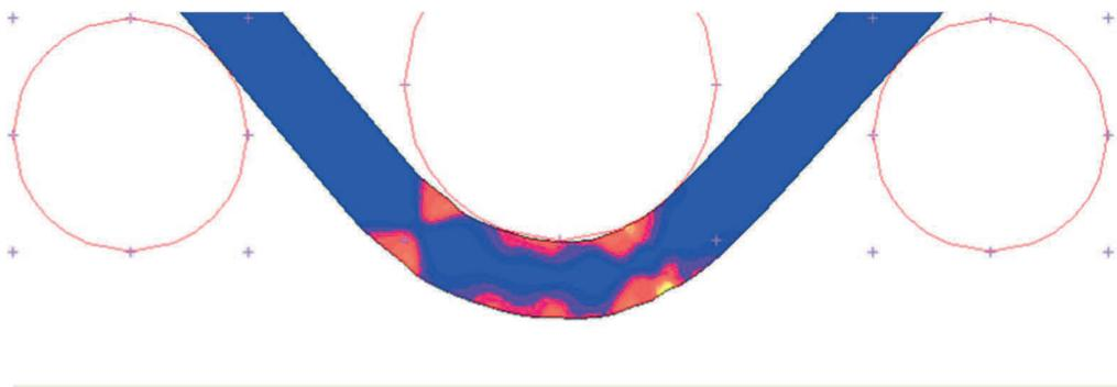
**Figure 8** Strains calculation based on local material properties obtained with the M-TT
