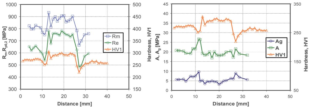
**Figure 5** Mechanical properties assessment across the heterogeneous weld
