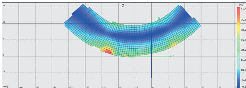
**Figure 9** Experimentally measured strains
