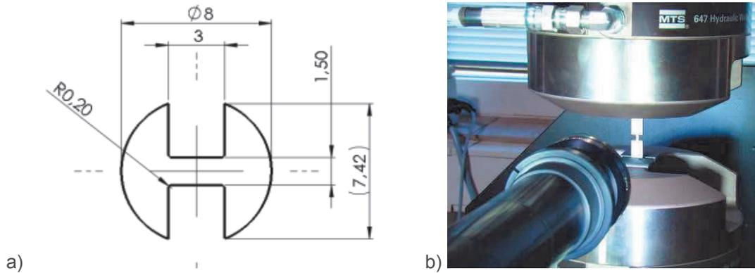
**Figure 2** a) M-TT specimen geometry, b) Testing set up for M-TT tests with ARAMIS system
