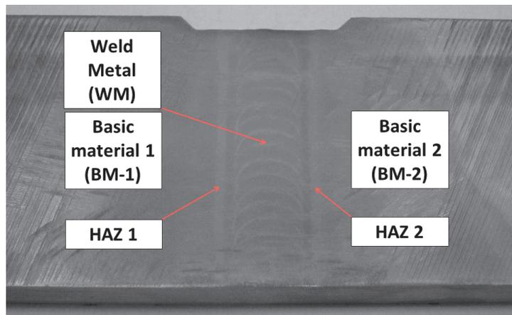
**Figure 1** Macro of the investigated heterogeneous weld
