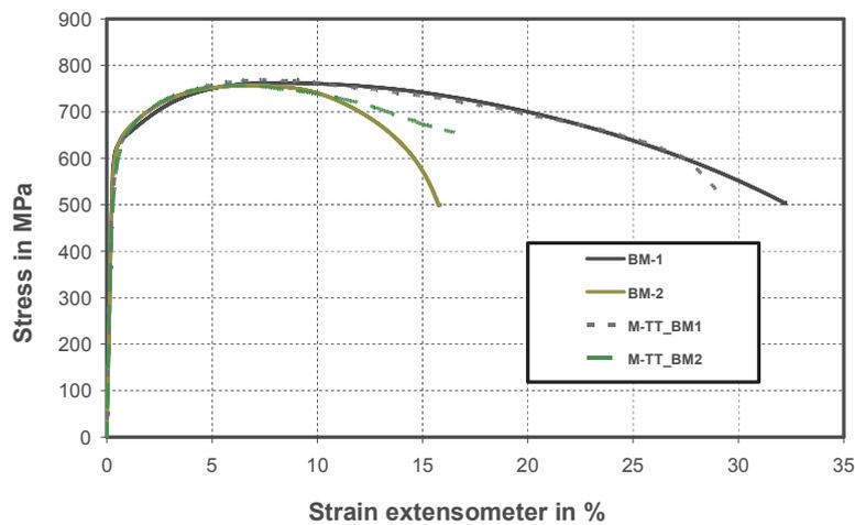
**Figure 4** Comparison of standard tensile test records with M-TT records
