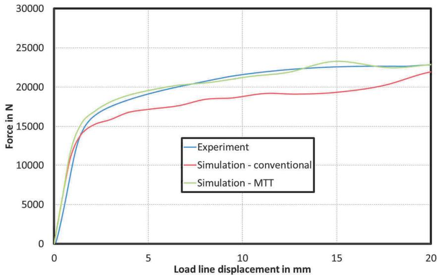
**Figure 10** Comparison of records obtained during experimental measurement and simulation using local data from the M-TT and simulation using global material properties
