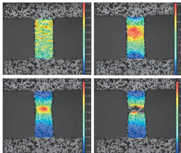
**Figure 3** Example of strain measurement at different stages of tensile test for M-TT
