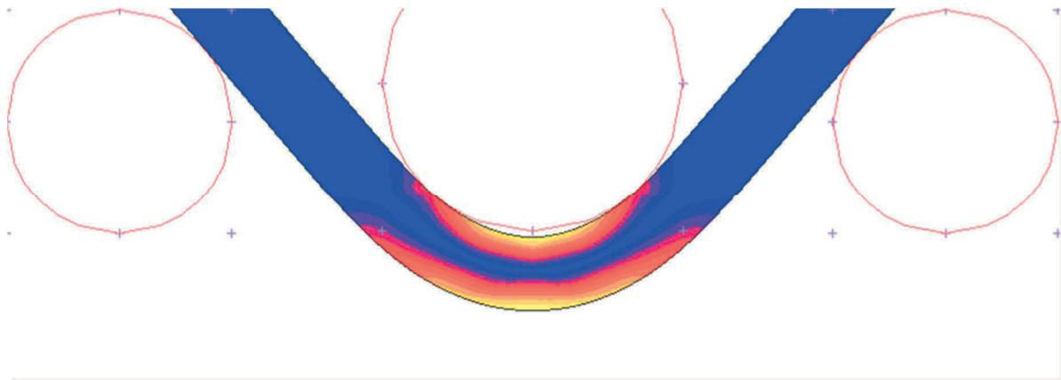
**Figure 7** Strains calculation based on global material properties
