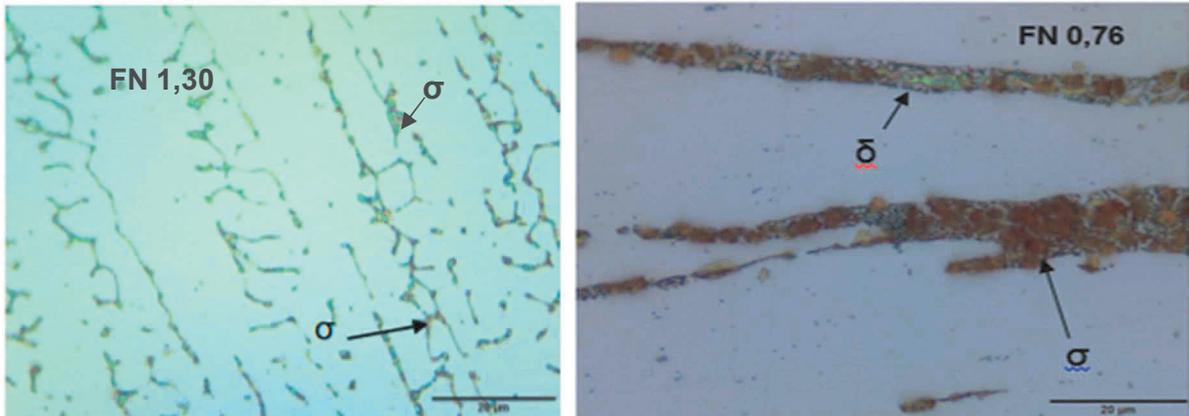
**Figure 4** Welded zone after 7 min exposure and transition, weld/base metal, at 15 min of exposure
