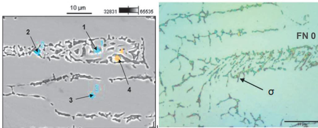
**Figure 5** AISI 317L during EDS analyzes and OM image on the transition region, weld to base metal
