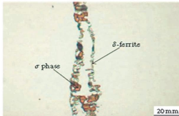
**Figure 3** AISI 316L showing  $\sigma$  phase formation from  $\delta$  ferrite [10]
