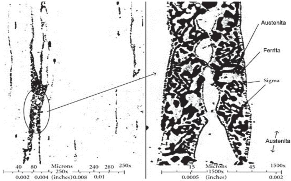
**Figure 1** AISI 304 aged at 650 °C up to 31000h, magnetic etched [6]
