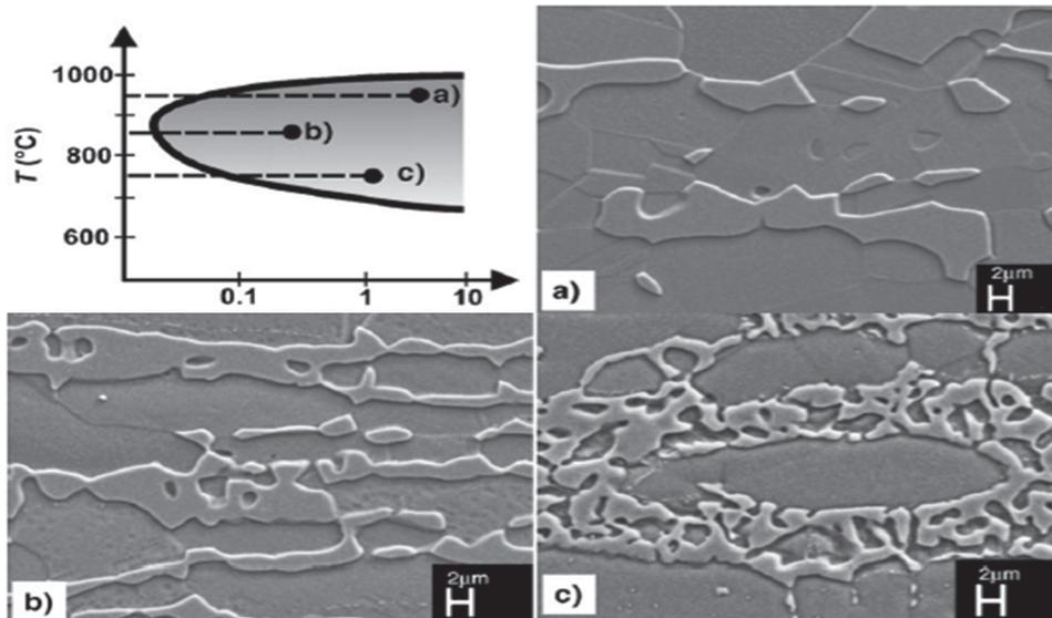
**Figure 2** Morphology of the sigma phase with respect to the isothermal annealing temperature, S31803 DSS; (a) 950 °C, (b) 850 °C, (c) 750 °C [9]
