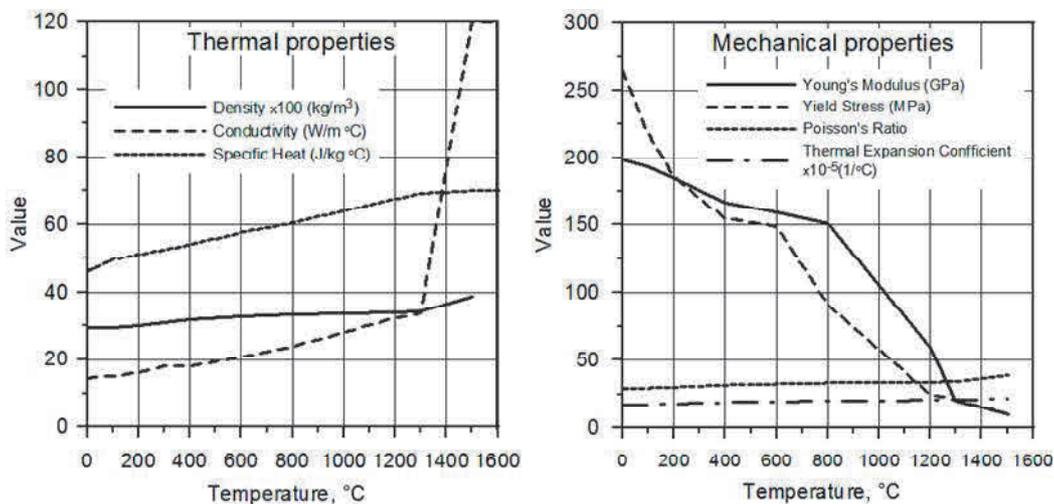
**Figure 2** Thermomechanical properties assumed in calculations [3]
