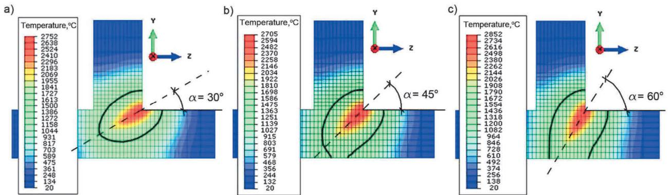
**Figure 4** Temperature distribution in cross section of welded T-joints
