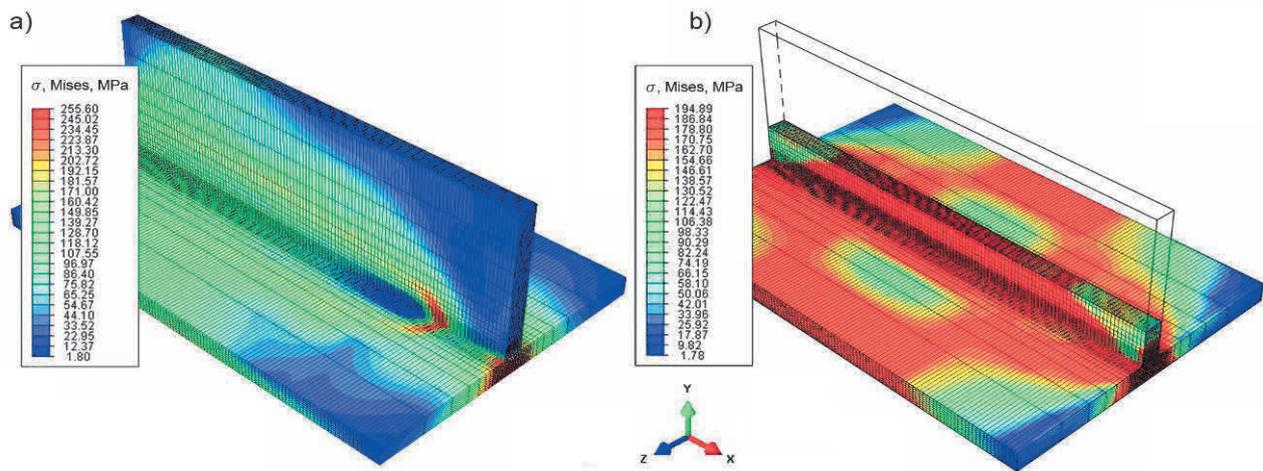
**Figure 5** Residual reduced stress  $\sigma$  of welded T-joints: a) temporary and b) residual
