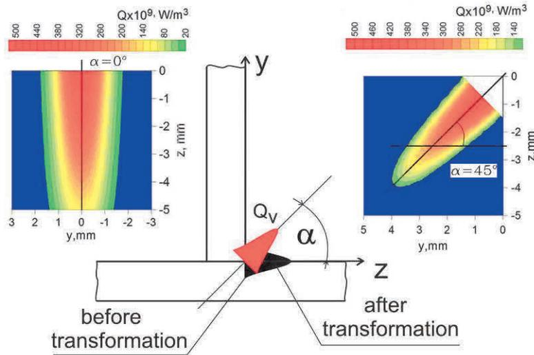
**Figure 3** Transformation of heat source power distribution
