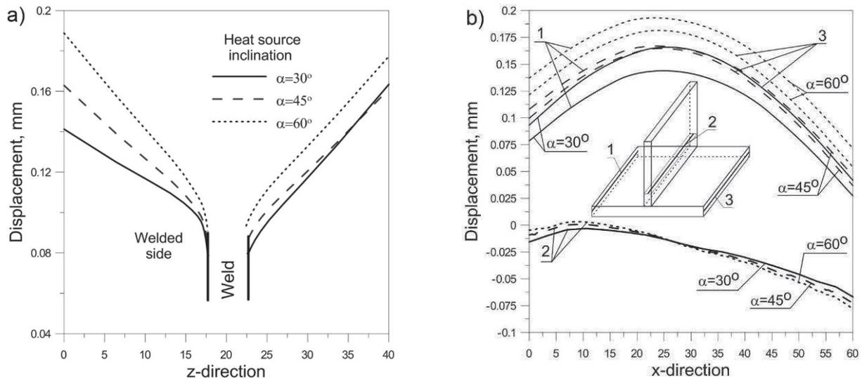
**Figure 6** Numerically estimated deflection  $U_y$ : a) in cross section of welded T-joint, b) in longitudinal section of the joint
