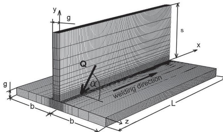
**Figure 1** Scheme of analyzed domain with the finite element mesh
