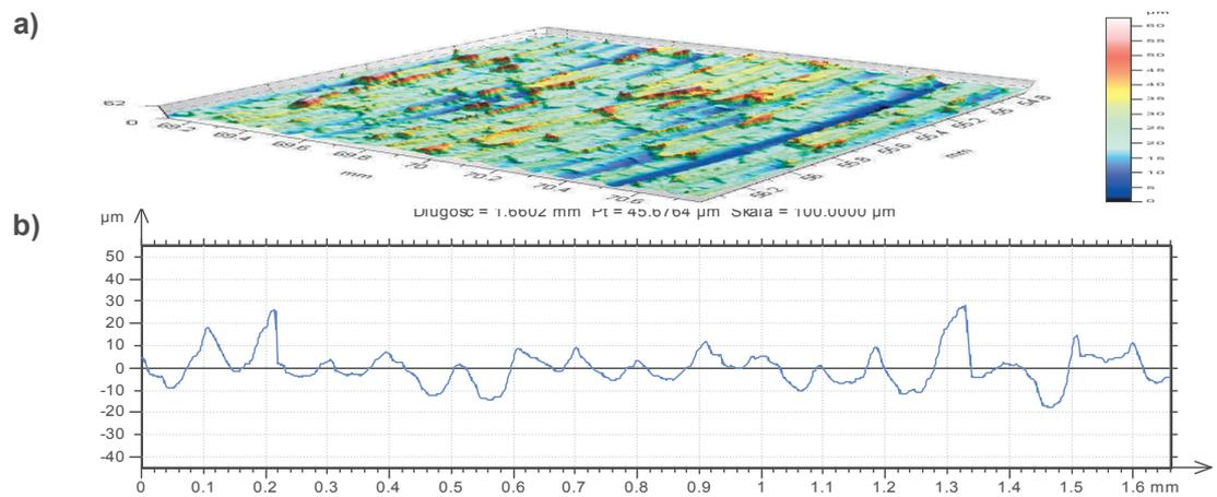
**Figure 5** Workpiece surface after turning with cutting fluid: a) 3D surface texture and b) roughness profile
