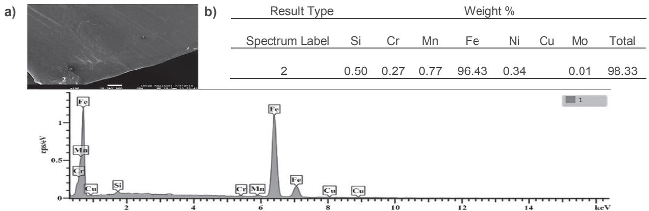
**Figure 6** SEM analysis of the tool wear after dry turning: a) image of the wear track and b) X-ray energy spectrum
