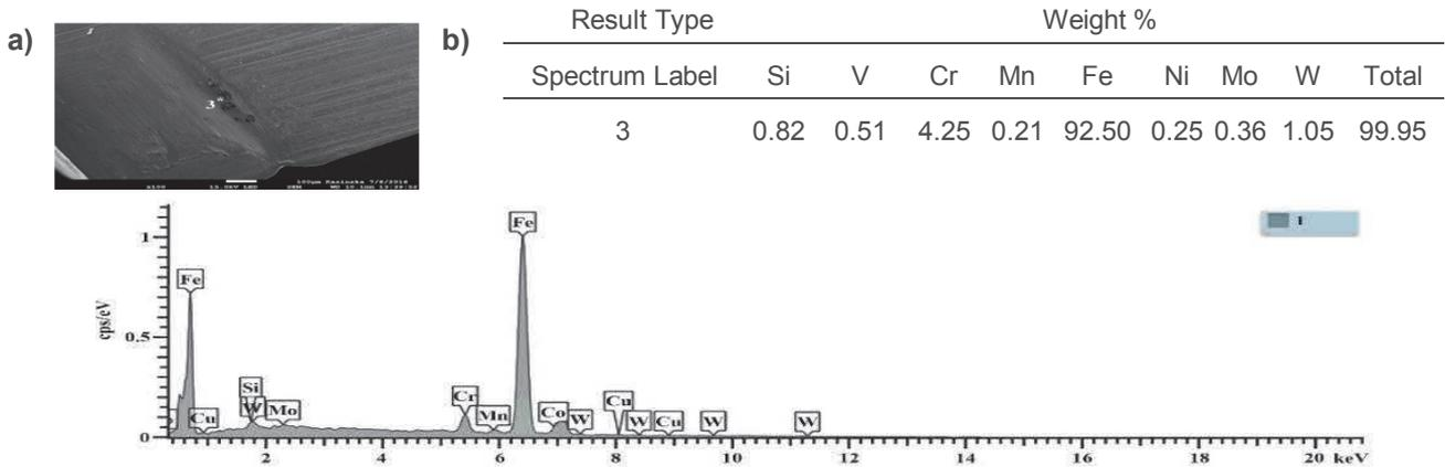
**Figure 7** SEM analysis of the tool wear after wet turning: a) image of the wear track and b) X-ray energy spectrum
