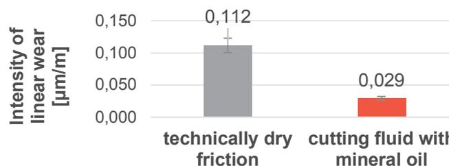
**Figure 10** Intensity of linear wear for dry and wet turning
