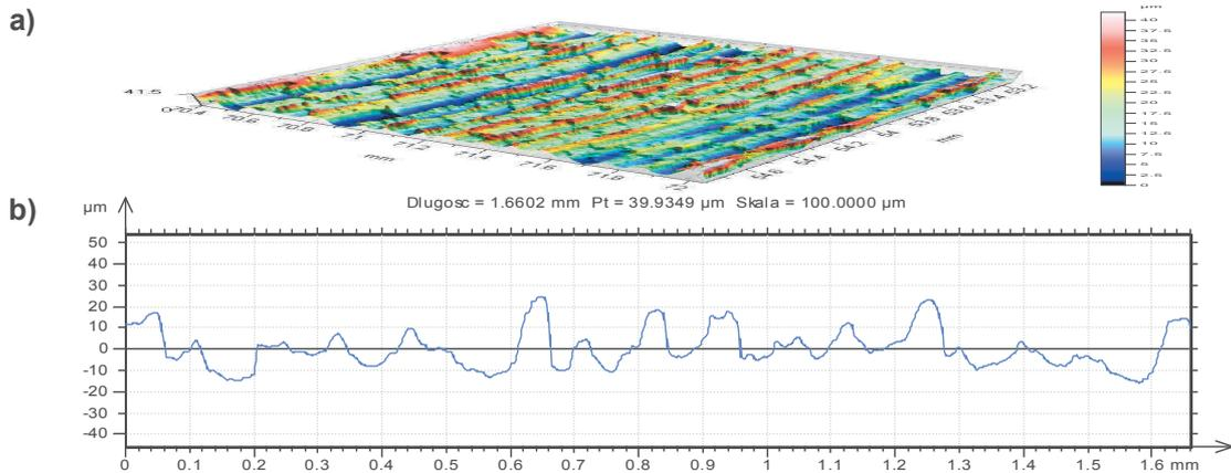
**Figure 4** Workpiece surface after dry turning: a) 3D surface texture and b) roughness profile
