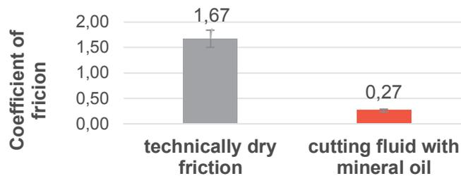
**Figure 9** Coefficient of friction for dry and wet turning
