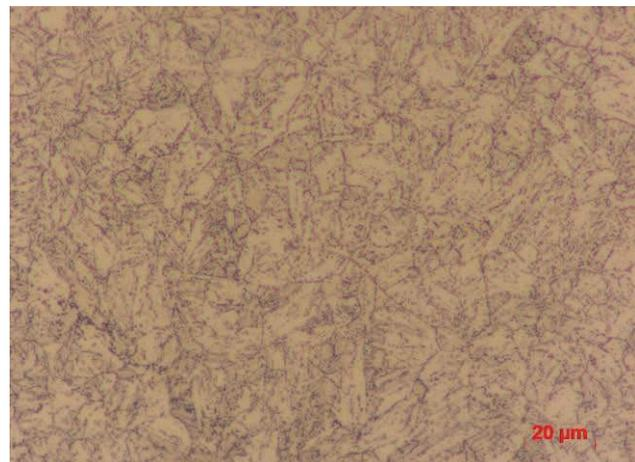
**Figure 3** Microstructure of the P92 steel, LM
