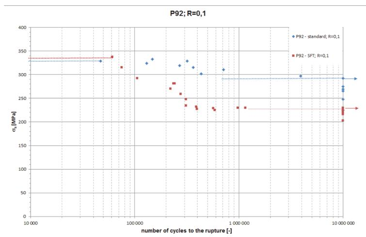
**Figure 11** Comparing results of traditional and SFT fatigue samples from steel P92, cycle asymmetry  $R=0.1$
