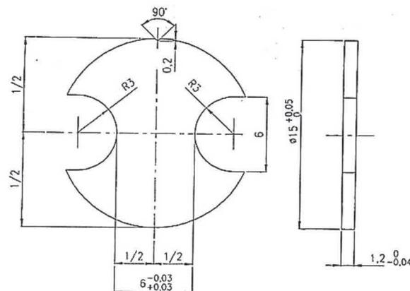
**Figure 1** Shape of Small Fatigue Test samples by [2]
