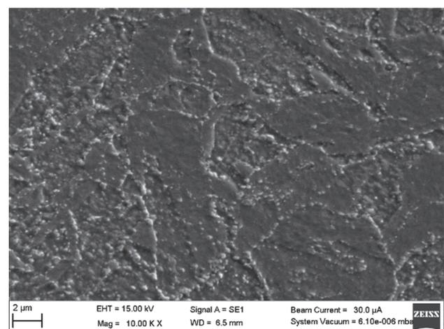
**Figure 5** Microstructure of the P92 steel, SEM
