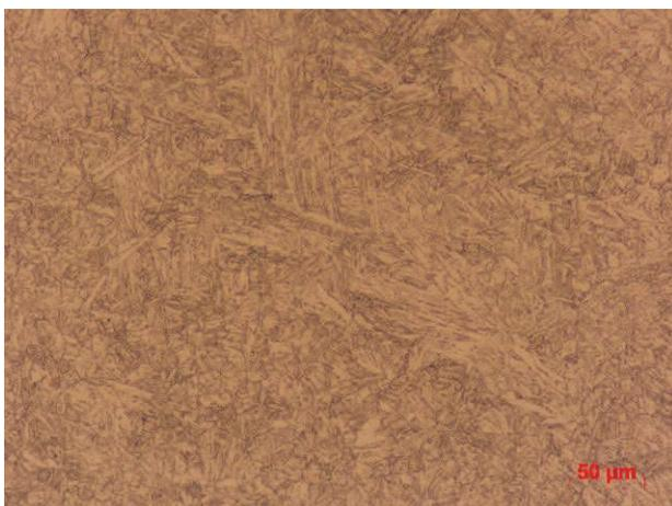
**Figure 2** Microstructure of the P92 steel, LM
