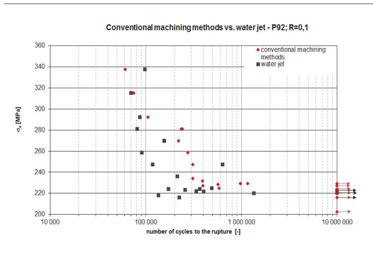
**Figure 12** Comparing results of SFT fatigue samples from steel P92, cycle asymmetry R=0.1
