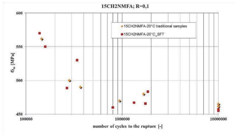
**Figure 10** Comparison of results of traditional and SFT samples from steel 15CH2NMFA, cycle asymmetry  $R=0.1$
