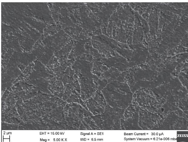
**Figure 4** Microstructure of the P92 steel, SEM
