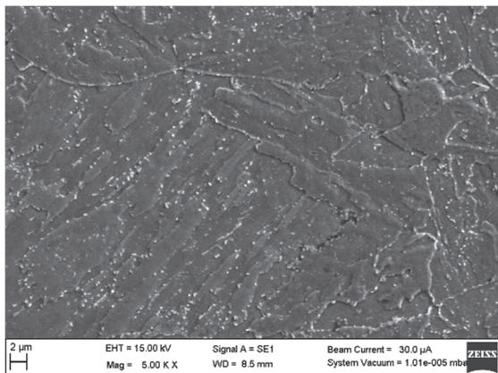
**Figure 8** 15CH2NMFA - microstructure, SEM
