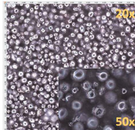
Figure 3 Magnification of metal powder 316L
