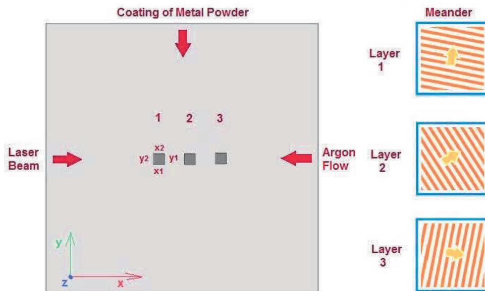
Figure 4 Layout of samples during printing
