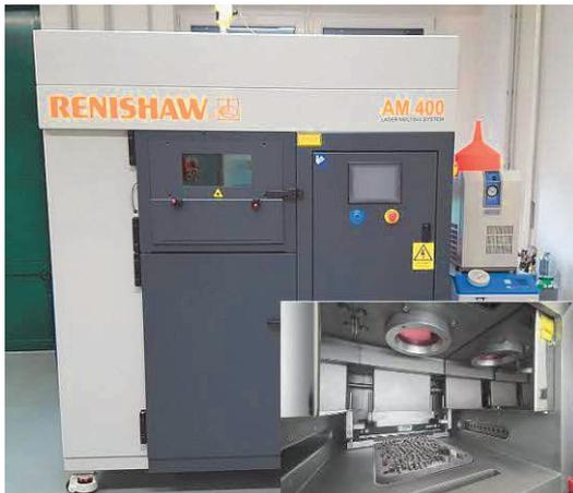
Figure 2 3D Printer Renishaw AM 400
