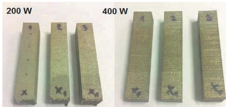
**Figure 5** The printed samples from material 316L at different machine performance
