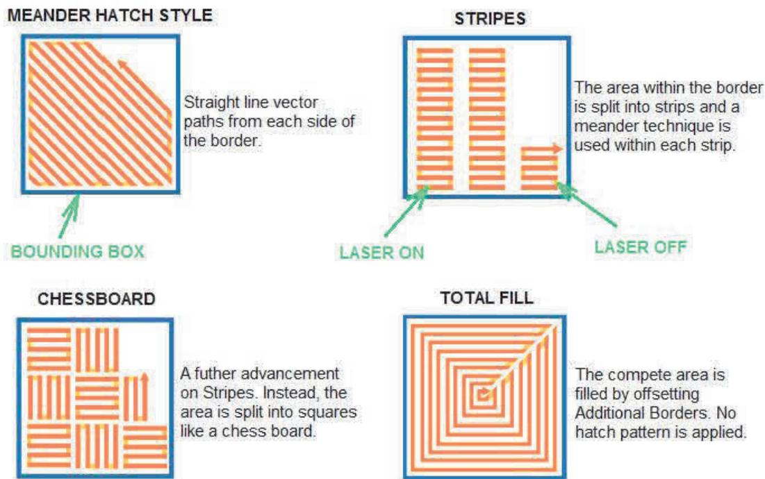
**Figure 1** Types of hatch styles [7]
