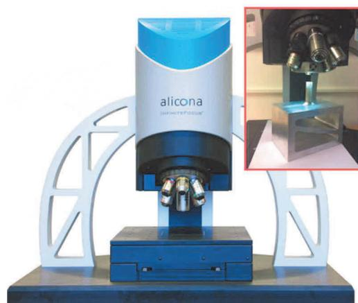
**Figure 6** Alicona Infinite Focus 5 microscope
