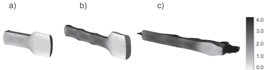
**Figure 2** Numerically estimated progression of effective strain in major forging stages (a-c)
