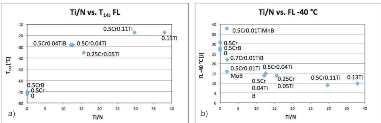
**Figure 2** a)  $T_{14J}$  transition temperatures in fusion line vs. Ti/N ratios (excluding the additional steels for which data is not available) b) Fusion line impact energies at -40 °C vs. Ti/N ratios for all the steels
