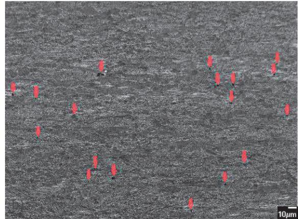
Figure 1 a) Base metal transverse transition curves b) TiN inclusions in the base metal of steel 0.13Ti
