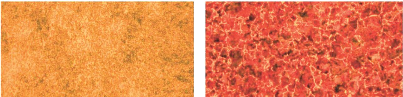
**Figure 9** The structure of the material 100Cr6 (magnification 1000:1) and C56E2 (magnification 100:1)
