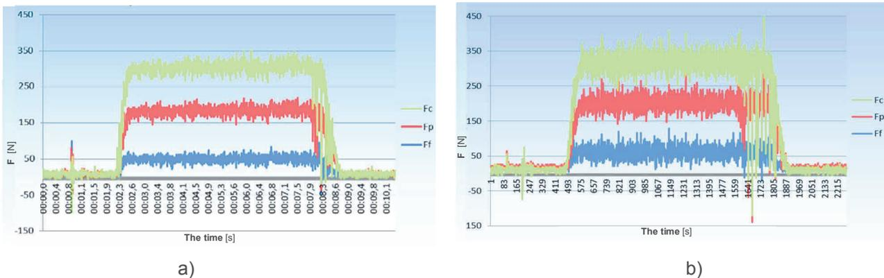
**Figure 11** The course of cutting forces during machining of material a) 100Cr6 and b) C56E2
