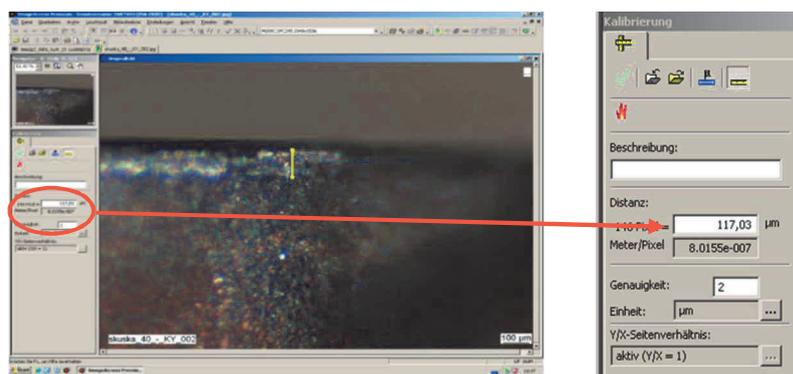
**Figure 3** Measurement of wear in the VB environment Image Access
