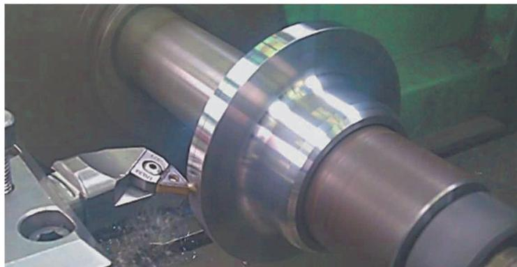
**Figure 10** The measurement of cutting forces on the flange
