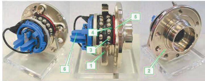
**Figure 1** The 3rd generation wheel bearing with the ABS encoder, 1- AU-outer ring, 2 - FL - flange on which is attached the wheel, 3 - ball, 4 - cage, 5 - the seal, 6 - ABS encoder power [8]
