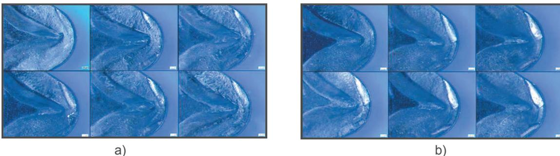
**Figure 4** Progressive wear of cutting plate of material a) 100Cr6 and b) C56E2
