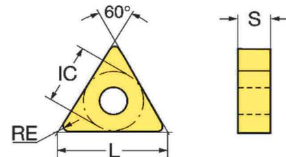
**Figure 2** Dimension triangular cutting plates
