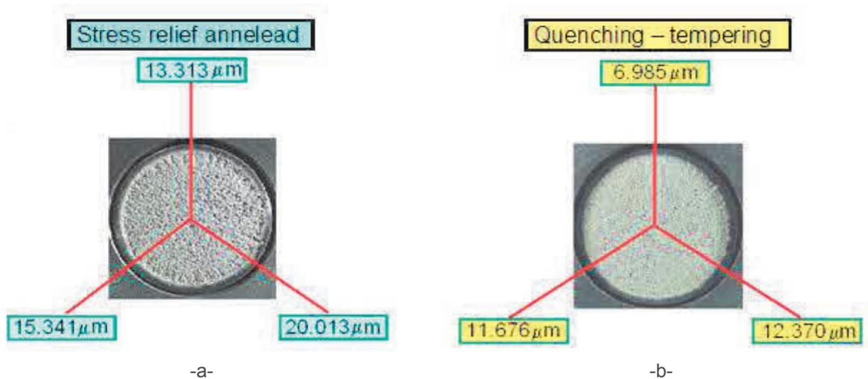
**Figure 7** Roughness values on the three measuring directions for the two structural states:
