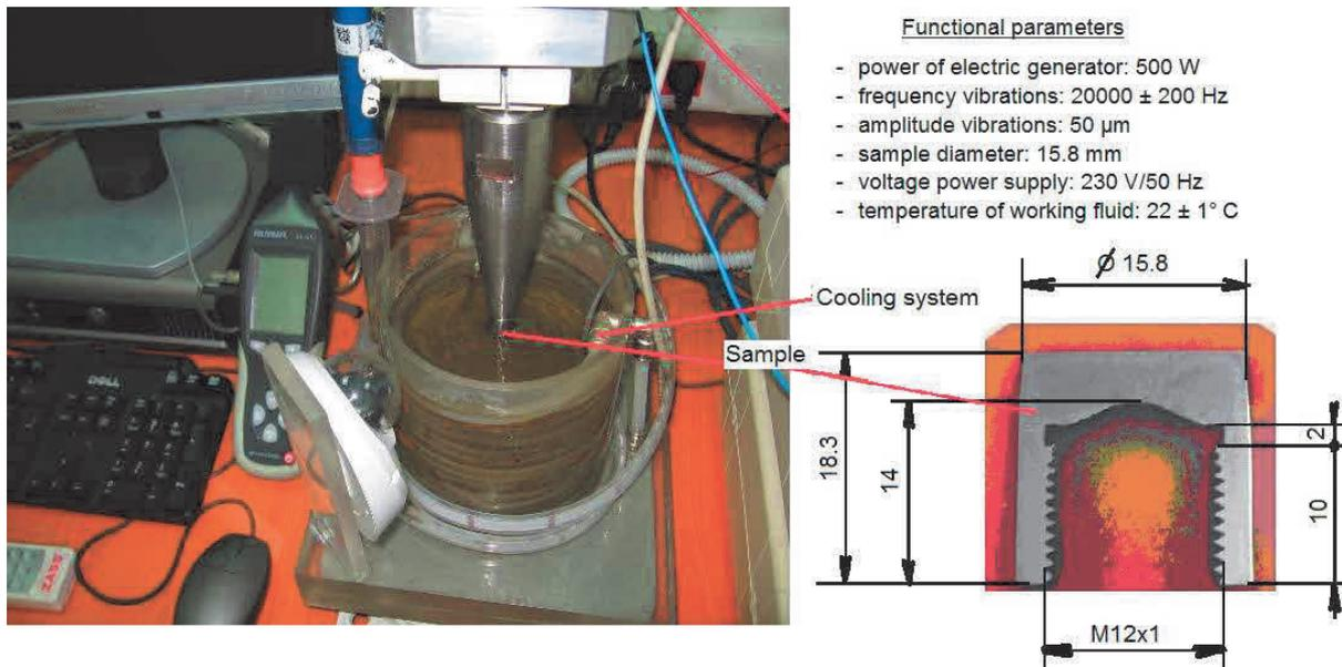
Figure 2 Overview of the vibrating apparatus with piezo-ceramic crystals
