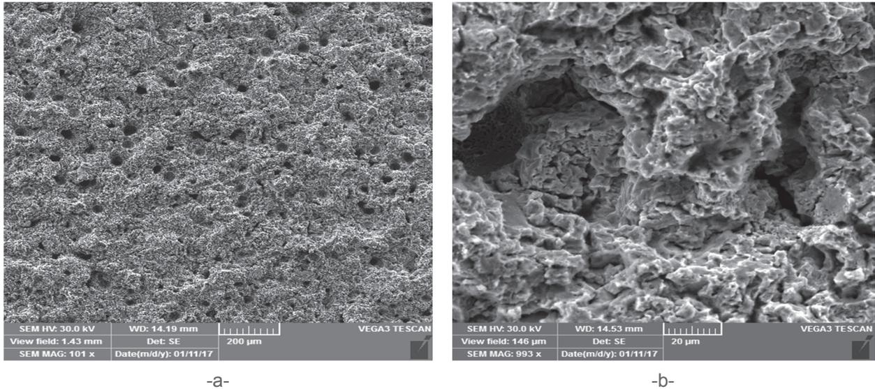
**Figure 5** SEM image of the eroded quenched - tempered surface after 165 minute cavitation time: a - material pinching; b - micro-cracks coalescence and formation of a micro tunnel
