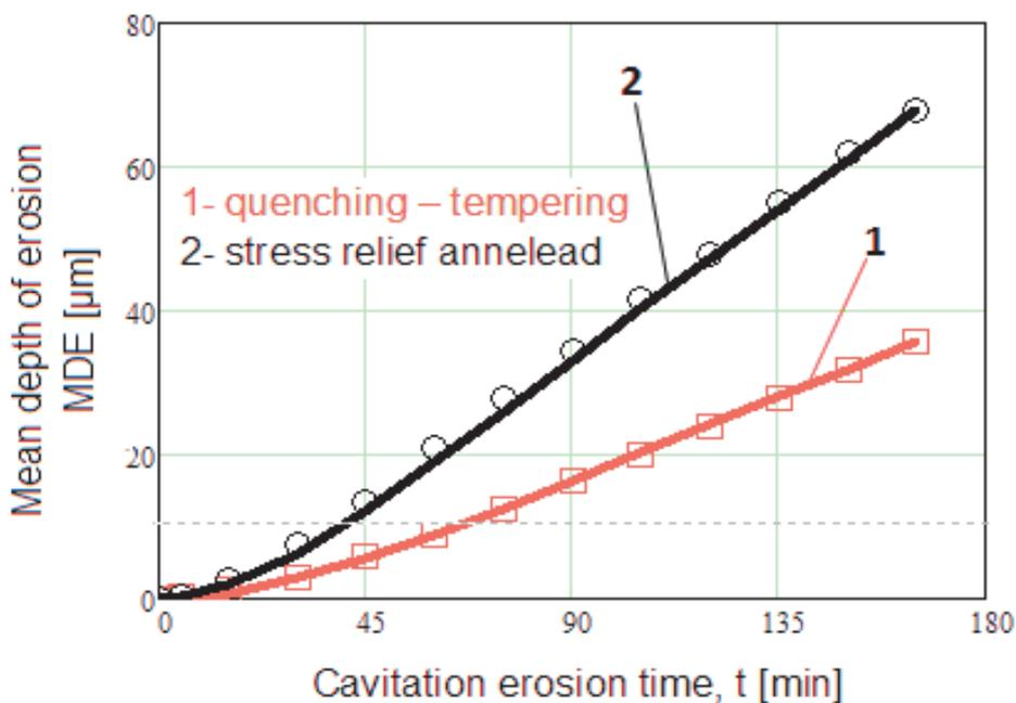
**Figure 3** Variation of the mean depth erosion penetration with the attack cavitation duration: 1 - quenching-tempering heat treatment; 2 - stress relief annealing
