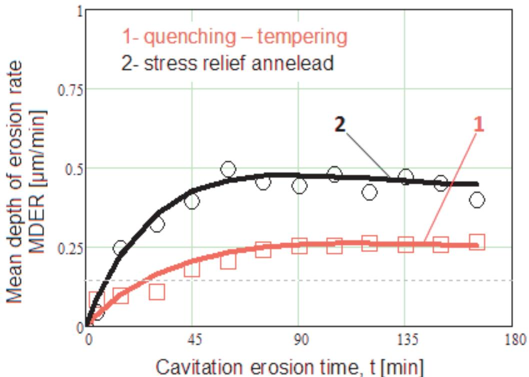
**Figure 4** Variation of the mean depth erosion penetration with the attack cavitation duration: 1 - quenching-tempering heat treatment; 2 - stress relief annealing
