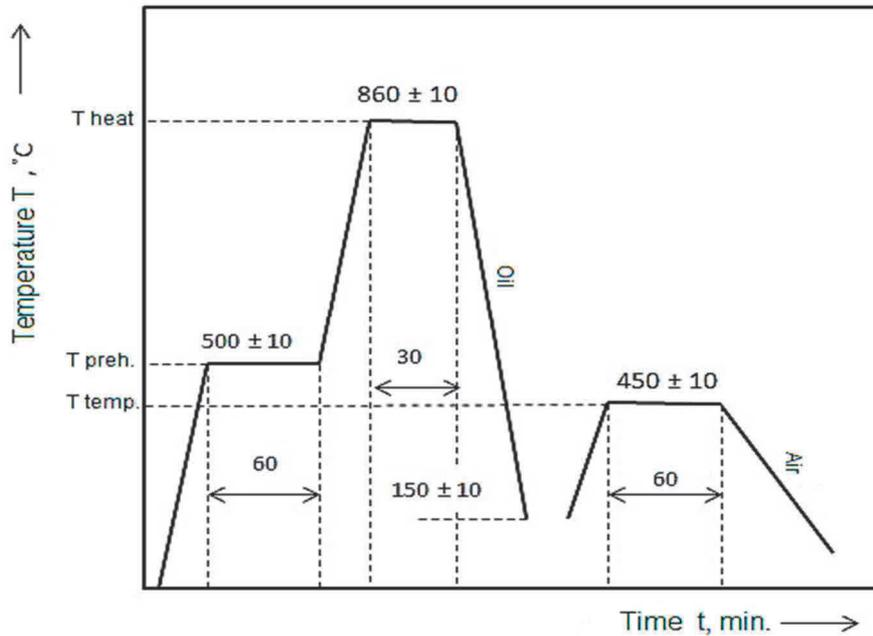
Figure 1 Heat Treatment Cyclogram of Quenching - Tempering
