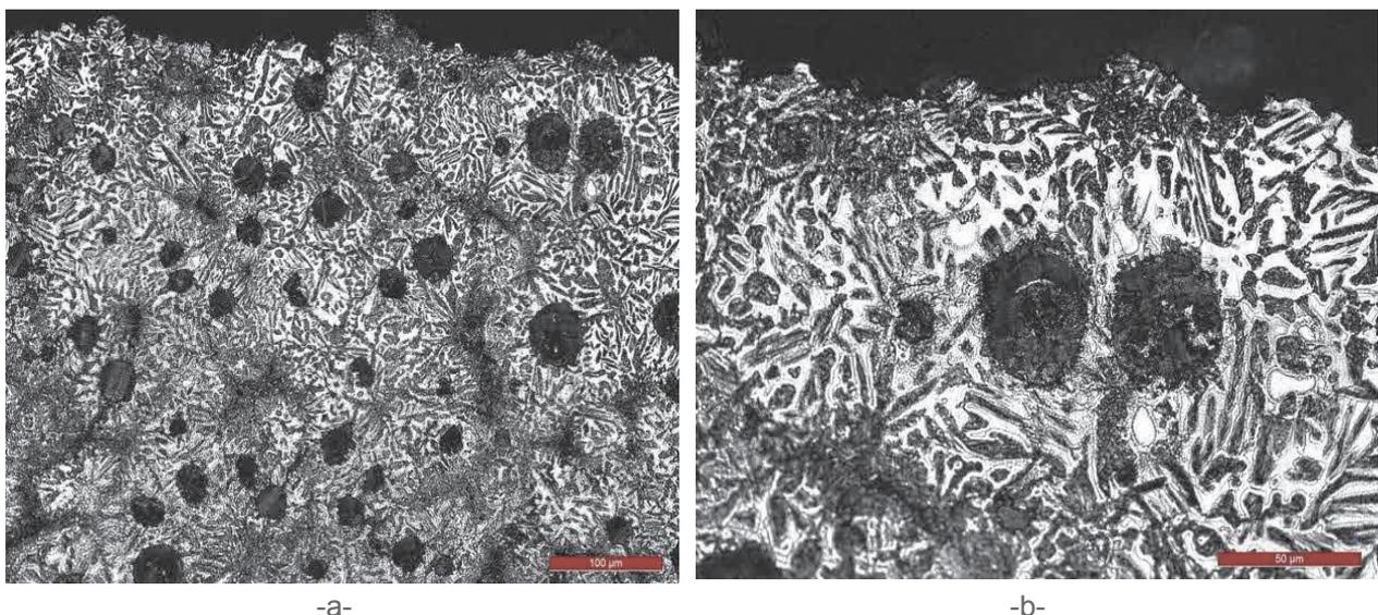
**Figure 6** Optical image of the longitudinal section through the eroded quenched - tempered samples tested for 165 min
