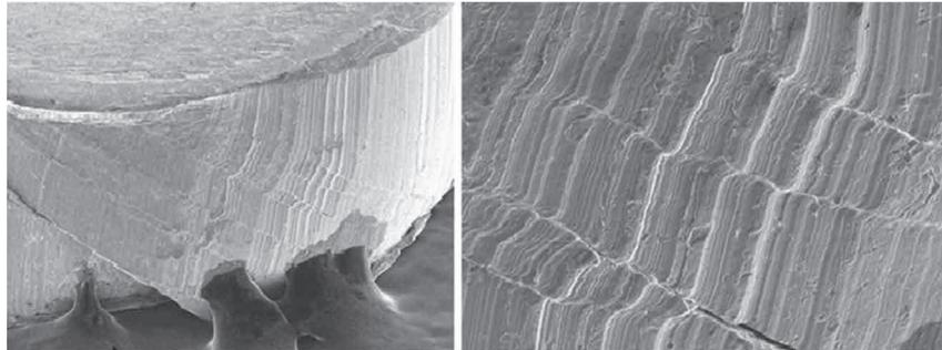
**Figure 7** SEM close ups of specimen (b) after ultrasonic assisted upsetting - PP amplitude 8.4  $\mu\text{m}$
