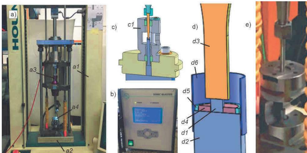
**Figure 1** Experimental set-up: a) overview, b) sonic blaster, c) micro-set with counter punch, d) close-up of plastic deformation zone - further described, e) overview of micro-set
