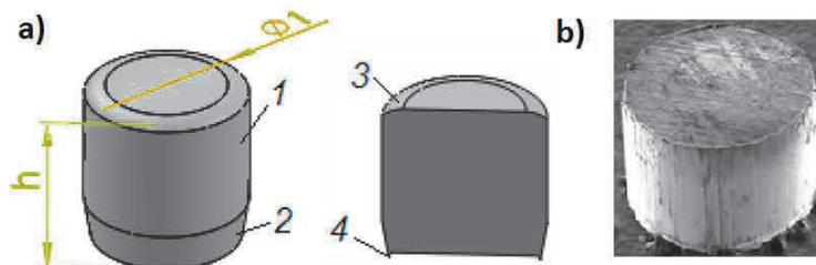
**Figure 4** Test sample: a) sample pattern after micro-punching, 1 - glossy surface, 2 - crack surface, 3 - radius, 4 - burr, b) SEM of example specimen
