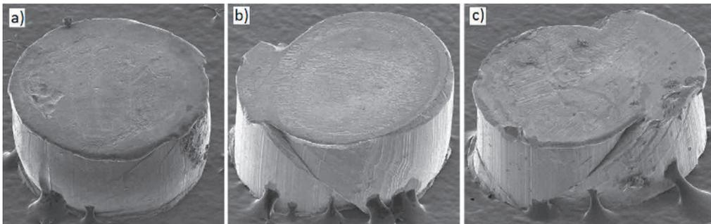
**Figure 6** SEM of specimens (a), (b) and (c) after ultrasonic assisted upsetting - see **Table 1**
