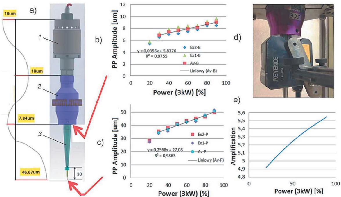
**Figure 3** Testing of ultrasonic system: a) example of amplitude distribution along the axis of US-head, b) amplitude on a bustler surface, c) amplitude on a punch nose, d) overview of a High-Speed/High-Accuracy Laser Displacement Transducer, e) Amplification factor as a function of applied power
