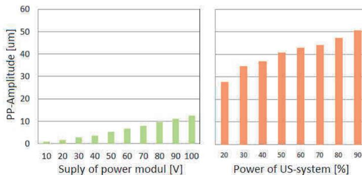
**Figure 2** Tested performance of ultrasonic system: peak to peak (PP) amplitude on the punch nose - free oscillation
