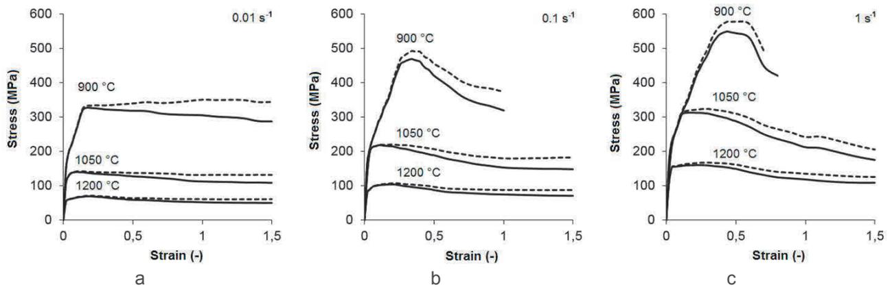
**Figure 1** Corrected (dash line) and measured (solid line) stress-strain curves of the alloy
