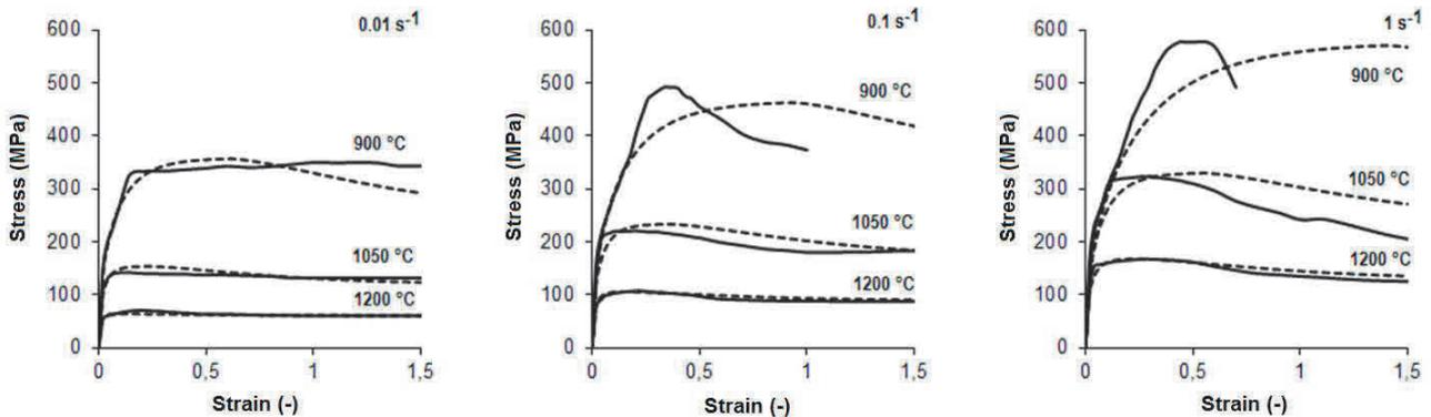
**Figure 2** Predicted (dash line) and actual (solid line) stress-strain curves of the alloy
