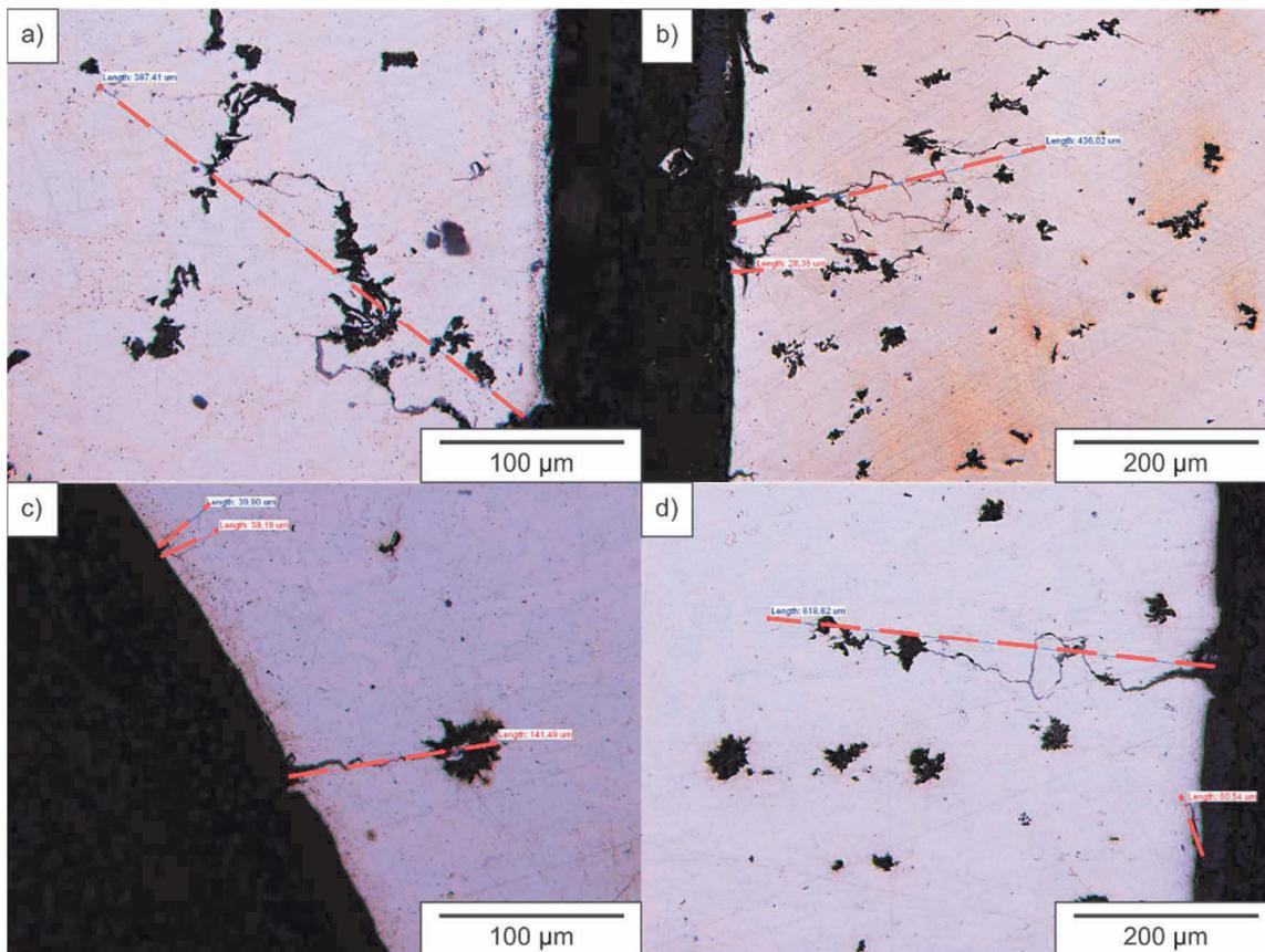
**Figure 2** Optical microphotographs of cracks formed during thermal fatigue investigation; a), b) standard ICDP - CIN; c), d) modified ICDP - CINA
