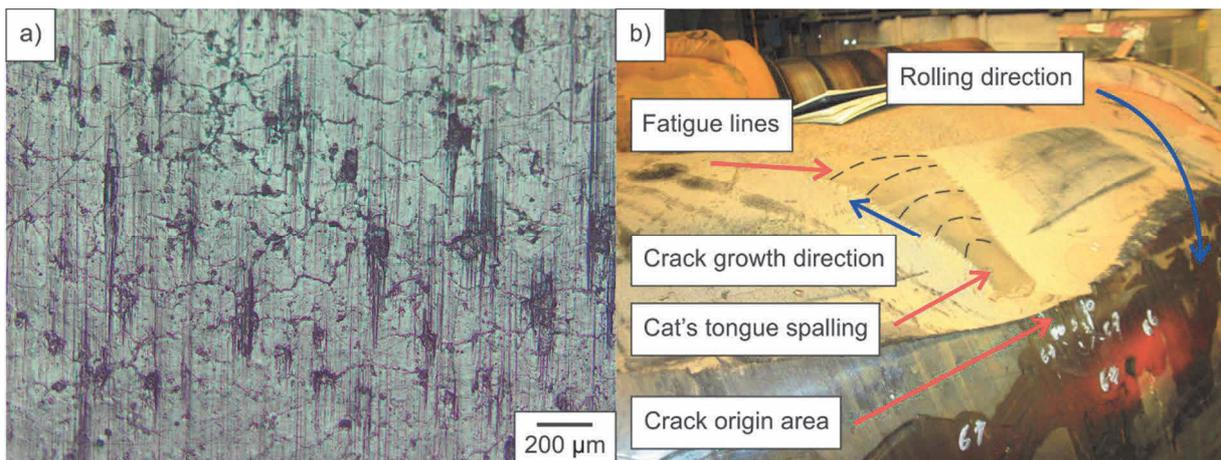
**Figure 3** Analyses of CINA work roll surface; a) a silicon replica of the CINA roll surface after exploitation; b) appearance of the cat's tongue on the spalled surface of the CINA work roll.
