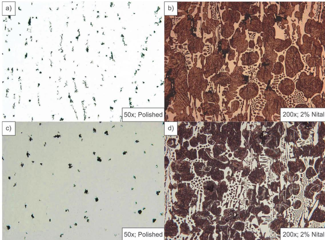
**Figure 1** Comparison between microstructures; a), b) standard ICDP - CIN, 40 mm in depth of the specimen; c), d) modified ICDP - CINA, 40 mm in depth of the specimen
