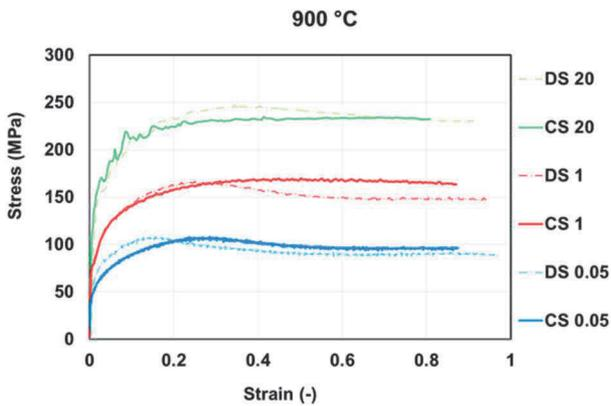
**Figure 6** Influence of strain rate on the stress curves of both structures at a temperature of 900 °C
