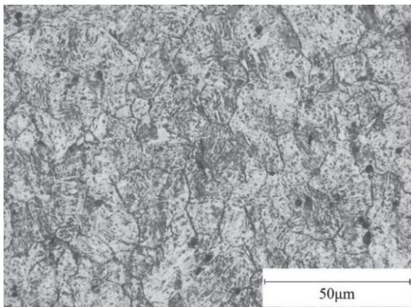
**Figure 1** Deformed state - quenching temperature 900 °C
