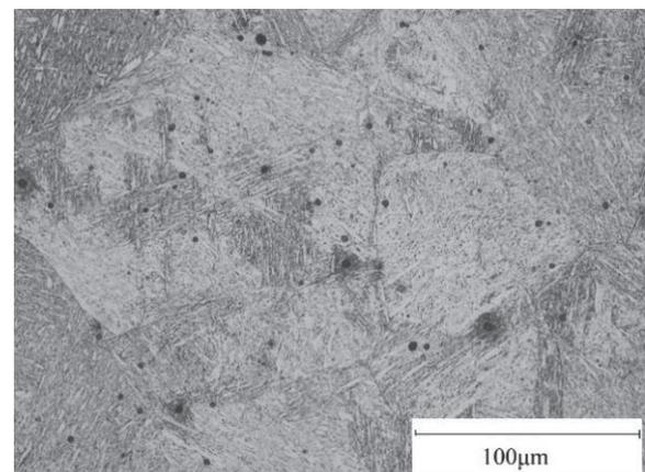
**Figure 4** Deformed state - quenching temperature 1250 °C
