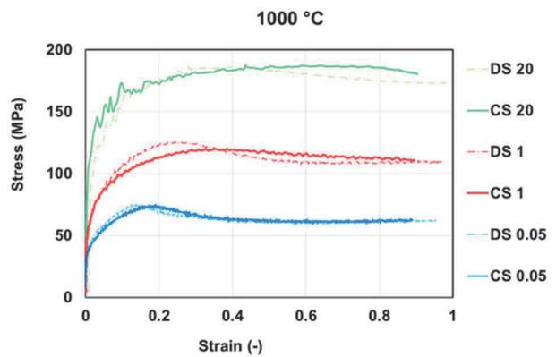
**Figure 7** Influence of strain rate on the stress curves of both structures at a temperature of 1000 °C
