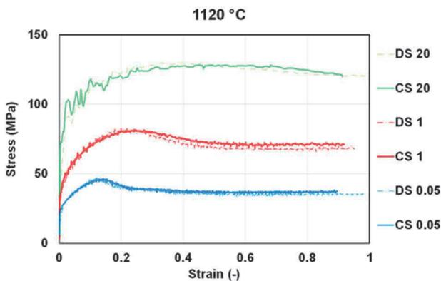
**Figure 8** Influence of strain rate on the stress curves of both structures at a temperature of 1120 °C
