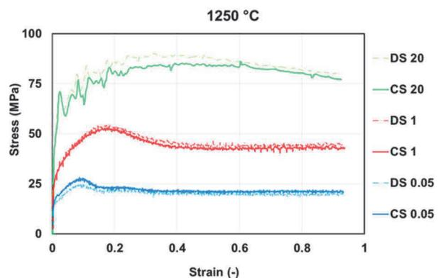
**Figure 9** Influence of strain rate on the stress curves of both structures at a temperature of 1250 °C
