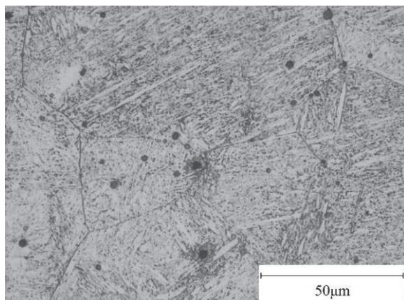
**Figure 3** Deformed state - quenching temperature 1120 °C
