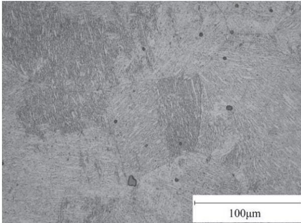
**Figure 5** Cast state - quenching temperature 1200 °C
