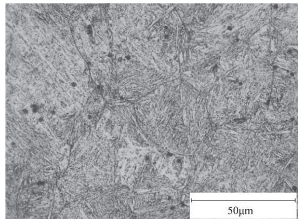
**Figure 2** Deformed state - quenching temperature 1000 °C
