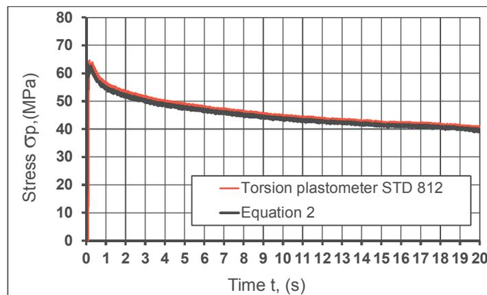
**Figure 6** The flow stress in the torsion of the 5019 aluminium alloy in the STD 812 torsion plastometer and the flow stress determined from Equation (2)
