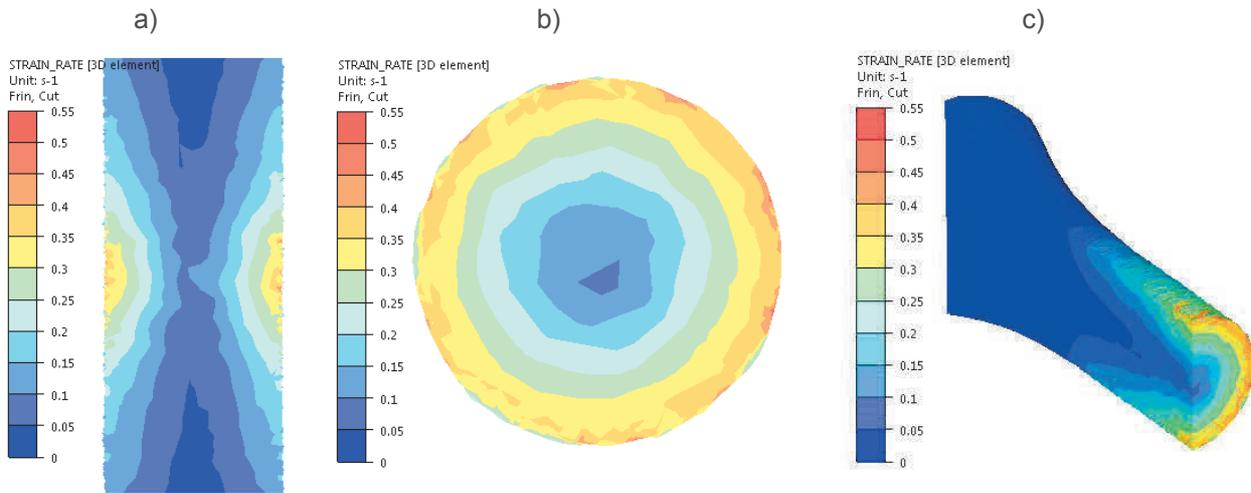
**Figure 9** Distribution of the strain rate intensity of aluminium alloy 5019 during hot torsion - temperature, 480 °C; strain rate, 0.25 s<sup>-1</sup>: a) longitudinal section; b) cross-section - the middle of the working portion; c) perspective
