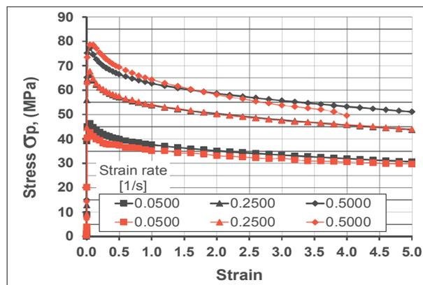
**Figure 4** The aluminium alloy flow curves: temperature, 4800 °C; red colour - plastometric test results; black colour - results after approximation
