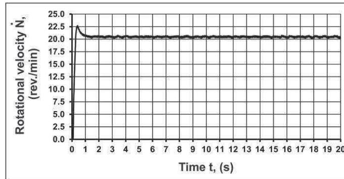
**Figure 3** Variations in the rotational speed of the STD 812 torsion plastometer motor during the torsion of 5019 aluminium alloy specimens
