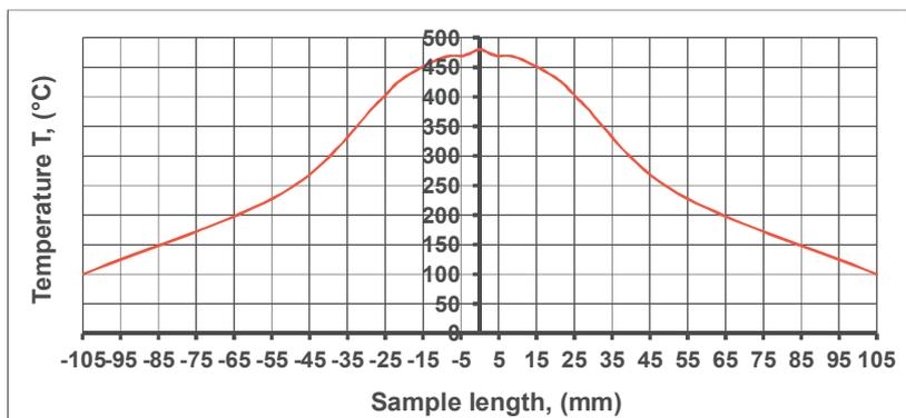
**Figure 2** The actual distribution of temperature across the length of the 5019 aluminium alloy specimen, as determined by the contact method
