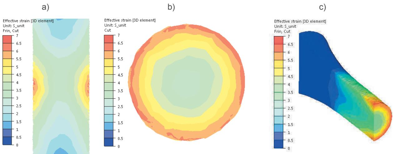
**Figure 8** Distribution of the strain intensity of aluminium alloy 5019 during hot torsion - temperature, 480 °C; strain rate, 0.25 s<sup>-1</sup>: a) longitudinal section; b) cross-section - the middle of the working portion; c) perspective
