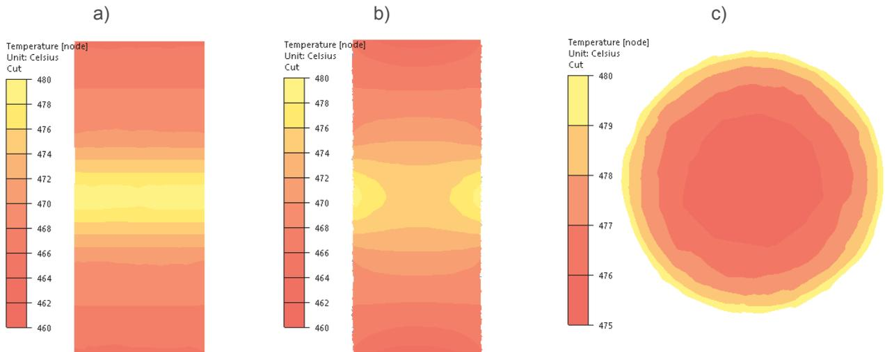
**Figure 7** Distribution of the temperature of aluminium alloy 5019 during hot torsion - temperature 480 °C; strain rate, 0.25 s<sup>-1</sup>: a) temperature distribution at the beginning of torsion - the longitudinal section; b) temperature distribution at the end of torsion - the longitudinal section; c) temperature distribution and the end of torsion - the cross-section in the middle of the specimen working portion
