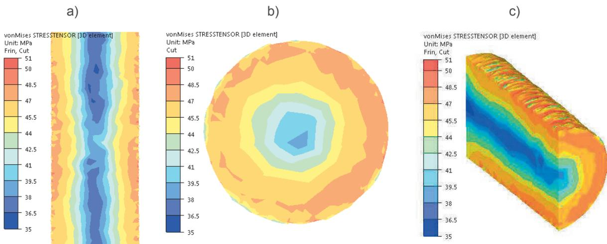
**Figure 10** Distribution of the stress intensity of aluminium alloy 5019 during hot torsion - temperature, 480 °C; strain rate, 0.25 s<sup>-1</sup>: a) longitudinal section; b) cross-section - the middle of the working portion; c) perspective
