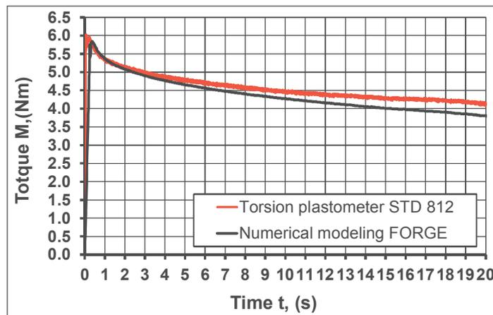
**Figure 5** The torsional moment in the torsion of the 5019 aluminium alloy in the STD 812 torsion plastometer and the torsional moment determined numerically using the Forge 2011® program
