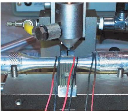
**Figure 1** A 5019 aluminium alloy specimen in a thermocouple welding machine
