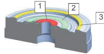
**Figure 3** Areas of analysis on the tool surface
