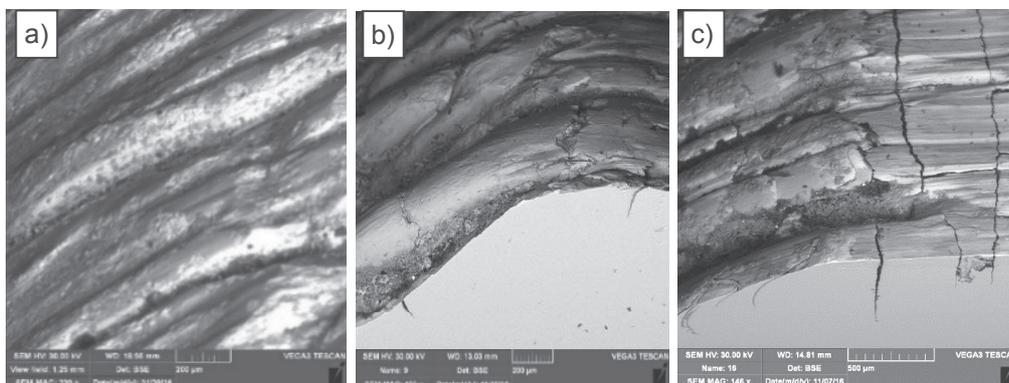
**Figure 6** SEM view of tool nitrided a) traditionally, b) by ZeroFlow variant no. 1 ( $\epsilon$ ), c) by ZeroFlow variant no. 2 ( $\gamma'$ ) in area 3 of analysis
