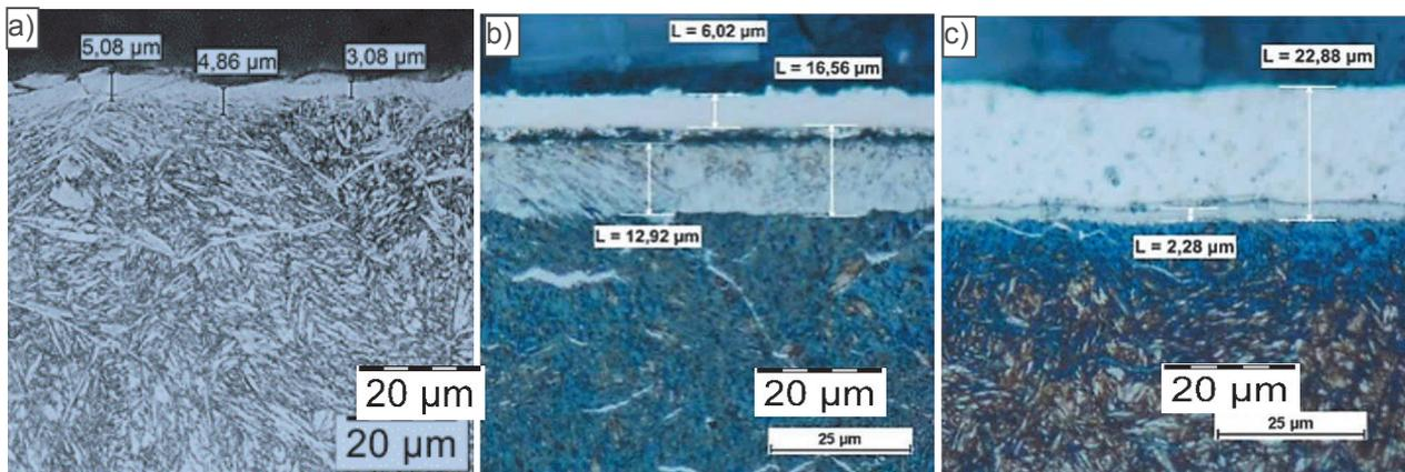
**Figure 1** View of the microstructure of the nitrided layer: a) traditional nitriding, b) ZeroFlow nitriding variant no. 1 ( $\epsilon$ ), c) ZeroFlow nitriding variant no. 2 ( $\gamma'$ )
