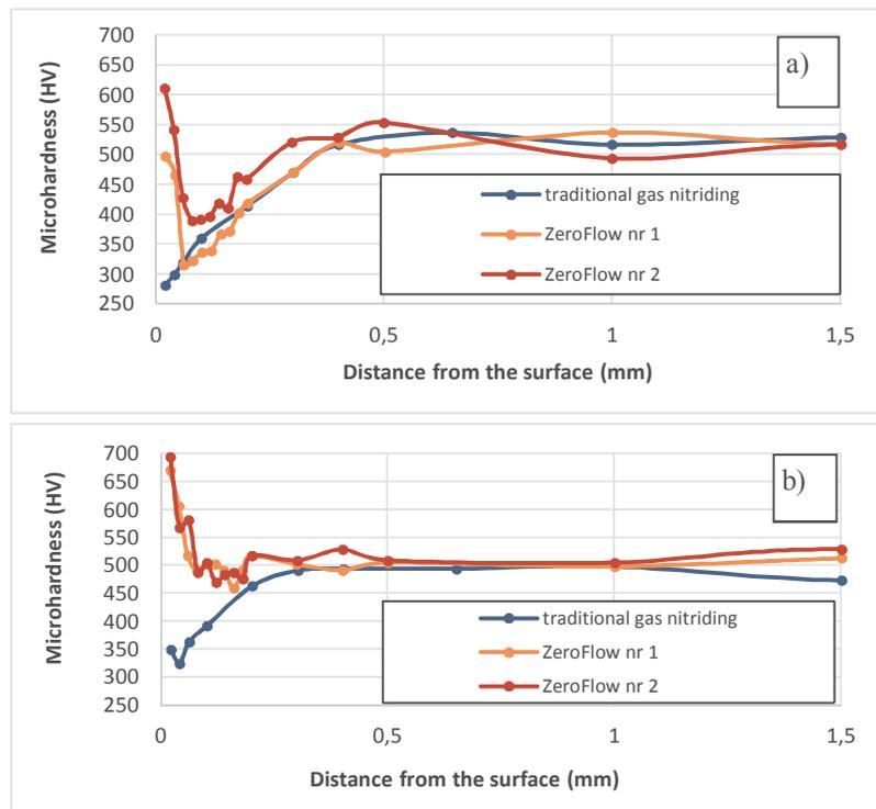
**Figure 7** Comparison of microhardness in the surface layer of tools after exploitation;
