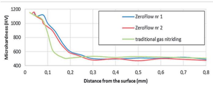
**Figure 2** Microhardness distributions determined on studied samples after nitriding
