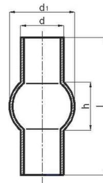
**Figure 5** Shapes and dimensions of axisymmetric component
