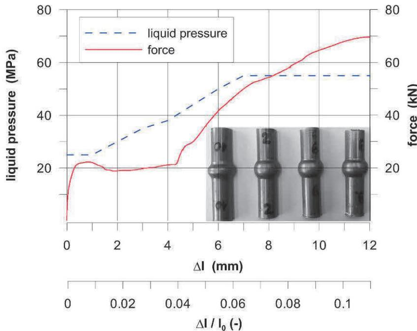
**Figure 4** Liquid pressure vs. displacement and force vs. displacement obtained for hydromechanically bulged axisymmetric components at different ratios  $\Delta l / l_0$  ( $\Delta l / l_0 = 0.054$ ;  $\Delta l / l_0 = 0.073$ ;  $\Delta l / l_0 = 0.091$  and  $\Delta l / l_0 = 0.109$ )
