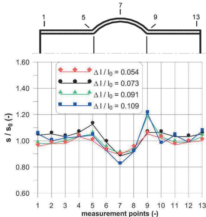
**Figure 6** The wall thickness distribution in longitudinal sections of hydromechanically bulged axisymmetric components made from copper tubes at relative ratio  $s_0 / D = 0.045$  and upsetting ratios  $\Delta l / l_0 = 0.054$ ;  $\Delta l / l_0 = 0.073$ ;  $\Delta l / l_0 = 0.091$  and  $\Delta l / l_0 = 0.109$ .
