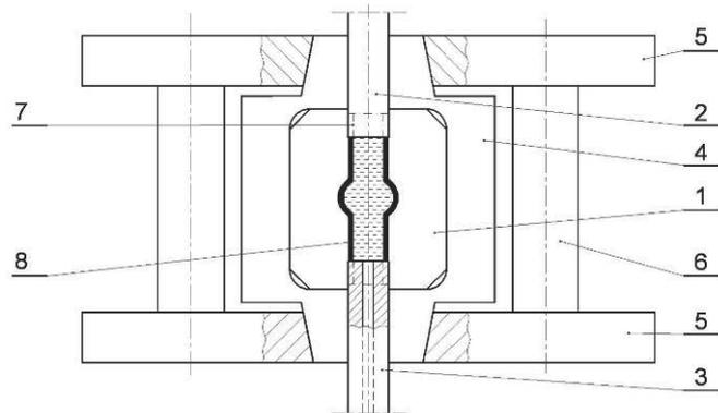
**Figure 3** Diagram of the main part of the hydromechanical bulge forming tool, where: 1- die insert, 2- upper punch, 3- lower punch, 4- half-die, 5- pressure platens, 6- guide-posts, 7- tube segment, 8- hydromechanically bulged axisymmetric component
