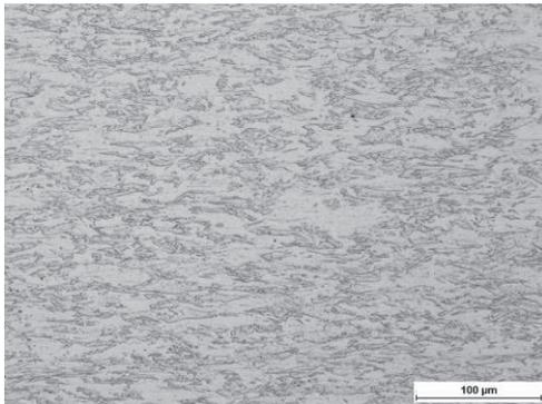
**Figure 2** The microstructure of sample of copper
