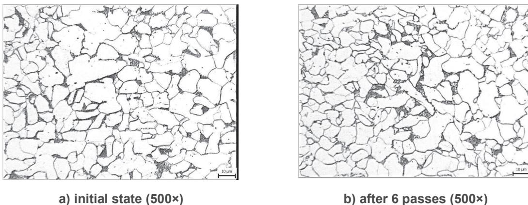
**Figure 4** Microstructure of DC 01 steel
