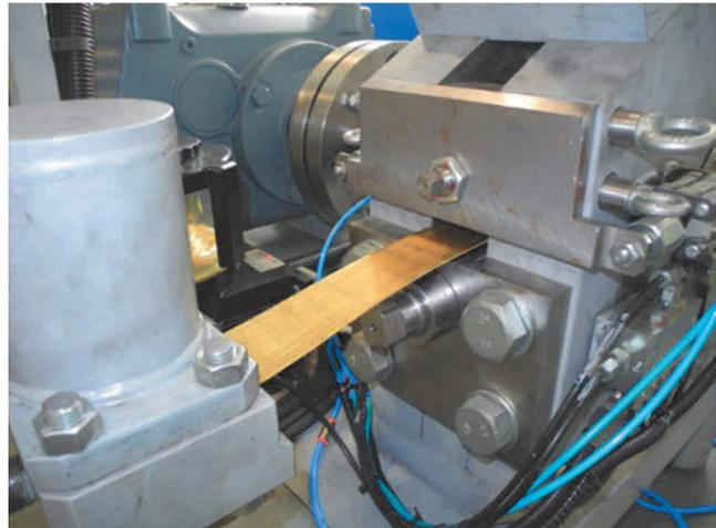
Figure 2 Forming device for extrusion of strip sheets
