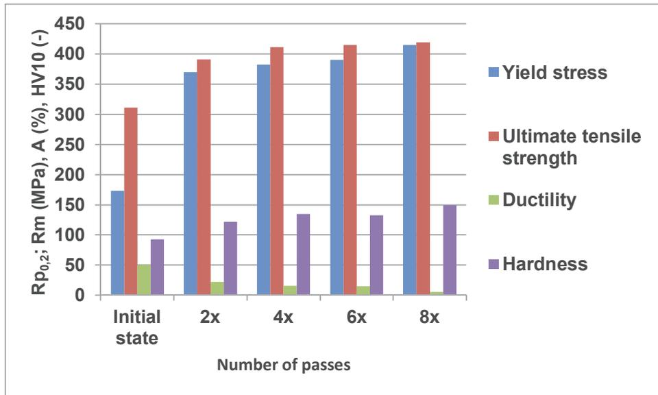
**Figure 3** Mechanical properties of DC01 steel after extrusion process
