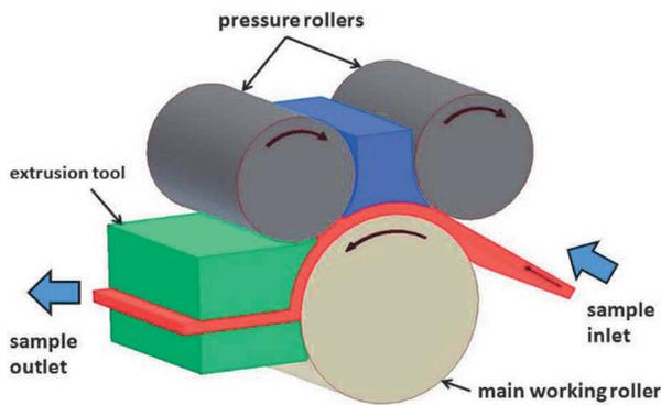
Figure 1 Scheme of DRECE method
