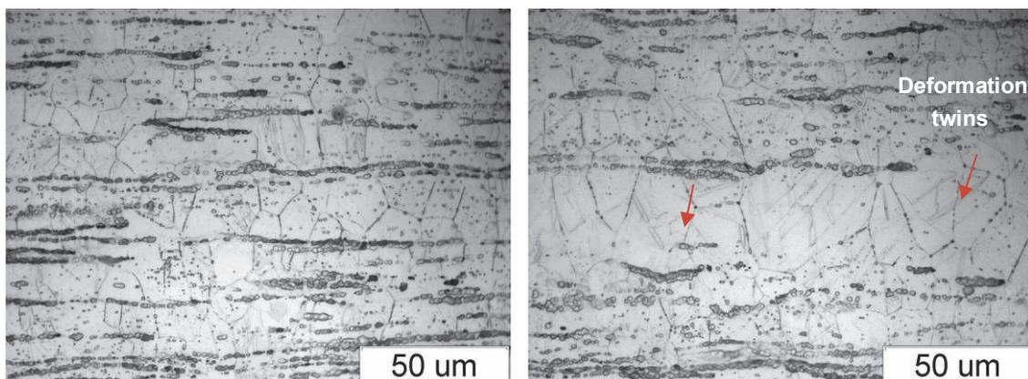
**Figure 5** Microstructure of alloy Mg-4Li-1Ca after static compression tests in room temperature
