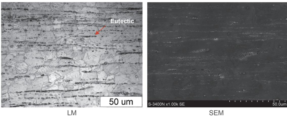
**Figure 4** Microstructure of alloy Mg-4Li-1Ca after process of extrusion
