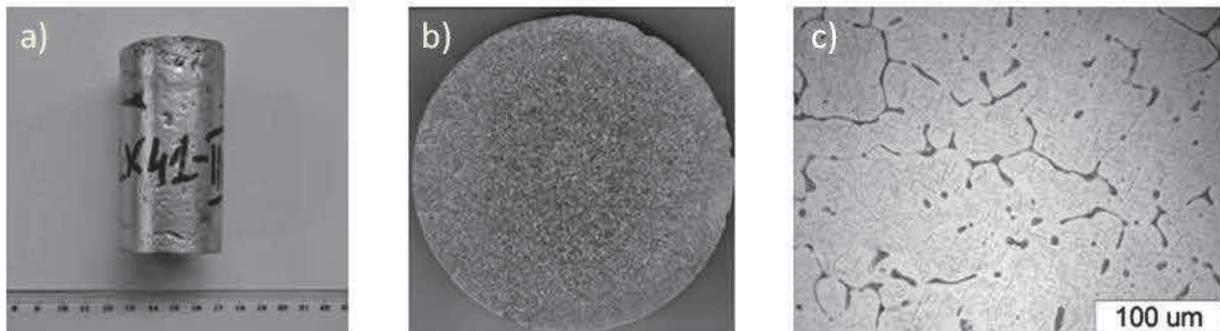
**Figure 1** Alloy Mg-4Li-1Ca after casting process: a) the appearance of the ingot, b-c) macrostructure
