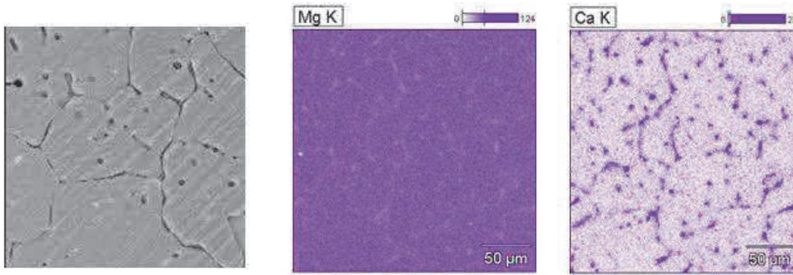
**Figure 3** Surface distribution of elements Mg, Ca in alloy Mg-4Li-1Ca after processes of casting and homogenisation
