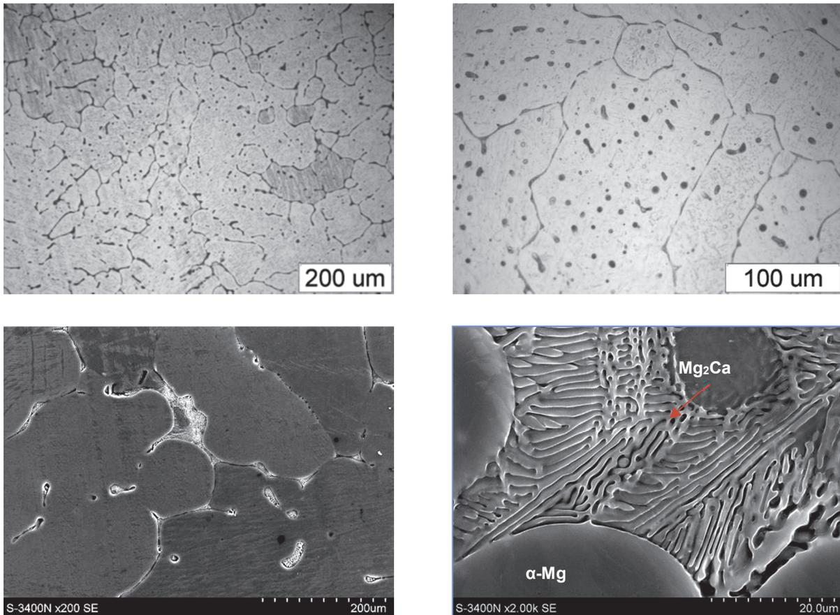
**Figure 2** Microstructure of alloy Mg-4Li-1Ca after casting and homogenisation, visible eutectics with lamellar structure in inter- dendritic areas
