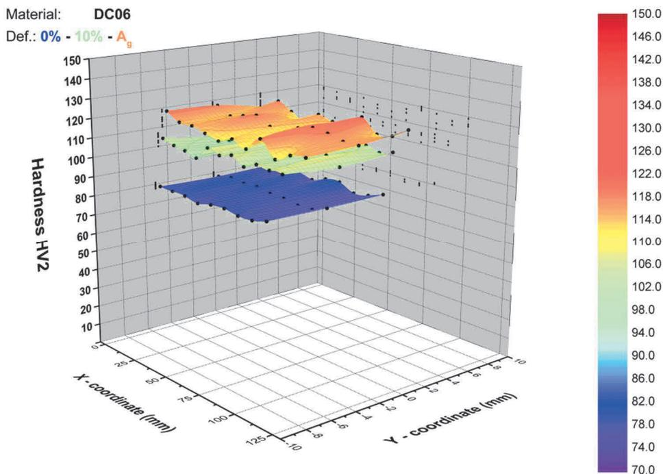
Figure 5 DC06 - 3D color maps surfaces for 1<sup>st</sup> three applied engineering strains: 0 % - 10 % -  $A_g$  (25 %)
