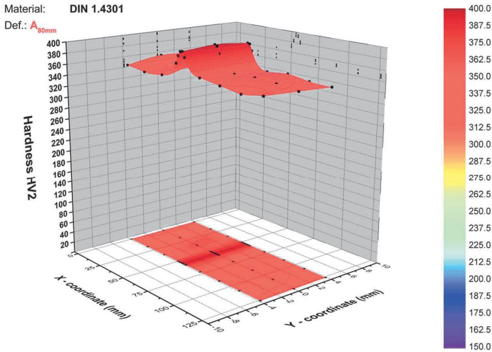
**Figure 8** DIN 1.4301 - 3D color map surface for the last applied engineering strain:  $A_{80mm}$  (54 %)
