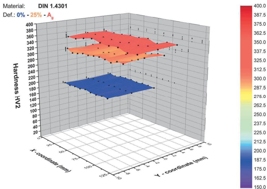
**Figure 7** DIN 1.4301 - 3D color maps surfaces for 1<sup>st</sup> three applied engineering strains: 0% - 25% -  $A_g$  (51%)
