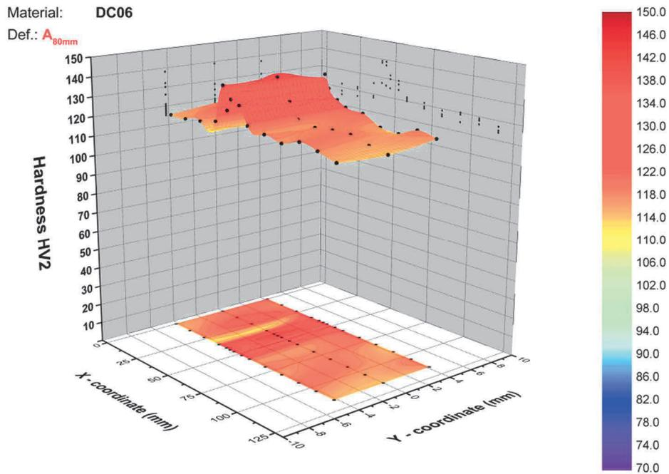
**Figure 6** DC06 - 3D color map surface for the last applied engineering strain:  $A_{80mm}$  (45 %)
