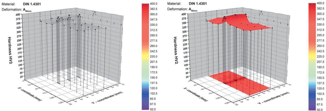
Figure 4 3D color map surface only as a mesh through measured points (left) and filled by color map (right)
