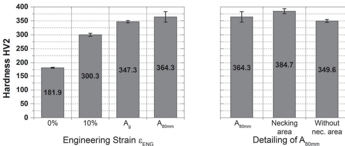
**Figure 10** DIN 1.4301 - hardness HV2 vs. engineering strain and its detailing for  $A_{80mm}$
