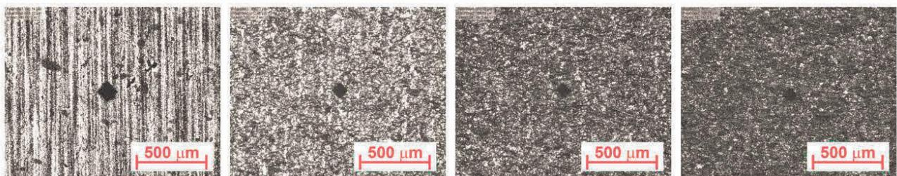
**Figure 3** DIN 1.4301 - hardness HV2 images in dependence on engineering strain: 0 % - 25 % -  $A_g$  -  $A_{80mm}$
