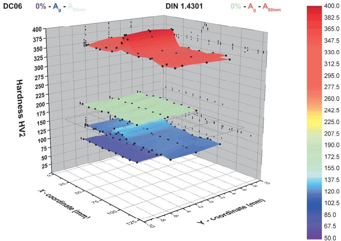
**Figure 11** Final comparison of hardness distribution for both tested materials (separated by plain grey mesh)
