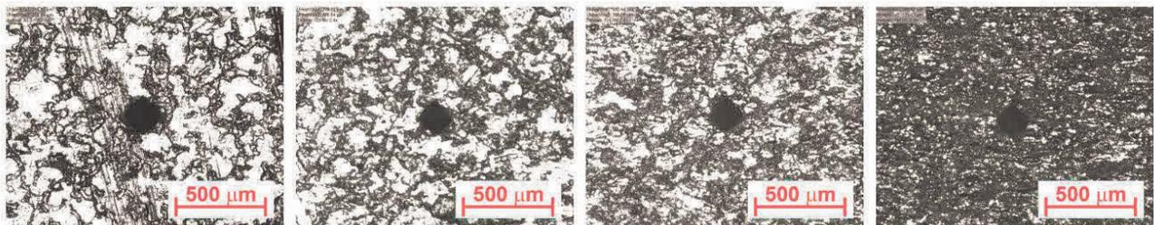
**Figure 2** DC06 - hardness HV2 images in dependence on engineering strain: 0 % - 10 % -  $A_g$  -  $A_{80mm}$
