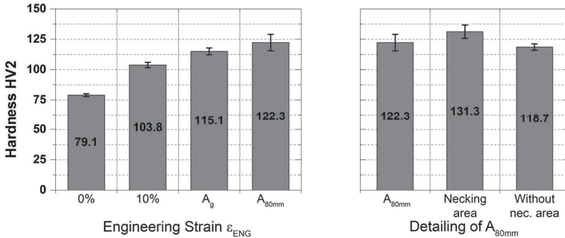
**Figure 9** DC06 - hardness HV2 vs. engineering strain and its detailing for  $A_{80mm}$
