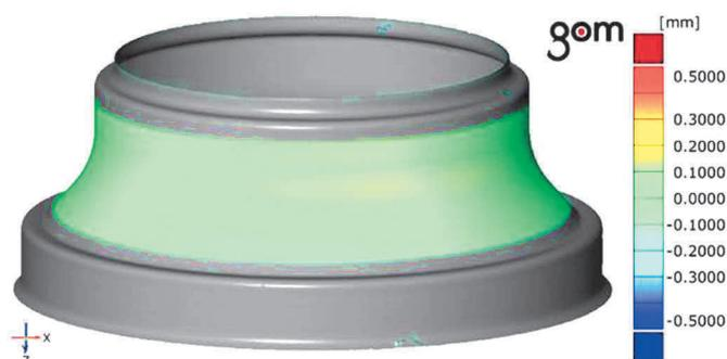
**Figure 5** The distribution of the shape error obtained using the GOM ATOS Core instrument
