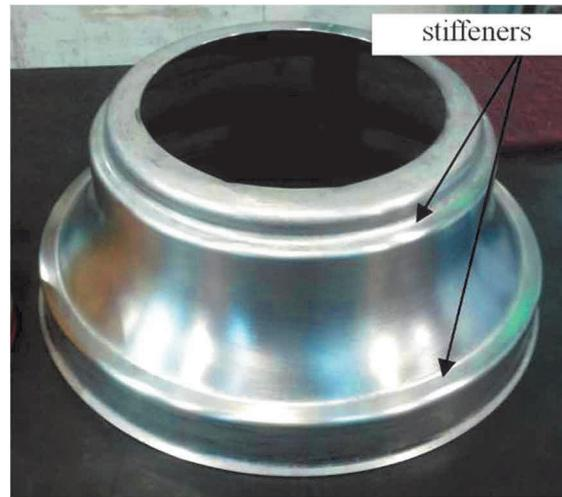
**Figure 3** The fan engine bearing housing element
