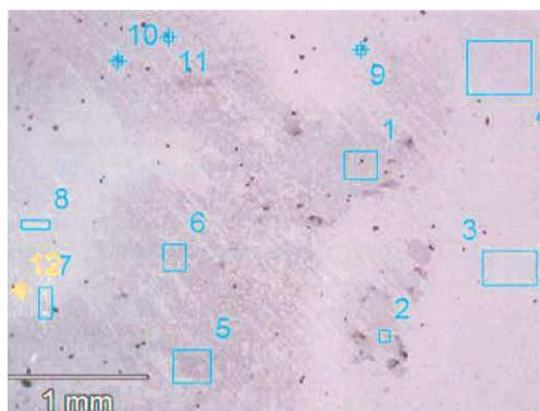
**Figure 7** View of the surface of the drawpiece with marked areas where the SEM EDS analysis was carried out
