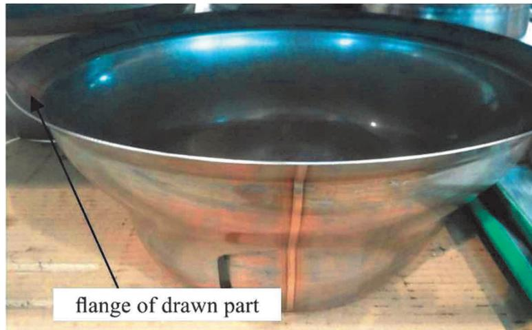
**Figure 4** The shape of the drawpiece after the first forming stage
