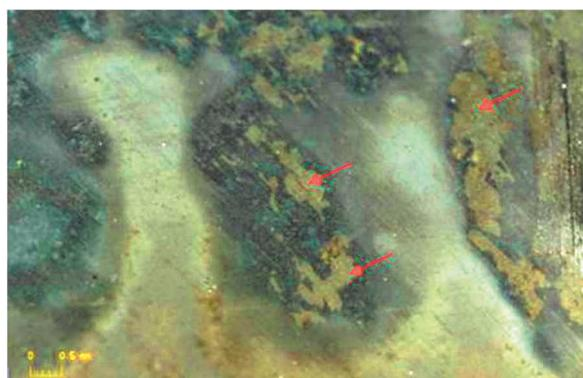
**Figure 6** Stains on the drawpiece surface
