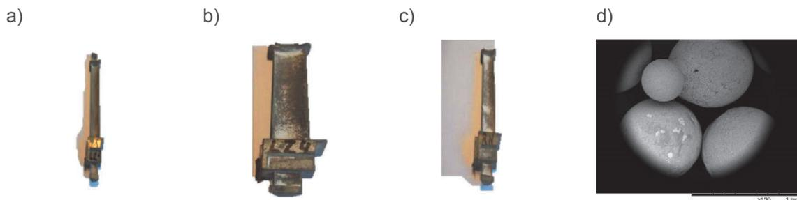
**Figure 3** Blade 1 (a), 2 (b), 3 (c) after initial shot blasting and shot (d)
