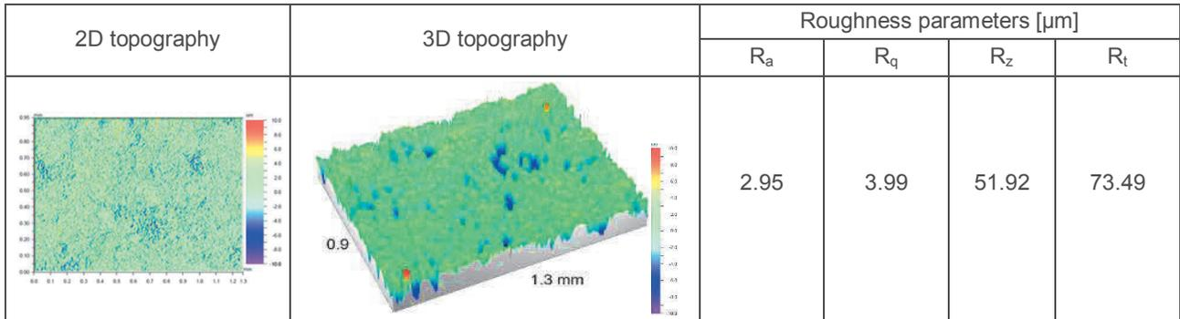
**Figure 7** Results of the roughness measurements of the wax blade model
