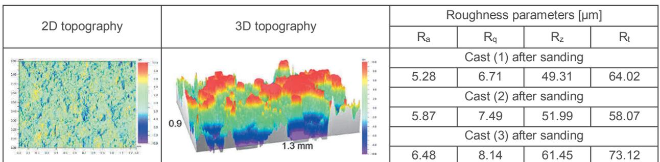
**Figure 10** Results of the roughness measurements after sanding
