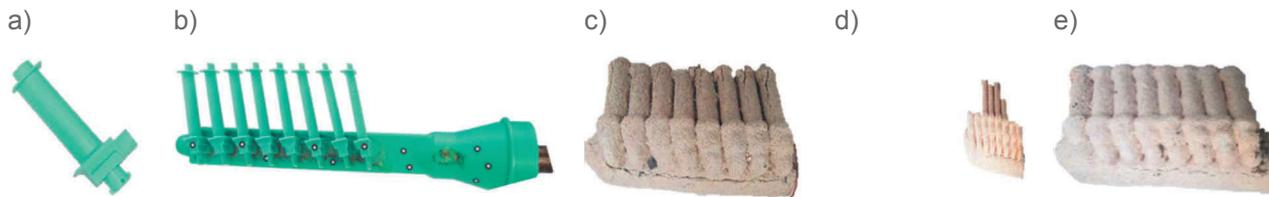
**Figure 1** Wax model of blade (a), model set (b), form 1 (c), form 2 (d), form 3 (e)
