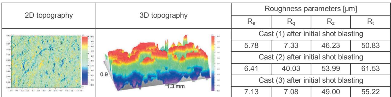
**Figure 9** Results of the roughness measurements after initial shot blasting
