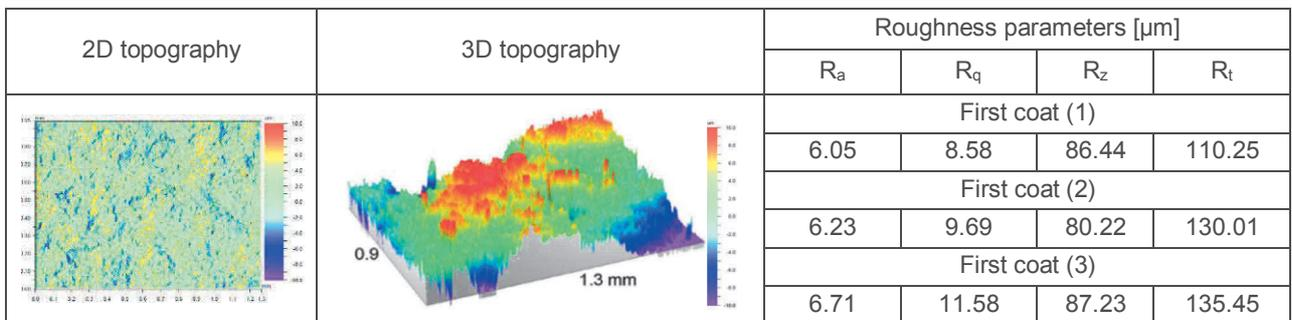
**Figure 8** Results of the roughness measurements of the first ceramic coat
