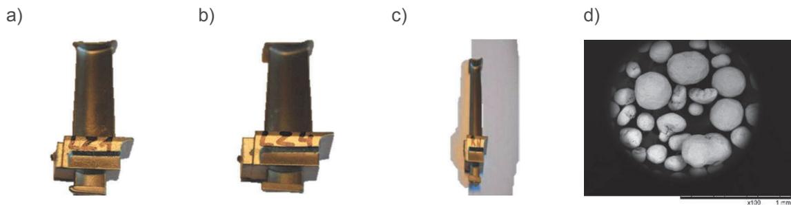
**Figure 5** Blades 1 (a), 2 (b), 3 (c) after the final blast process and chronital (d)
