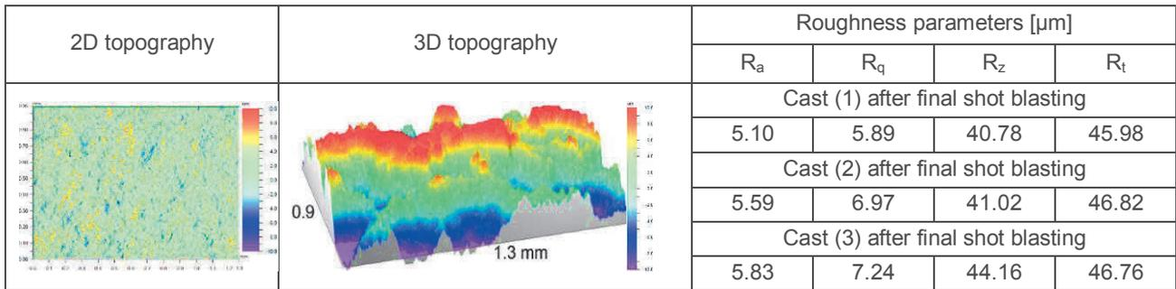
**Figure 11** Results of the roughness measurements after final shot blasting
