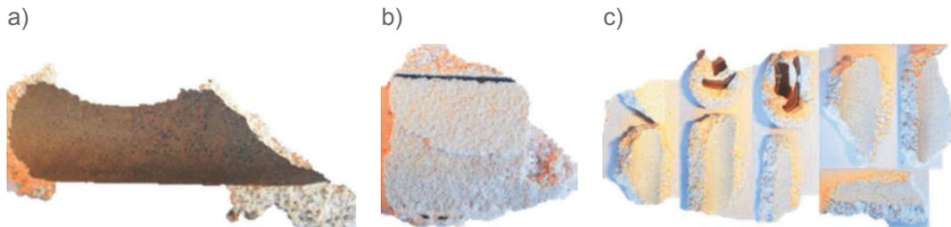
**Figure 2** Ceramic form after breaking down. A model shell (a), further molds (b-c)
