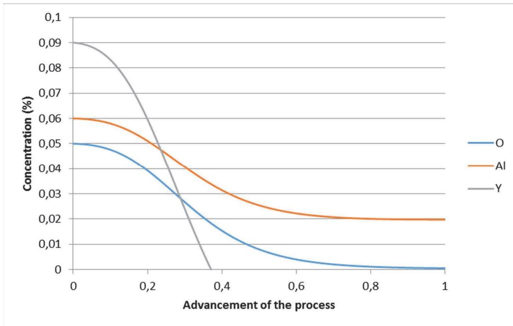
**Figure 3** Change of concentration of components in the course of growth of two-component nucleus  $\text{Al}_2\text{O}_3$   $\text{Y}_2\text{O}_3$  (for  $r_0 = 5 \mu\text{m}$ ) concentration
