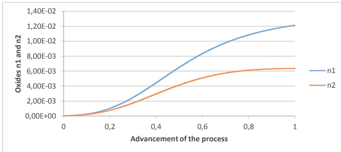
**Figure 5** Increase of two-component nuclei of oxides n1( $\text{Al}_2\text{O}_3$ ) [mole] and n2 ( $\text{Y}_2\text{O}_3$ ) [mole] (for  $r_0 = 5 \mu\text{m}$ )
