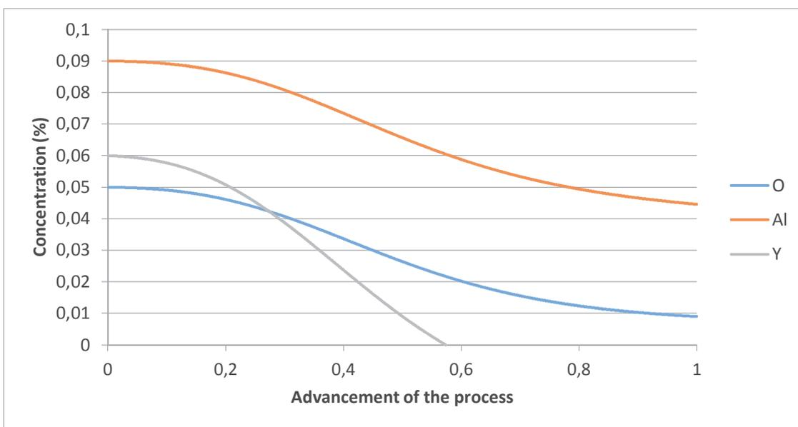
**Figure 6** Change of concentration of components in the course of growth of two-component nucleus  $\text{Al}_2\text{O}_3 \text{ Y}_2\text{O}_3$  (for  $r_0 = 5 \mu\text{m}$ )
