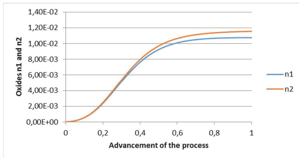
**Figure 2** Increase of two-component nuclei of oxides n1 ( $Al_2O_3$ ) [mole] and n2 ( $Y_2O_3$ ) [mole] (for  $r_0 = 5 \mu m$ )
