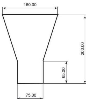
**Figure 1** Dimensions of the test ingot YIV (PN-EN 1563:2012)
