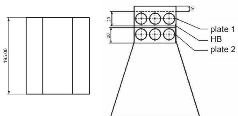
**Figure 2** Plates cutting method
