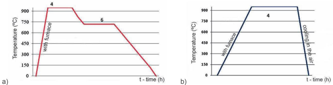
**Figure 3** Diagram of the heat treatment: a) ferritizing annealing, b) normalizing
