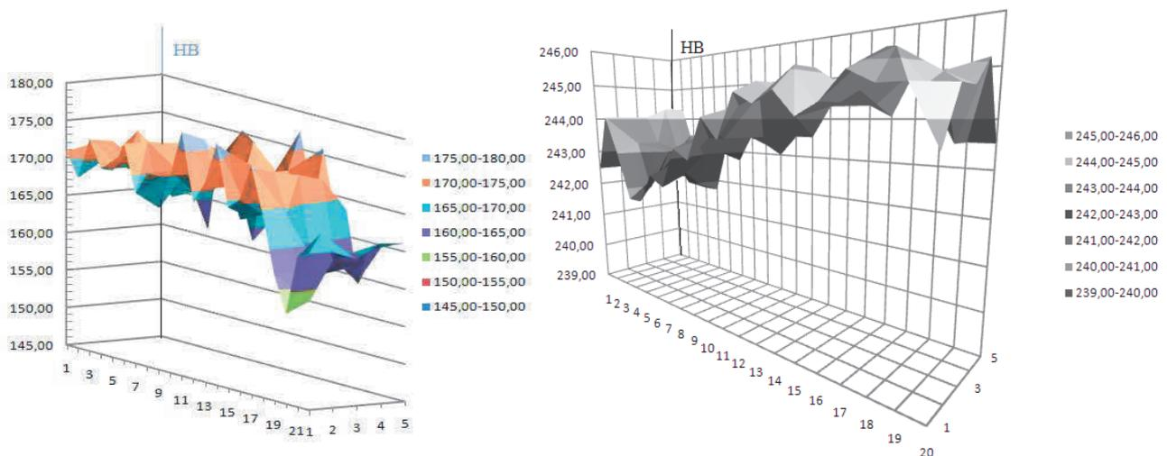
**Figure 5** Distribution of hardness after: a) casting non-alloy cast iron, b) casting copper alloy
