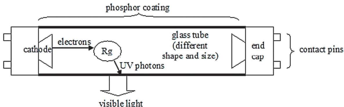
**Figure 4** The view and principle of working the fluorescent lamp [10]
