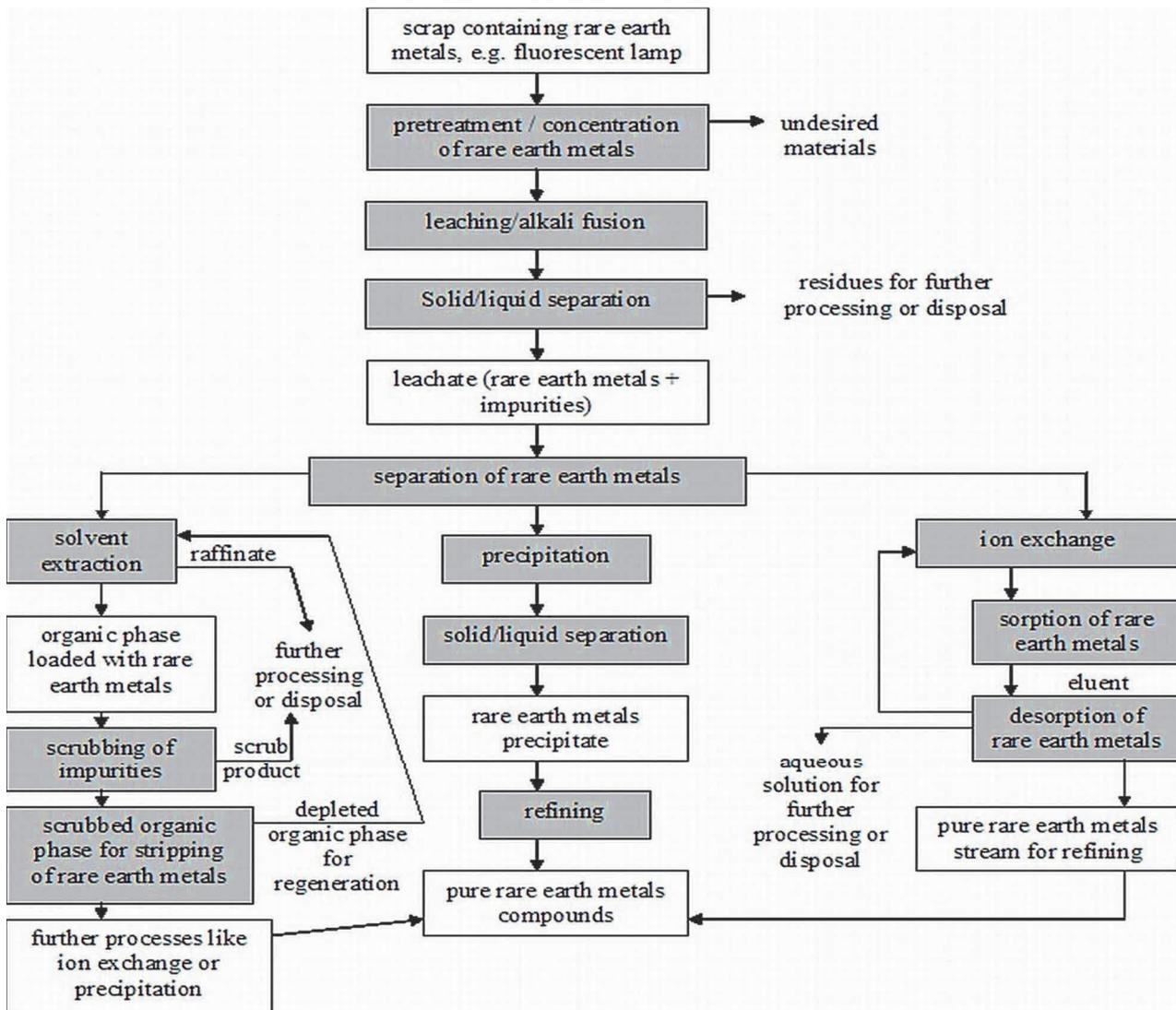
**Figure 6** The scheme of different purification processes of rare earth metals [26]
