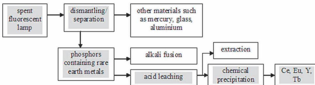
**Figure 5** The scheme of recycling process of rare earth metals [10]
