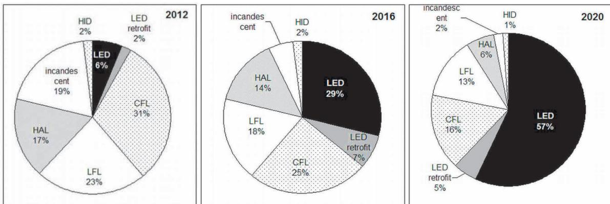
**Figure 3** Predicted values in year 2020 of global market considering different lightning technology: CFL - Compact Fluorescent Lamp, LFL - Linear Fluorescent Lamp, HAL - Halogen lamp, HID - High-intensity discharge lamp, LED - Light Emitting Diodes comparing with year 2012 and 2016 [6, 7]
