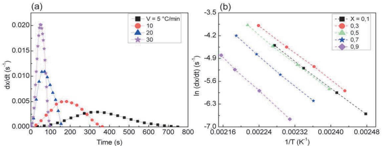
**Figure 2 a)** Rate of recrystallization process versus time, **b)** Plot of  $\ln (dX/dt)$  versus  $1/T$  of Mg-1.44 wt.% Ce alloy processed by HPT to 1/2 turn
