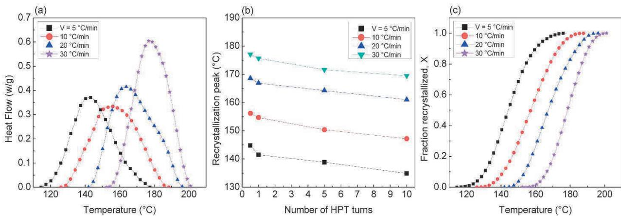
**Figure 1 a)** DSC curves of an exothermic peak records to the recrystallization process of Mg-1.44 wt.% Ce alloy processed by HPT to 1/2 turn; **b)** Evolution of recrystallization temperature peak of Mg-1.44 wt.% Ce as function of number of HPT turns; **c)** Fraction recrystallized, X versus temperature of Mg-1.44 wt.% Ce alloy processed by HPT to 1/2 turn
