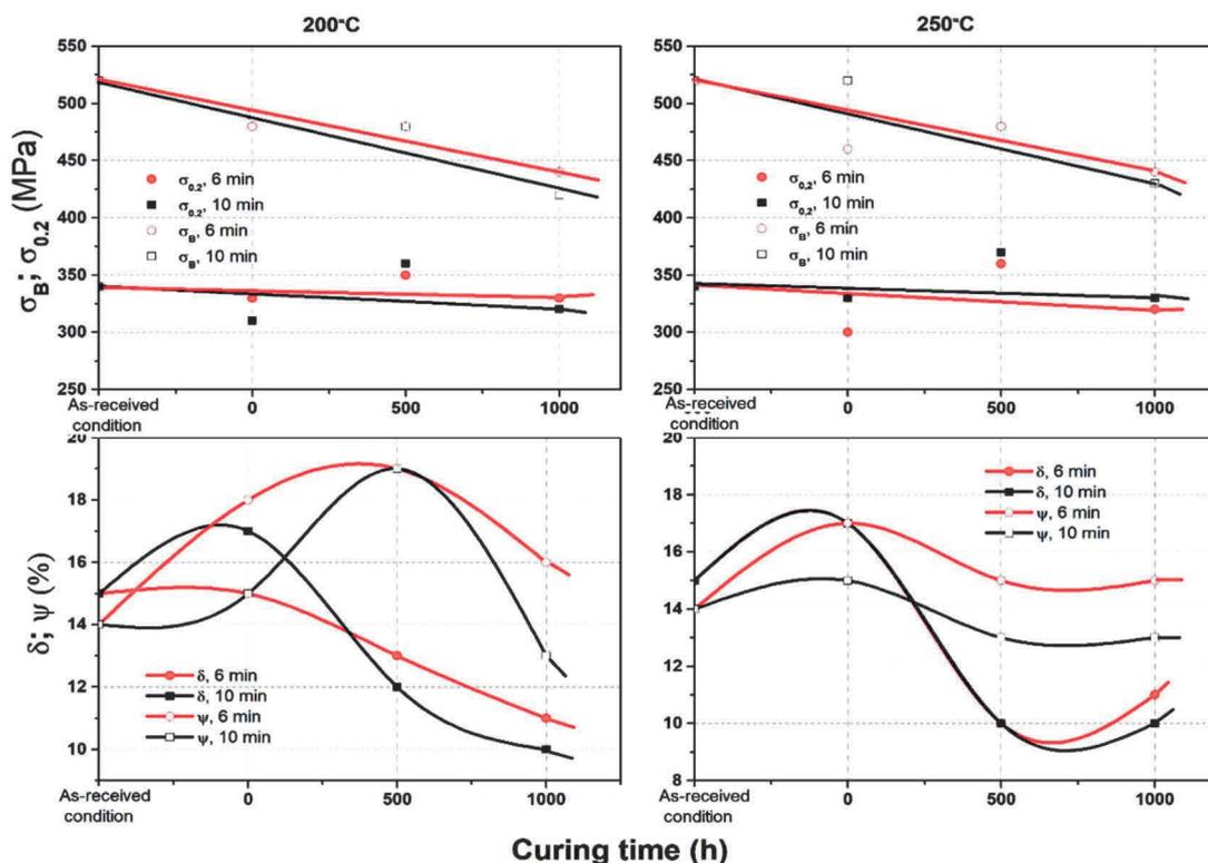
**Figure 2** The effect of operating exposure duration at 150 °C on the mechanical properties of 2024 alloy after preliminary heating ("0" point) to 200 - 250 °C with the exposure of 6-10 min
