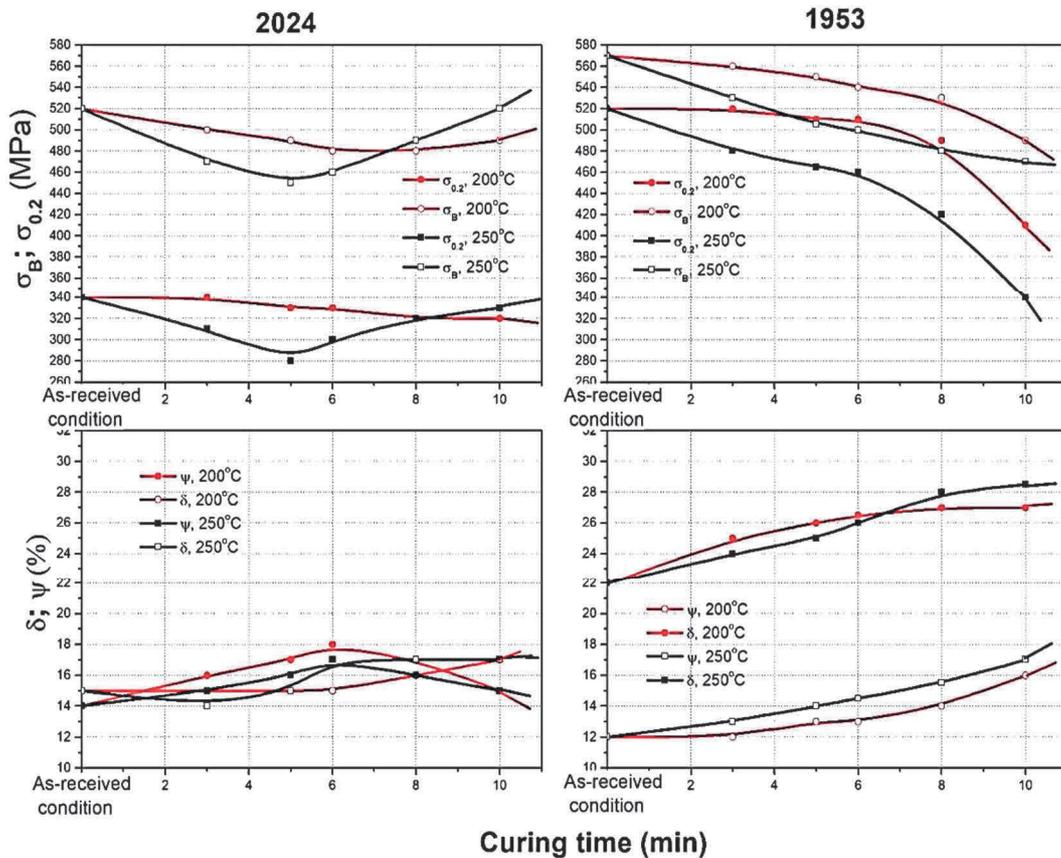
**Figure 1** Technological heating duration and temperature effect on the mechanical properties of 2024 and 1953 alloys
