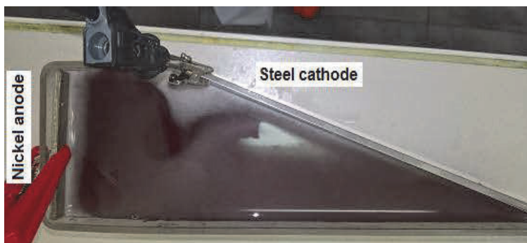
Figure 3 View showing the Hull cell
