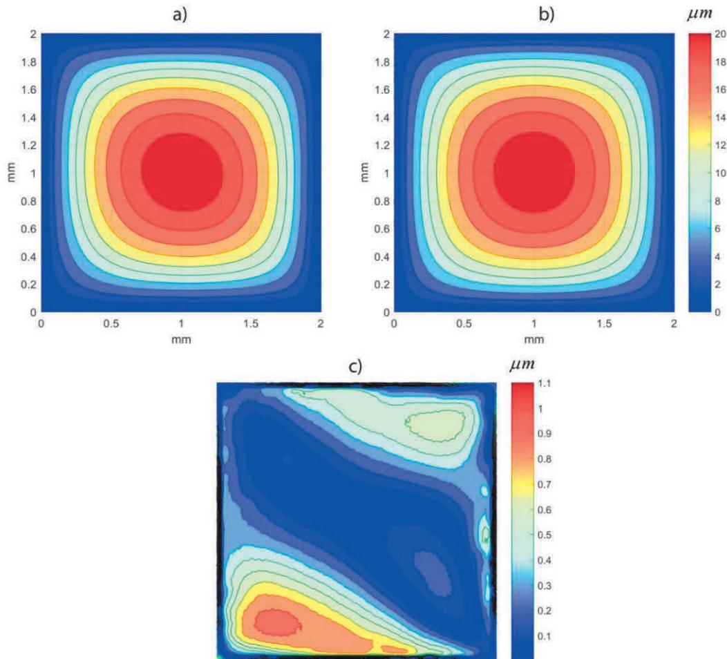
**Figure 6** 3D shape of the membrane, z position is described by color coding. a) Experimental shape of the membrane derived from the interferometric measurement, b) calculated shape of the membrane by FEM, c) difference between the two shapes;  $p = 10\text{kPa}$ .
