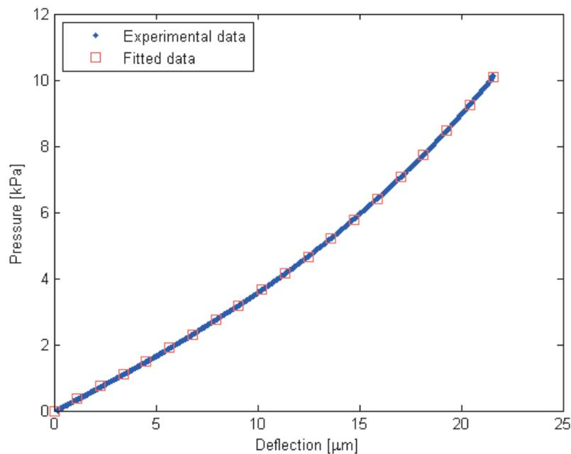
**Figure 5** Pressure - deflection curve for 2x2 mm membrane center and the fit of Eq. 1. Experimental data point are in blue (25000 data points), the fit is represented by red squares.
