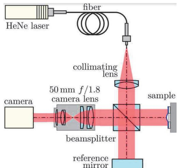
**Figure 2** Schematics of the bulge test apparatus
