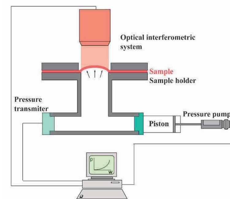
**Figure 3** Interferometer setup
