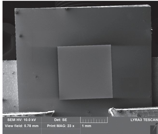
**Figure 1** Si frame with  $\text{Si}_3\text{N}_4$  membrane
