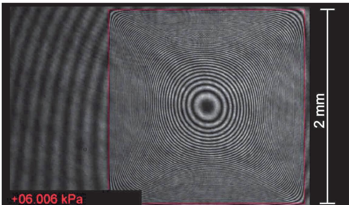
**Figure 4** Interferometric image of the membrane at 6 kPa pressure
