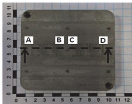
**Figure 2** A precious geometry platform with reducing plates and welded joints (the letters show the sections AB and CD reducing plates used for microstructural analysis)
