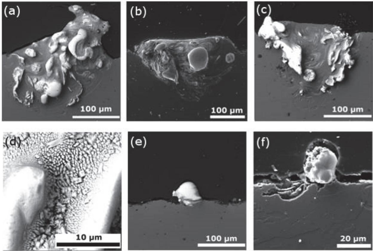
**Figure 4** Microstructure of: (a) welded joint I (SEM-BSE), (b) welded joint II (SEM-SE), (c) welded joint III (SEM-BSE), (d) detail of welded joint III (SEM-BSE), (e) balling phenomenon, area AB (SEM-BSE) and (f) balling phenomenon, area CD (SEM-SE)
