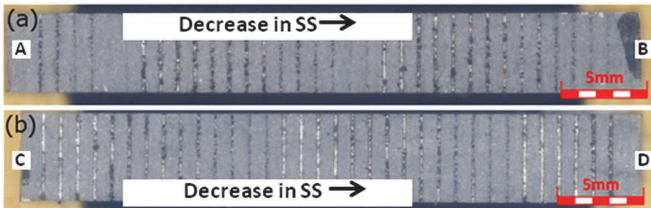
**Figure 3** The appearance of laser tracks in the areas (a) AB and (b) CD
