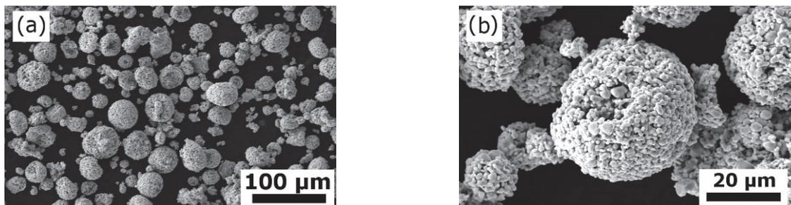
**Figure 1** (a) Morphology of Mo powder, (b) detail of Mo powder, (SEM-SE)
