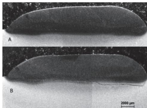
**Figure 3** Sample 3 (A) and 3HT (B) - high speed steel deposit before (A), and after (B) teempering. Crack in HAZ of sample B
