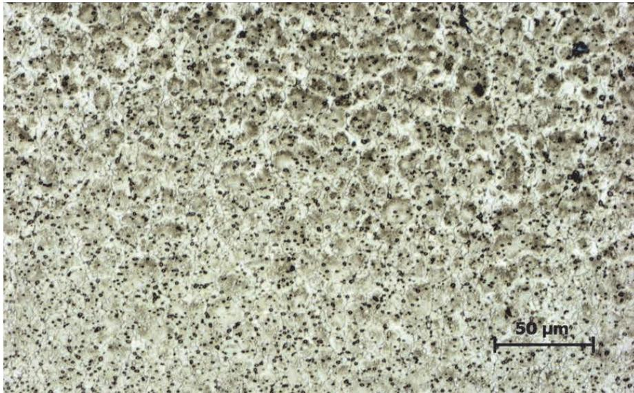
**Figure 4** Sample 2 - transition area between parent material and deposited layer, 100x
