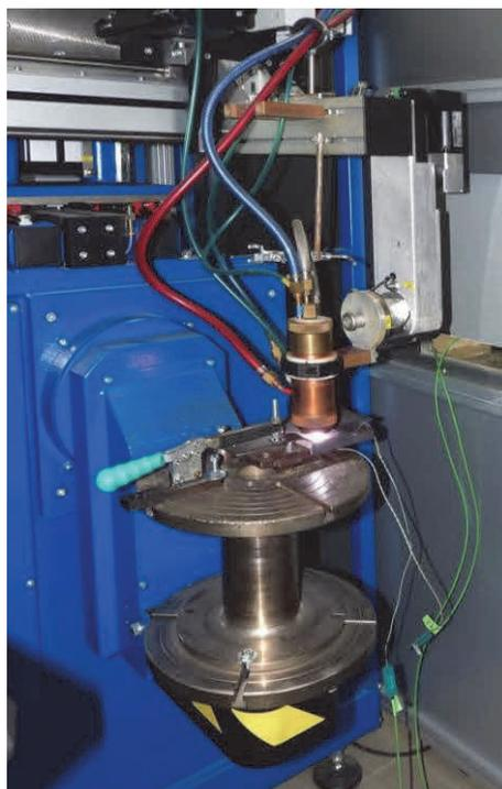
**Figure 1** PTA hardfacing on plasma surfacing automate PPC 250 R6 (KSK, s.r.o., Czech Rep.)
