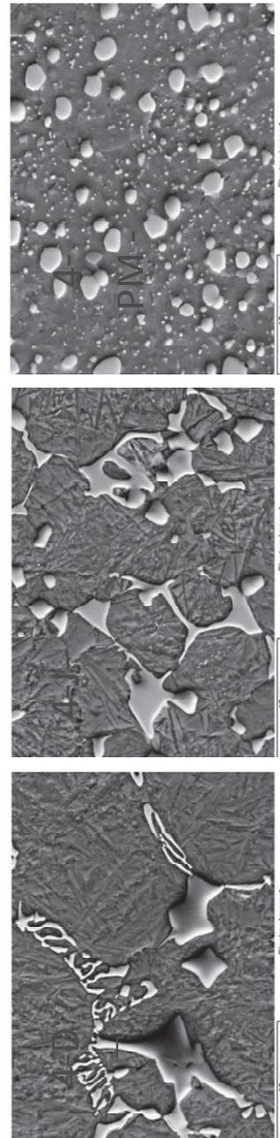
**Figure 7** SEM micrographs of sample 4-HT. 4-D-T - deposit, 4-J-T - deposit/parent material boundary, 4-PM-T - parent material 4000x
