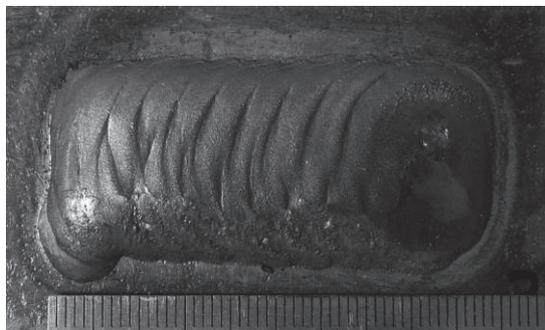
**Figure 2** Deposit of high speed steel on the same grade parent material - pulsed plasma current - 100Hz
