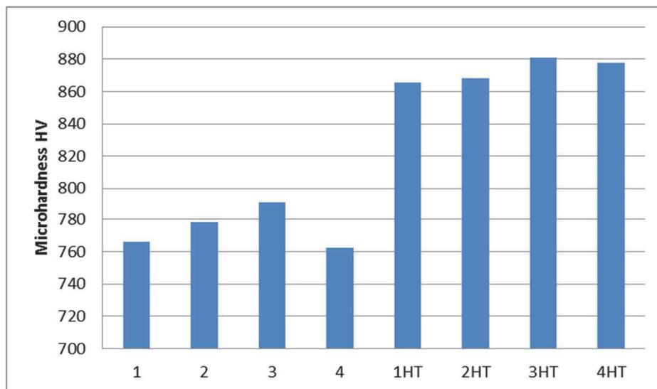
**Figure 5** Microhardness of deposits - 2 mm under free surface
