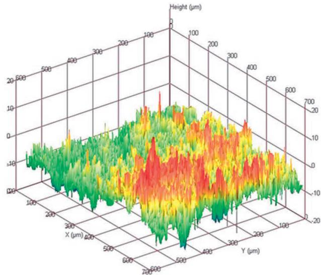
**Figure 4** The comparison of isometric surface image of thermal diffusion coated flat samples before corrosion test - a and after 24 h in salt chamber - b
