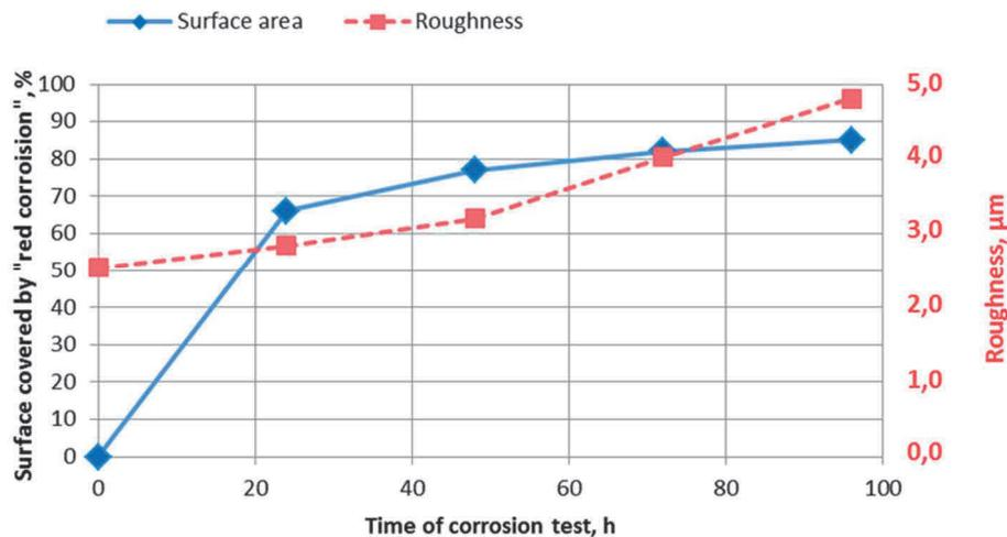
**Figure 3** Kinetics of the corrosion of flat samples after thermal diffusion galvanizing expressed in the percent of the surface occupied by "red corrosion" and roughness changes
