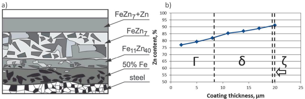
**Figure 5** Theoretical structure observed at the cross section of thermal diffusion coating - a [5] together with zinc distribution at the investigated coating cross section - b
