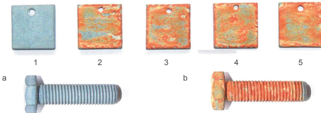
**Figure 2** An appearance of samples investigated in corrosion test: 1 - initial sample, 2 - sample after 24 h, 3 - sample after 48 h, 4 - sample after 72h, 5 - sample after 96 h together with screw M10 before test - a and after 96 h in salt chamber - b.
