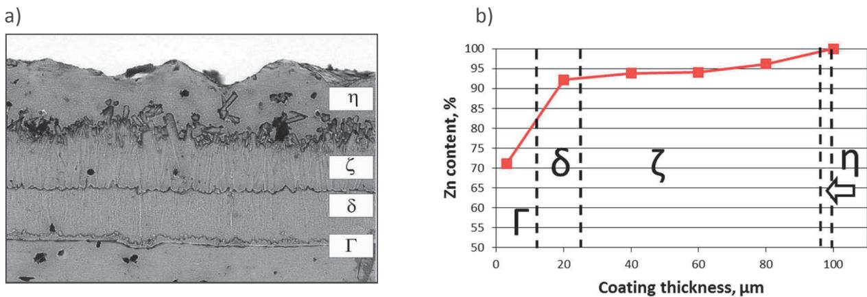
**Figure 6** Theoretical structure observed at the cross section of hot-dip zinc coating - a together with zinc distribution at the investigated coating cross section - b
