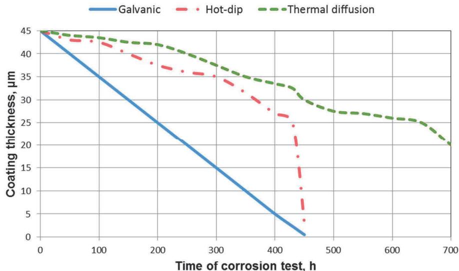
**Figure 1** Comparison of different coatings resistance in neutral salt spray (NSS) [9]
