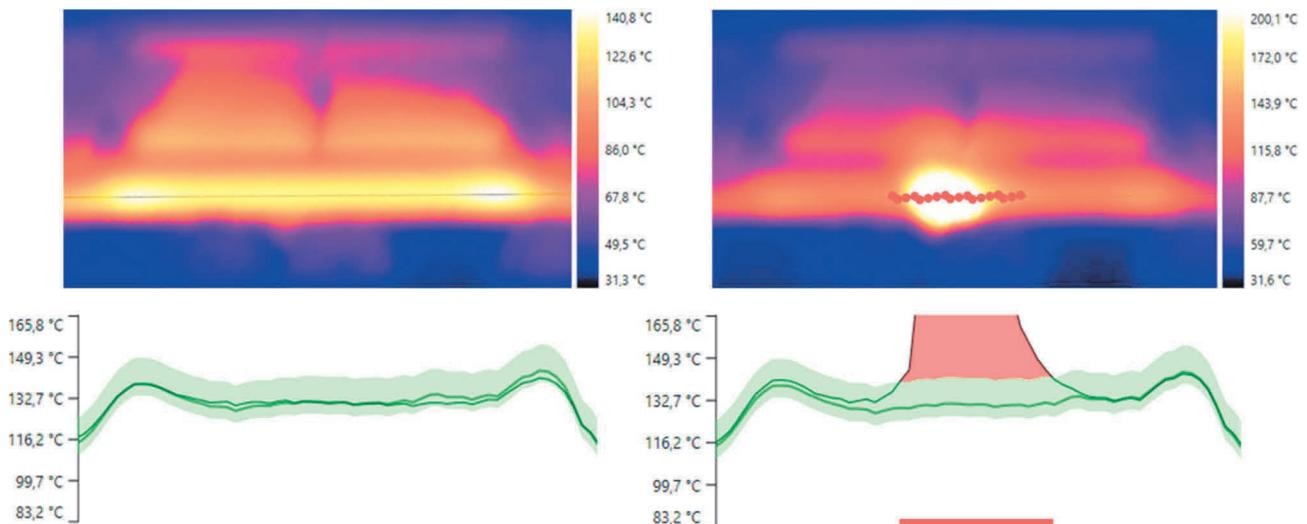
**Figure 2** Thermography plastics laser welds inspection demonstration. Left: correctly welded parts. Right: A weld with an overheated area - red points show the weld parts with too high temperature.
