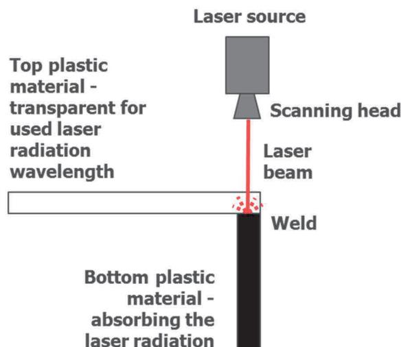
**Figure 1** Schematic representation of laser plastics welding principle.
