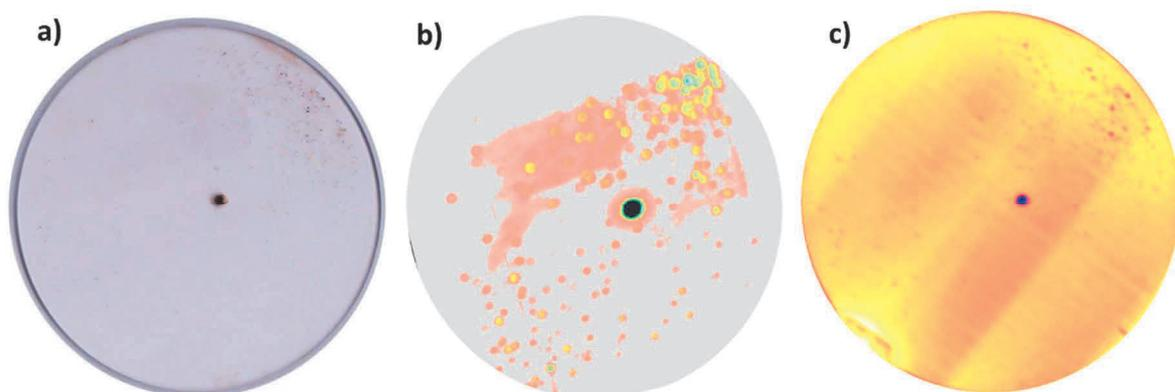
**Figure 3** Example of an evaluation of laser scanning head protection glass contamination: a) optical scanner record, b) laser thermography inspection, c) flash-pulse thermography inspection
